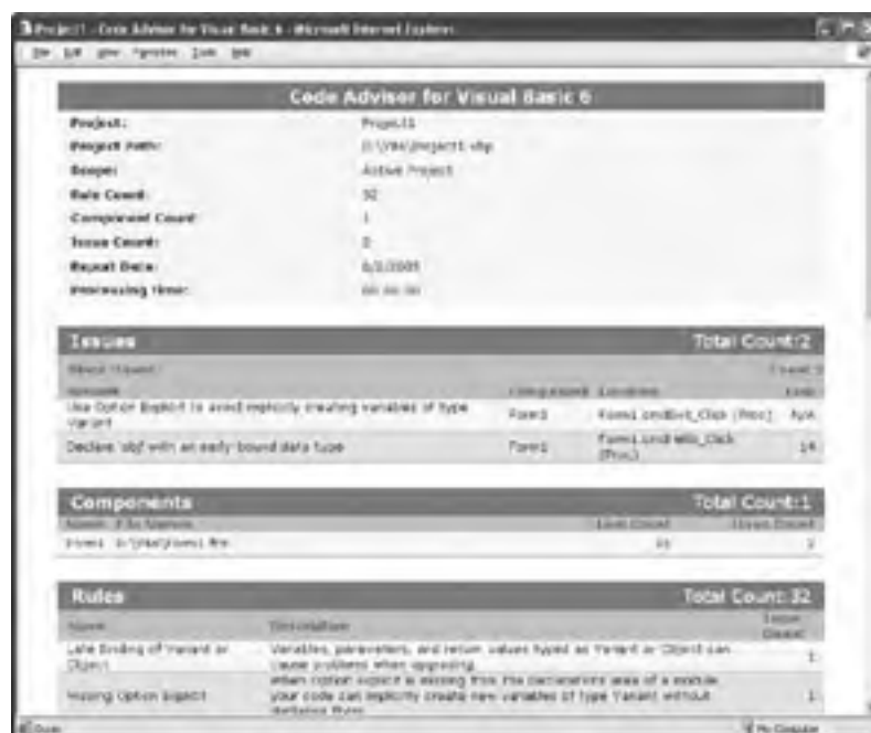
Figure 6-10. Viewing the FixIts report
