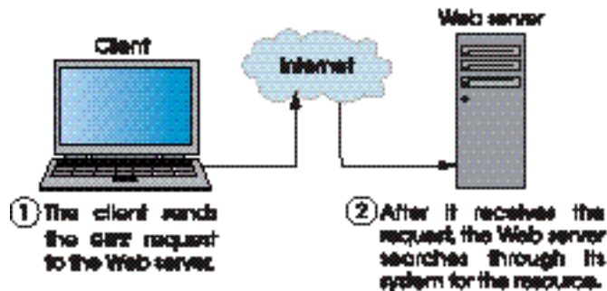
Fig. 20.1 Client interacting with Web server. Step 1: The GET request, GET /books/downloads.htm HTTP/1.1 .
