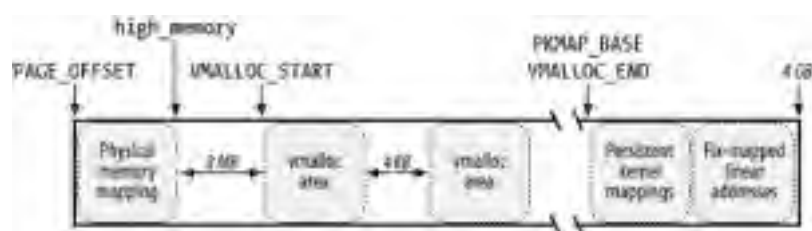
Figure 7-7. The linear address interval starting from PAGE_OFFSET
