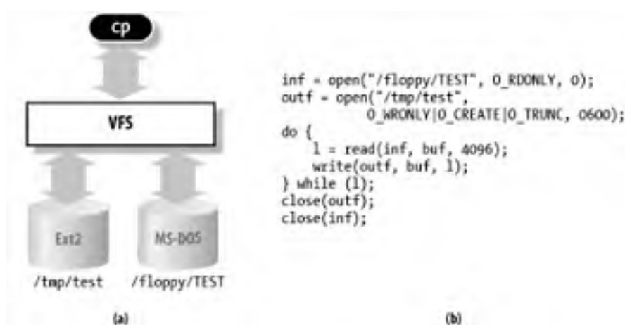
Figure 12-1. VFS role in a simple file copy operation
