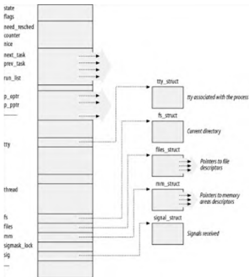
Figure 3-1. The Linux process descriptor
