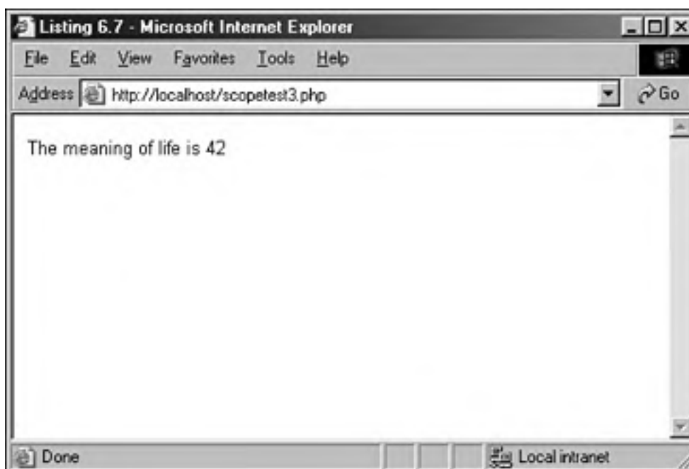
Figure 6.5. Successfully accessing a global variable from within a function using the global keyword.
