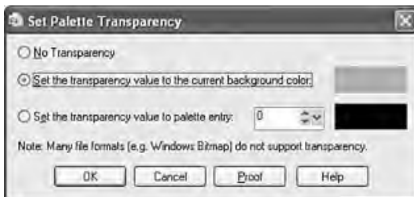
Figure 9.5. This dialog box appears when you select Image, Palette, Set Palette Transparency. You will usually want the middle option.
