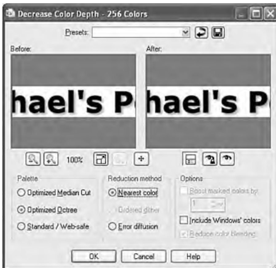
Figure 7.10. Reducing the number of colors in an image can dramatically decrease file size without noticeably changing the appearance of the image.
