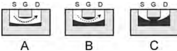
23-3 At A, the depletion region (darkest area) is narrow, the channel (white area) is wide, and many charge carriers (heavy dashed line) flow. At B, the depletion region is wider, the channel is narrower, and fewer charge carriers flow. At C, the depletion region obstructs the channel, and no charge carriers flow.
