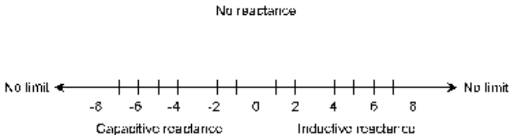
14-1 Inductive and capacitive reactance can be represented as numerical values (corresponding to ohms multiplied by j ) along a number line.
