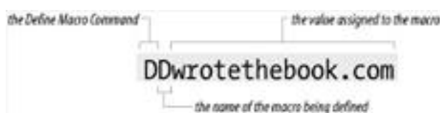
Figure 10-2. A sendmail.cf configuration command
