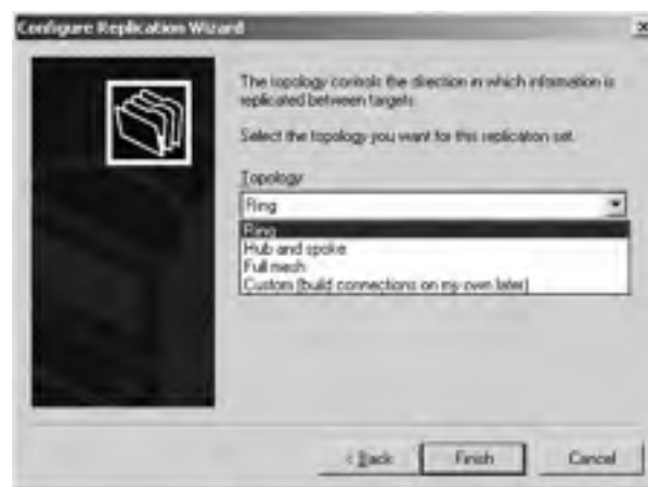
FIGURE 14.24 Selecting a topology to replicate DFS replicas
