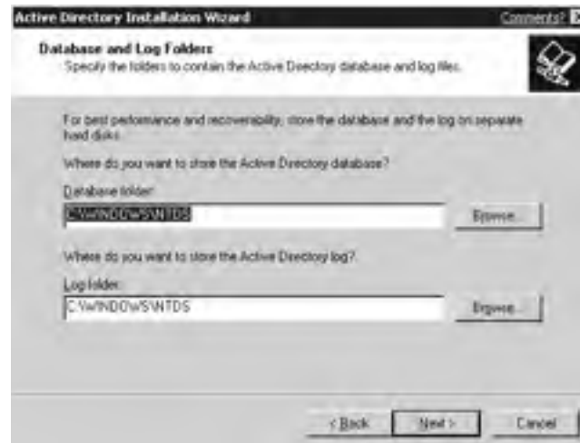
FIGURE 9.7 Storing the database and log files
