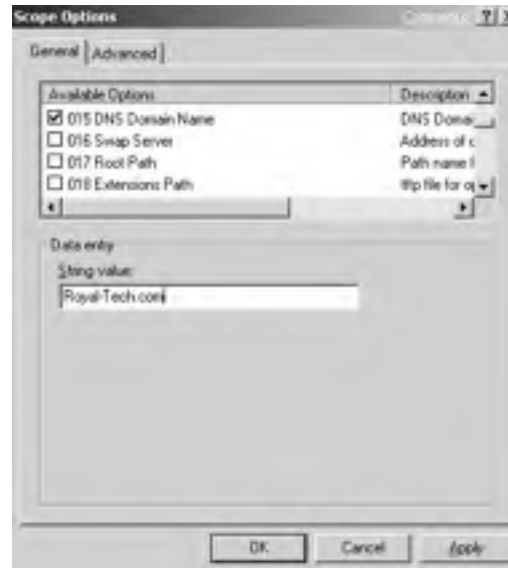
FIGURE 7.28 Configuring the DNS Domain Name option
