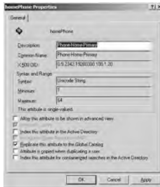
FIGURE 14.2 Viewing Global Catalog attributes with the Schema Master MMC
