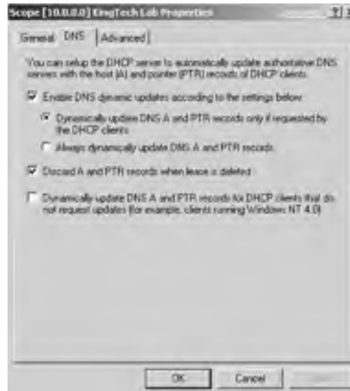
FIGURE 7.29 Enabling DHCP to manage DNS host records
