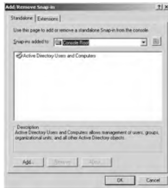
FIGURE 11.2 The Add/Remove Snap-in dialog box
