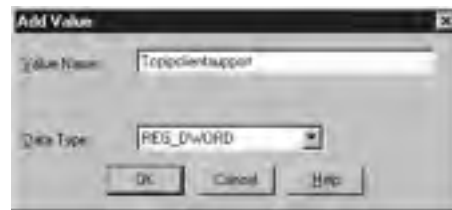
FIGURE 17.10 Adding the Value Name and Data Type to the Registry
