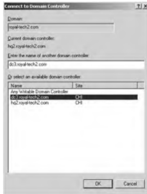
FIGURE 14.30 Selecting a domain controller for transfer
