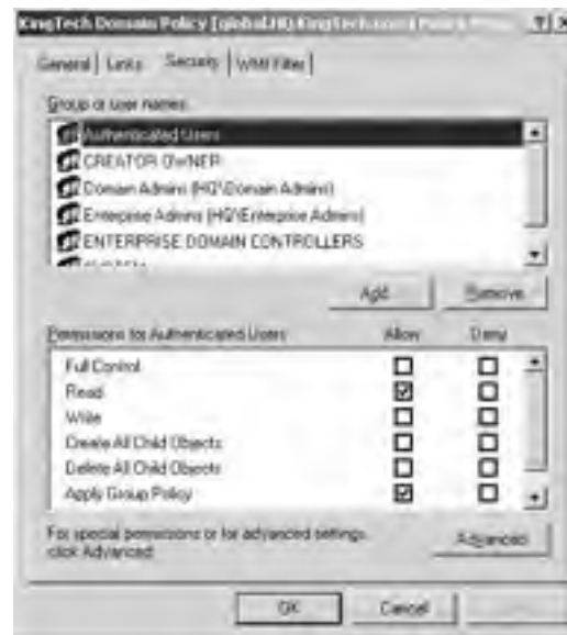
FIGURE 11.38 Security tab of the GPO Properties dialog box
