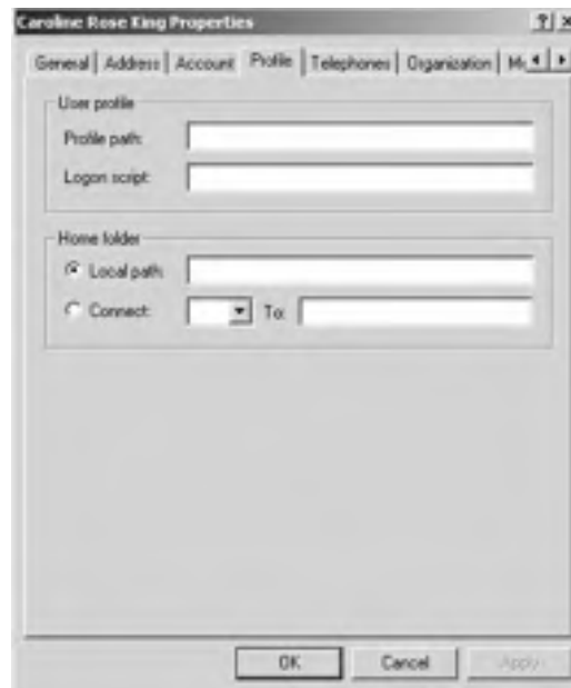
FIGURE 9.44 The Profile tab of the User Properties window
