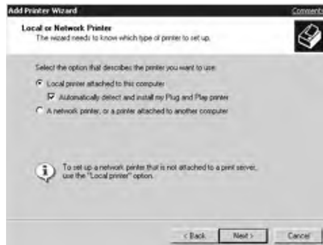
FIGURE 9.64 Installing a local or network printer
