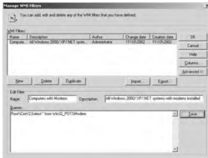
FIGURE 11.42 The Manage WMI Filters dialog box
