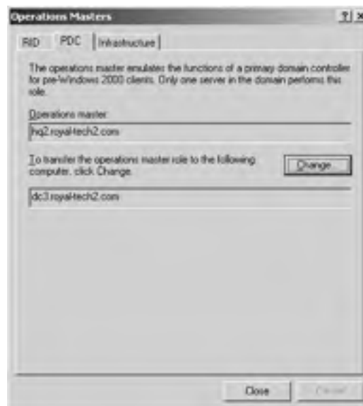
FIGURE 14.31 Transferring a PDC Master
