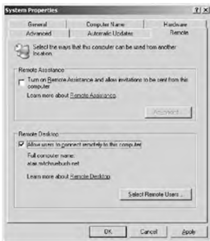
Figure 10.2: Enabling Remote Desktop for Administration
