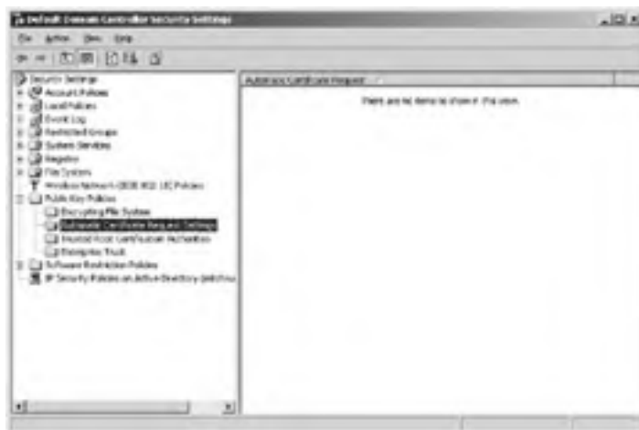
Figure 6.14: The automatic certificate request settings in the Group Policy Editor
