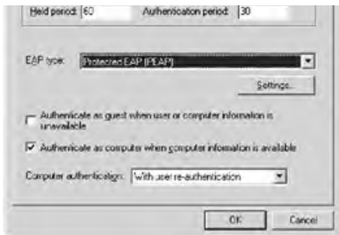
Figure 3.15: Enabling PEAP on Windows Server 2003
