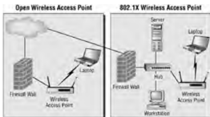
Figure 3.16: Network layout with an open access point
