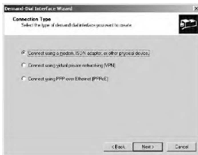
Figure 3.8: Various demand-dial connection types that can be used for the demand-dial interface
