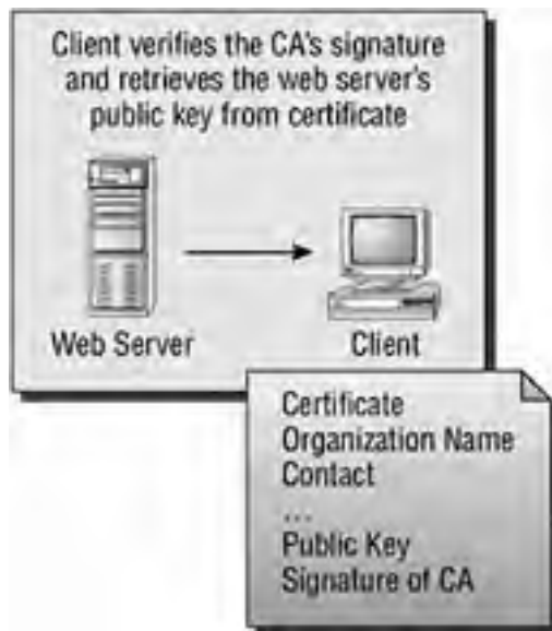
Figure 6.8: Client verifies certificate signature and uses public key to encrypt response.
