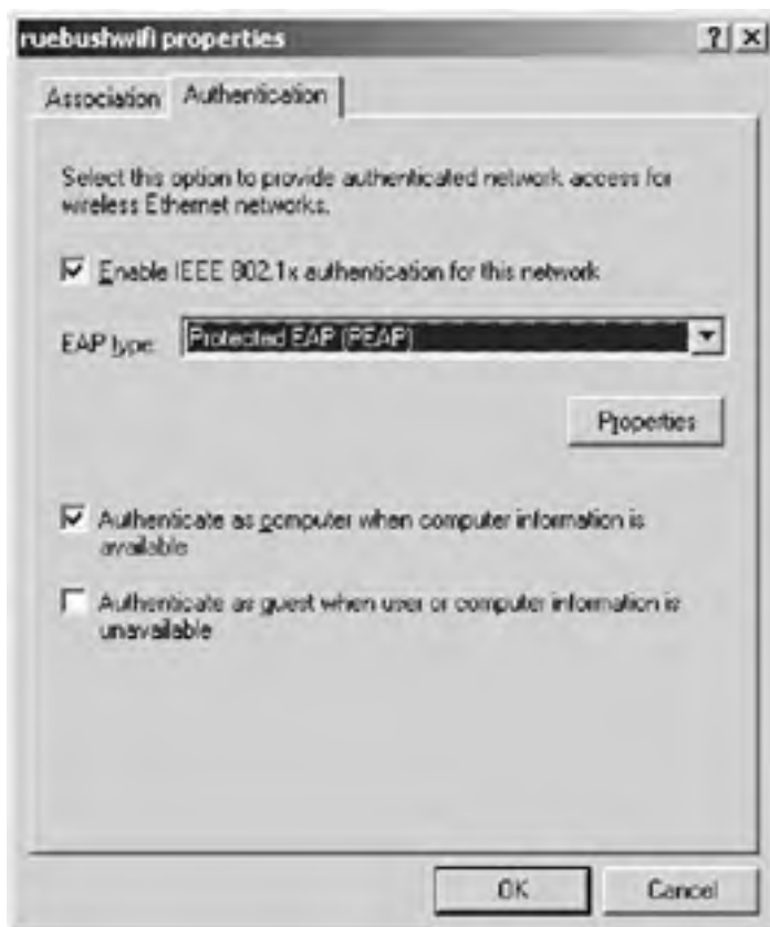
Figure 3.14: Enabling PEAP for 802.1x authentication
