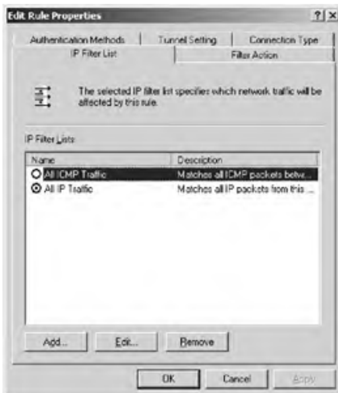
Figure 3.4: Creating IPSec rules on Windows Server 2003
