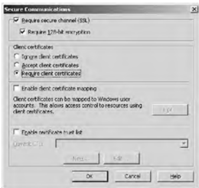
Figure 7.4: Requiring client certificates to access the website
