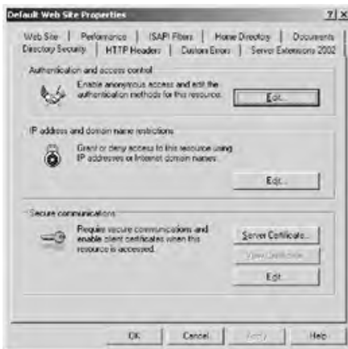
Figure 3.5: Filtering IP addresses using the IP Address And Domain Name Restrictions dialog box
