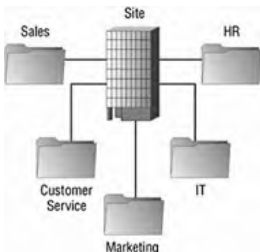
Figure 9.3: OU Model with security groups for computer function.
