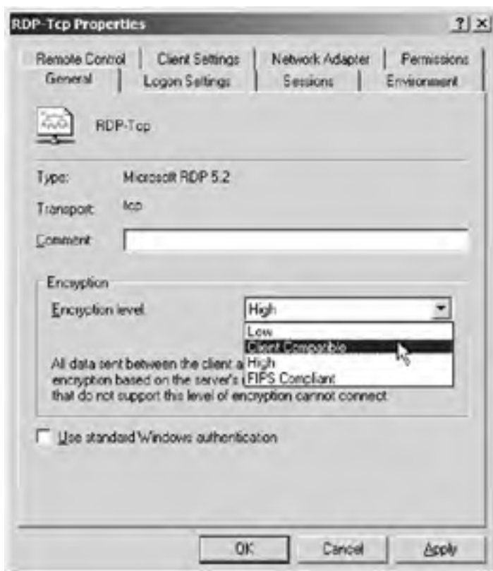
Figure 10.4: Setting the encryption level for the RDP protocol
