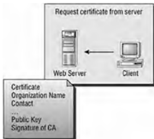
Figure 6.7: Client requesting certificate from the server
