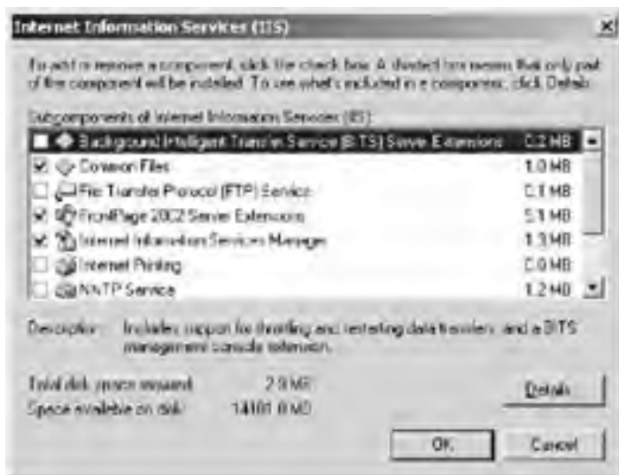
Figure 7.1: Selecting the IIS services to install through Windows Component Wizard's Internet Information Services (IIS) dialog box
