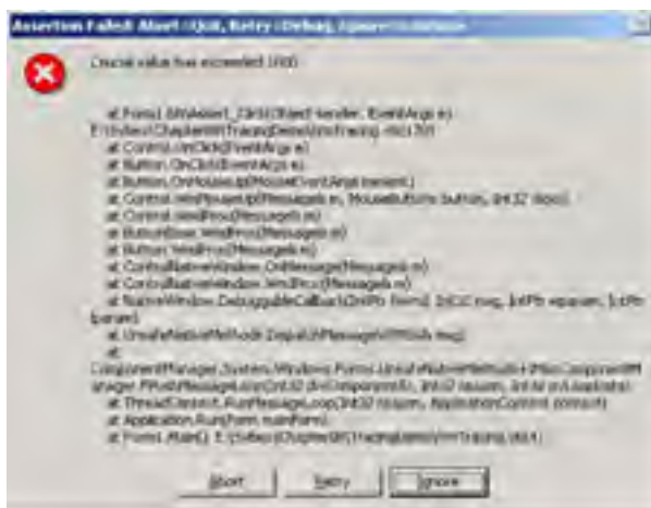
Figure 8.7: The message box that is displayed when an Assert method call fails
