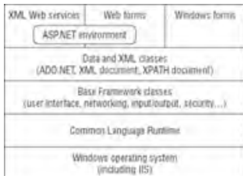
Figure 9.1: Diagram of OS/CLR/.NET Framework classes
