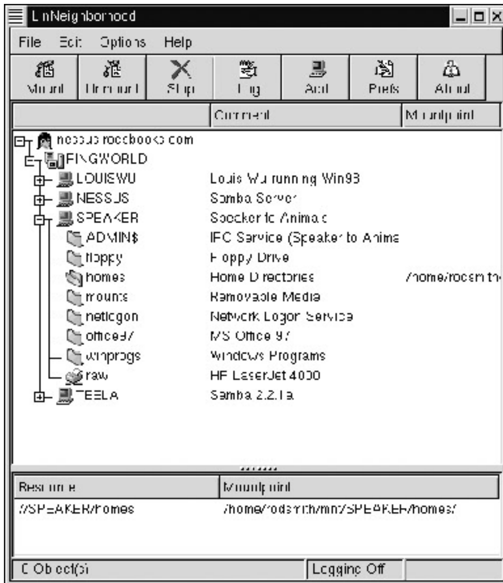
Figure 12.4: LinNeighborhood and other GUI SMB/CIFS browsers provide a user interface similar to that of Network Neighborhood in Windows.
