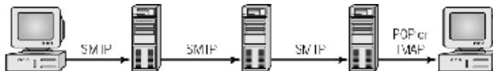
Figure 14.1: E-mail frequently passes through several computers between its source and its destination.
