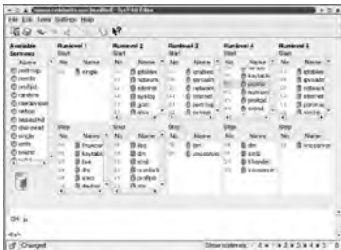
Figure 22.4: The ksysv runlevel configuration tool enables you to drag and drop services between runlevels.
