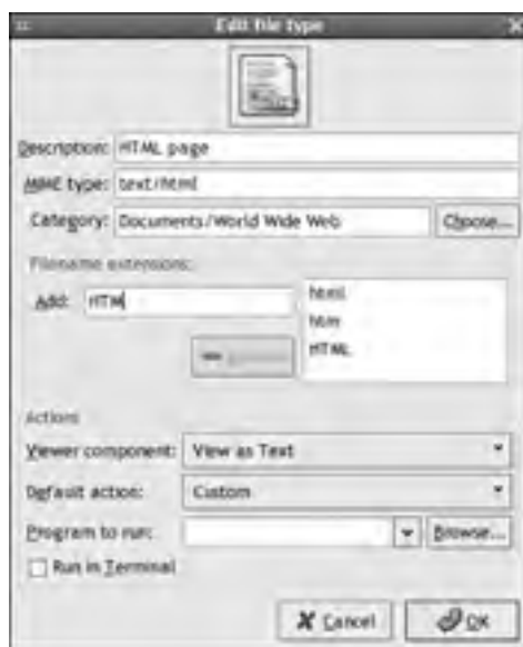
Figure 6.9: You can modify MIME types using the Edit File Type dialog box.
