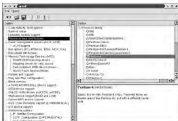
Figure 1.1: The Linux kernel provides many options related to the CPU.
