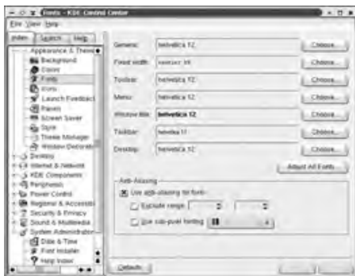
Figure 16.3: KDE provides tools to enable font smoothing for KDE applications.
