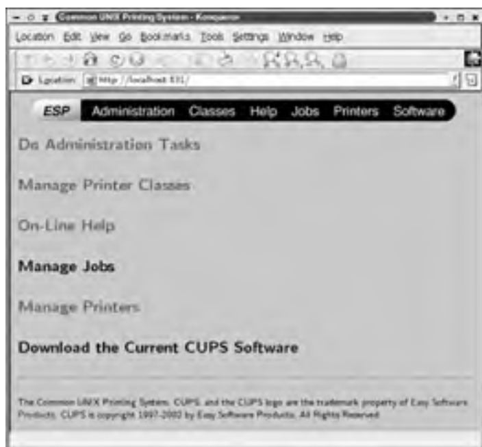
Figure 13.1: CUPS provides a web-based tool for managing printers.
