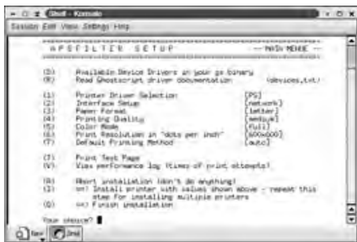
Figure 13.2: The main Apsfilter Setup screen lets you change various printer options.
