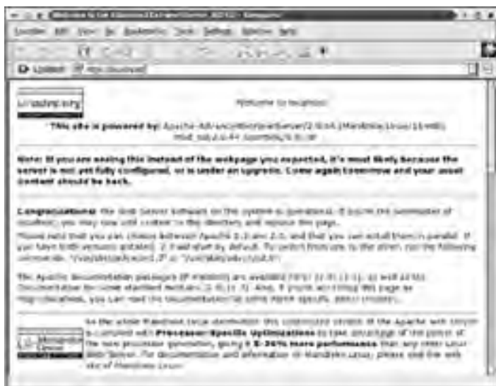
Figure 23.1: Once installed and run, a default Apache configuration displays a generic Apache web page or a page for your distribution.
