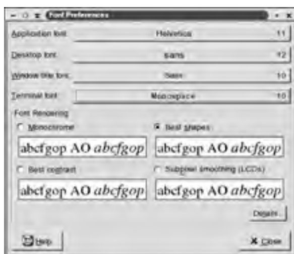
Figure 16.4: GNOME's Font Preferences dialog box enables you to select GNOME fonts and set font-smoothing options.
