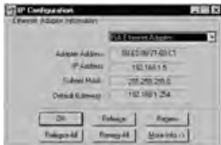
Figure 27.2: Windows 9x/Me provides a GUI tool for displaying the MAC address and other network information.
