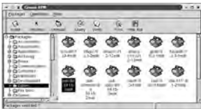
Figure 11.1: GUI RPM Tools enable you to browse and manipulate installed and uninstalled packages in a point-and-click environment.
