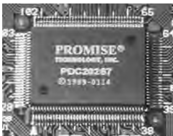
Figure 1.2: Device chips are often marked to identify the chipset.
