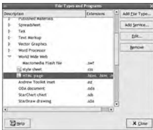
Figure 6.8: The File Types and Programs tool enables you to edit GNOME's file type associations.
