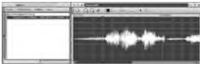
Figure 8.1: GUI sound editors let you modify sounds using visual representations of the audio waveform.
