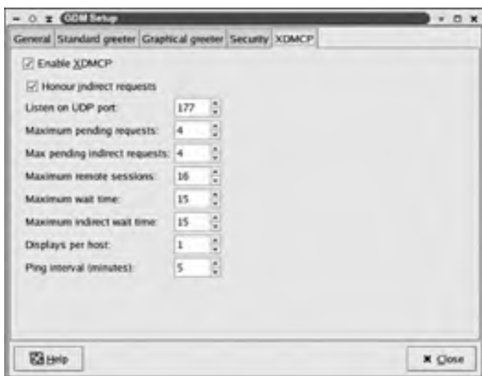
Figure 26.2: GDM provides a GUI configuration tool in which you can activate XDMCP options.
