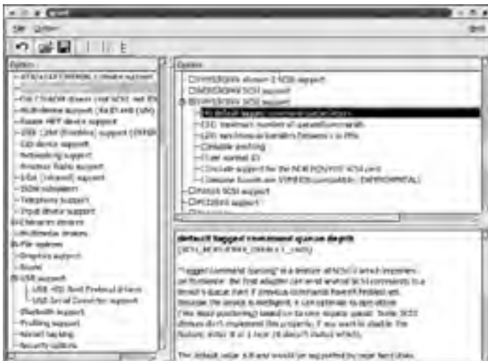
Figure 15.4: Some kernel options provide associated sub-options that fine-tune the driver's behavior.
