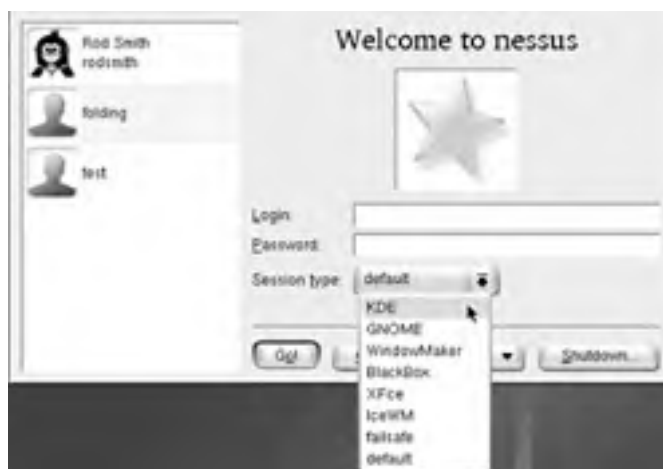
Figure 6.1: GUI login managers usually provide a selection of environments from which you can choose what to run.
