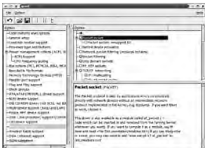
Figure 27.1: You must enable certain kernel options to run a recent DHCP server.
