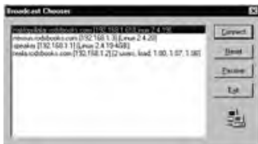
Figure 26.4: XDMCP clients frequently enable you to pick which XDMCP server to use from a list.
