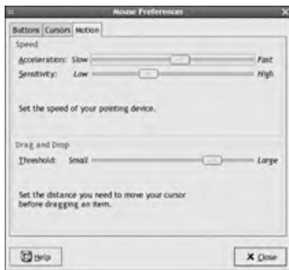
Figure 6.11: The Mouse Preferences dialog box provides tools for adjusting mouse behavior.
