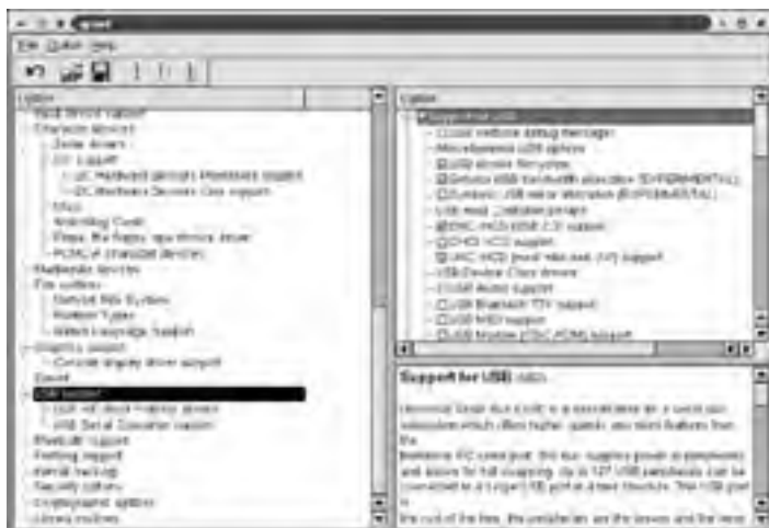
Figure 3.2: The Linux kernel provides a large number of USB driver options.
