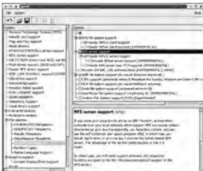
Figure 24.1: The Linux kernel provides NFS support options in its configuration tool.
