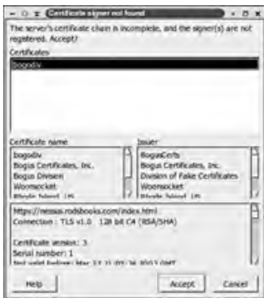
Figure 23.2: Secure HTTP provides authentication and warnings when a server's identity can't be verified.
