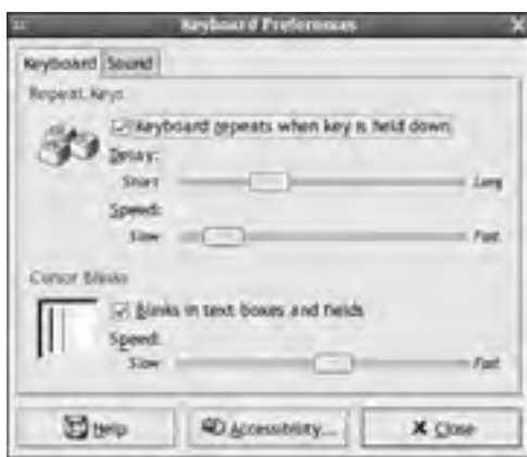
Figure 6.12: The Keyboard Preferences dialog box controls the keyboard repeat rate and other keyboard and text-entry options.
