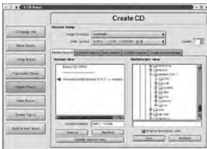
Figure 2.2: X-CD-Roast provides GUI tools for specifying what files to include on a CD-R.
