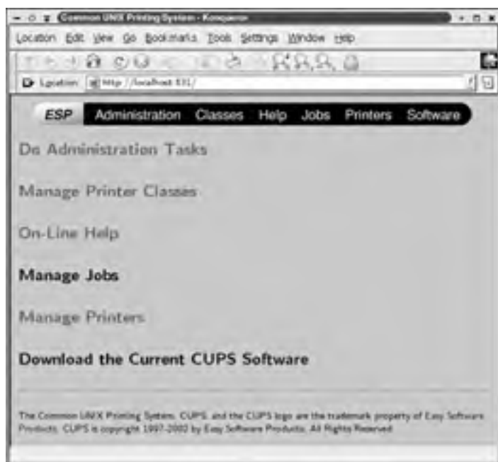
Figure 13.1: CUPS provides a web-based tool for managing printers.
