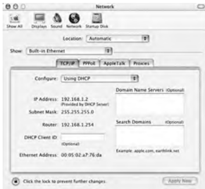
Figure 27.3: Mac OS X calls the MAC address the Ethernet Address in its GUI configuration tool.
