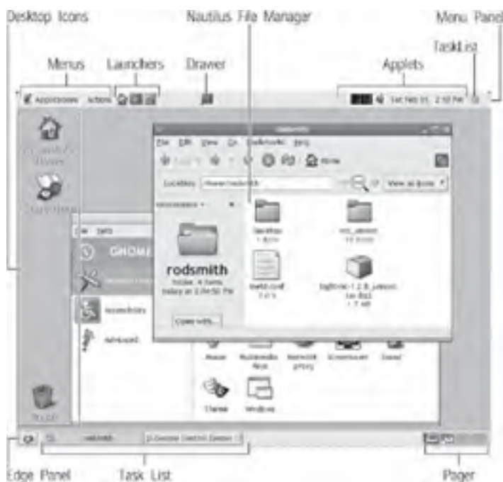
Figure 6.7: The GNOME desktop provides all the familiar features of modern computer desktop environments.
