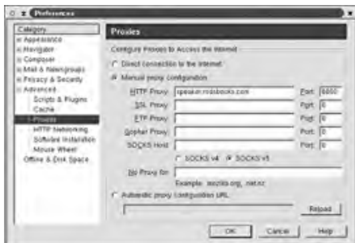
Figure 8.9: All major web browsers enable you to specify one or more proxy servers to use instead of direct access.
