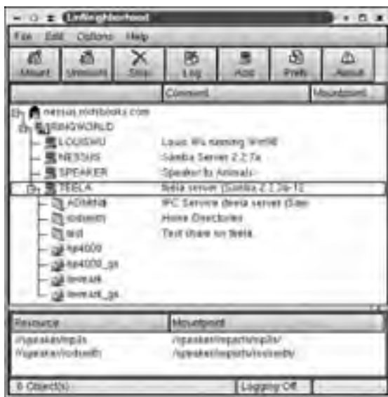
Figure 24.3: GUI SMB/CIFS browsers such as LinNeighborhood enable you to browse the contents of a Windows network.
