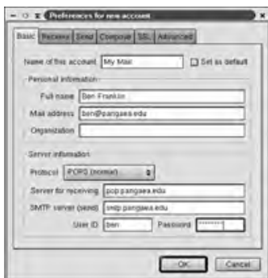
Figure 8.11: You must tell your mail reader how to send and receive mail.
