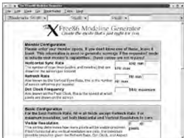
Figure 16.6: The XFree86 Modeline Generator page performs the tedious calculations required to create a custom video mode.
