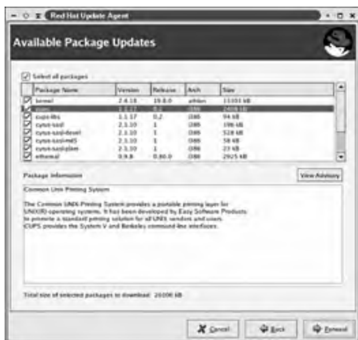
Figure 11.3: Red Hat's Update Agent presents a list of packages for which updates are available.
