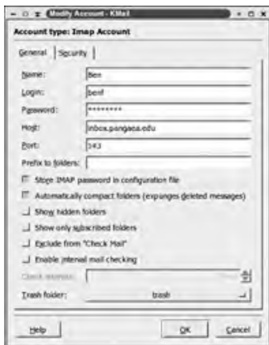
Figure 25.2: Mail clients must be told where to find a POP or IMAP server.
