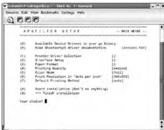
Figure 8.2: The main Apsfilter menu provides options for creating and modifying printer queues.
