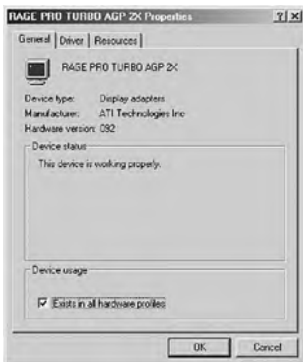
Figure 2.15: The Windows Properties dialog box for the video card may provide information on the video chipset manufacturer.
