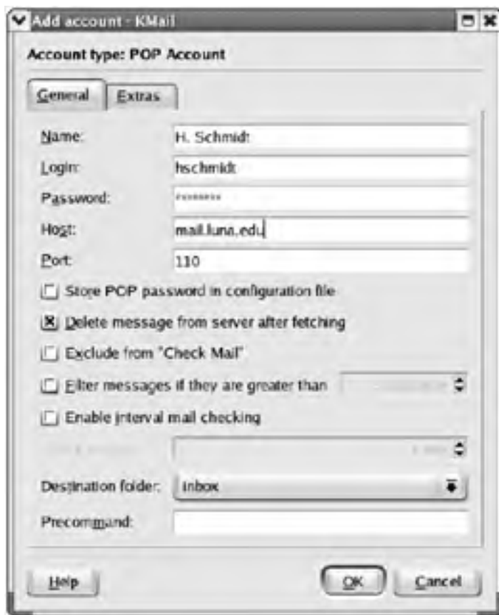
Figure 5.8: An e-mail client using a pull mail protocol employs your account on a mail server to retrieve e-mail.
