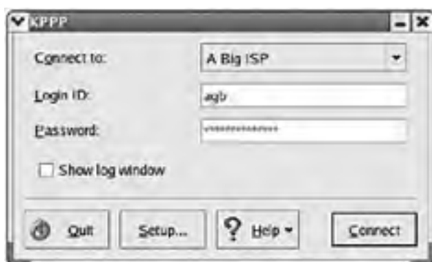
Figure 5.5: GUI dialers enable you to select from among several ISPs or dial-up numbers and connect by clicking a button.
