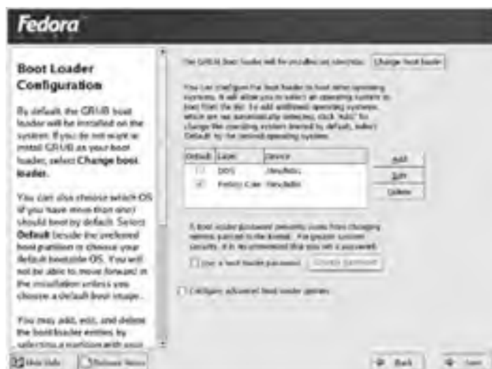
Figure 2.6: You must provide a few key pieces of information about how you intend to boot the computer.
