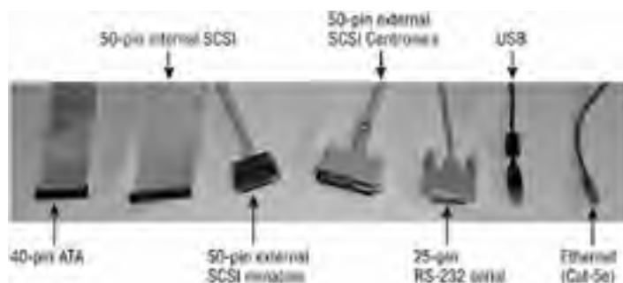
Figure 1.3: Internal and external cables come in a wide variety of shapes and sizes, although some resemble each other.
