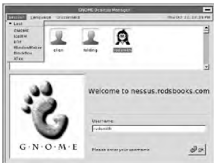
Figure 2.20: The GDM and KDM programs both provide users with a way to select the login environment.
