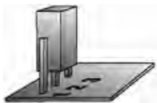
Figure 8.9: Jumpers allow you to adjust key aspects of hardware operation, particularly on older hardware.
