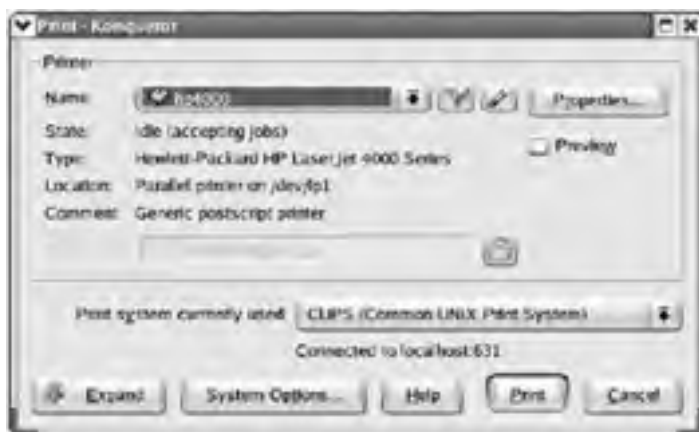
Figure 8.6: Most Linux programs that can print do so by using lpr , but many hide the details of the lpr command behind a dialog box.
