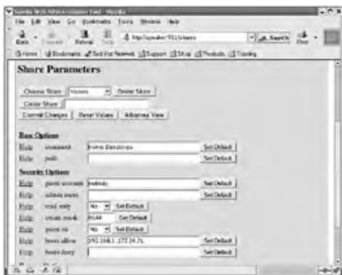
Figure 5.11: SWAT enables you to administer Samba using a Web browser's point-and-click tools.
