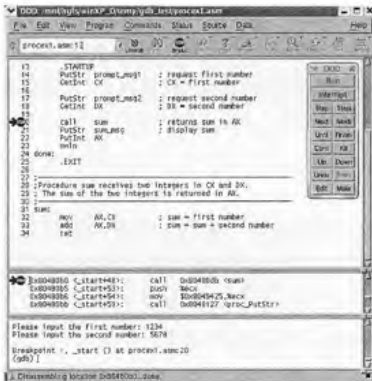
Figure 8.2 DDD window at the breakpoint on line 20. This screenshot also shows the machine code window and the source code line numbers.
