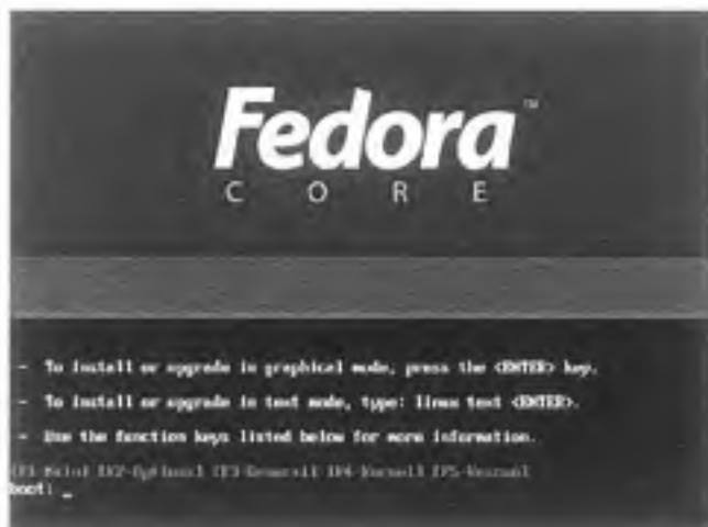
Figure 5.1 Fedora Core 3 initial screenshot. Type linux rescue to access the parted utility to partition your hard disk.
