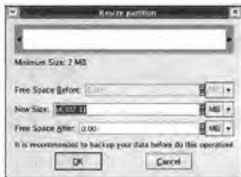
Figure 5.3 When the resize operation is selected, this pop-up window allows us specify the new partition size.
