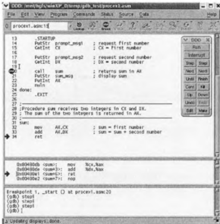
Figure 8.5 DDD window after single stepping from the breakpoint on line 20.
