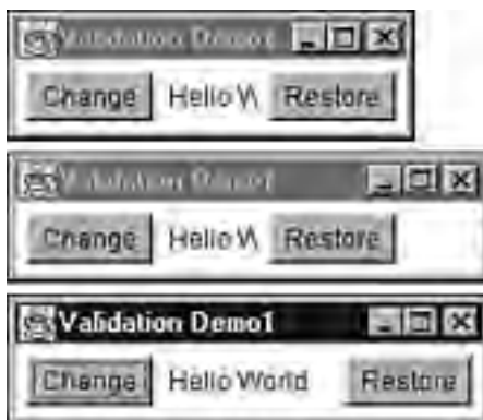
Figure 16.27. ValidationDemo1's GUI is shown when no arguments (top), an S argument, and a V argument (bottom) are specified.
