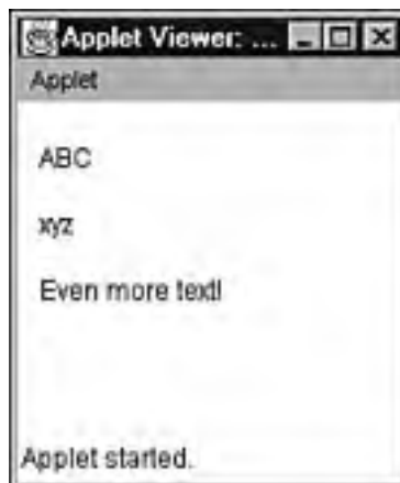
Figure 13.2. The DrawTextDemo applet shows text displayed using a graphics context's text drawing methods.
