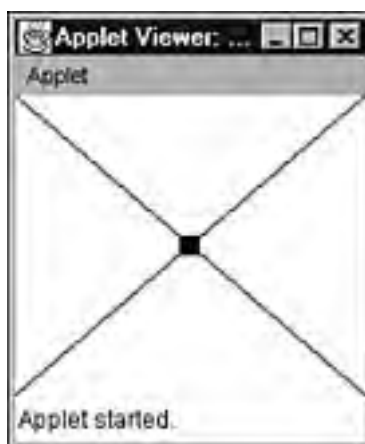
Figure 13.3. The DrawLinePointDemo applet shows lines and points displayed using a graphics context's drawLine method.
