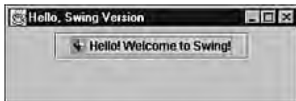
Figure 15.2. Like AWTHello , SwingHello 's GUI consists of a button initialized to default text.
