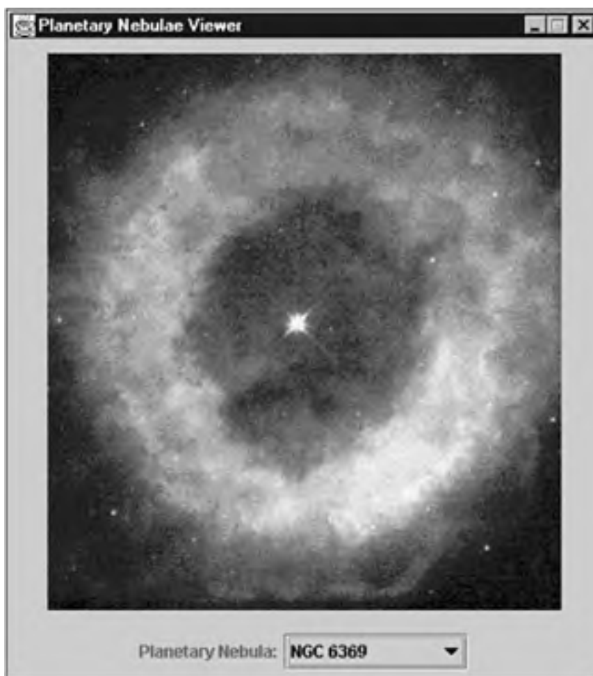
Figure 12.2. The PNViewer2 application presents a Swing GUI consisting of an image (displayed in a JLabel component) and a JComboBox component.
