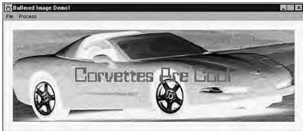
Figure 18.27. An inverted image results from swapping color numbers with their extreme opposites.
