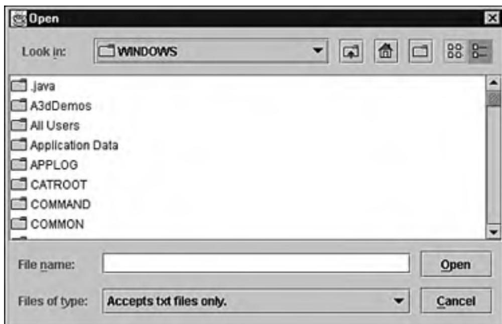
Figure 16.12. Swing's file chooser is configured to serve as an Open dialog box. It can also be configured to serve as a Save dialog box.
