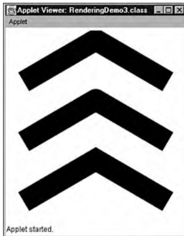
Figure 18.4. A basic stroke's join styles include bevel (top), round (middle), and miter (bottom).
