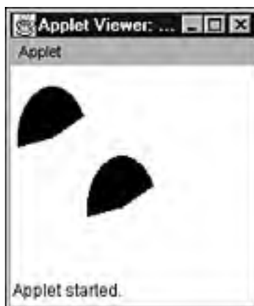
Figure 13.12. The CopyDemo applet shows the results of using a graphics context's copyArea method.
