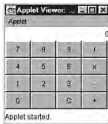
Figure 14.20. Layout managers can be combined to achieve an appropriate layout for a calculator GUI.
