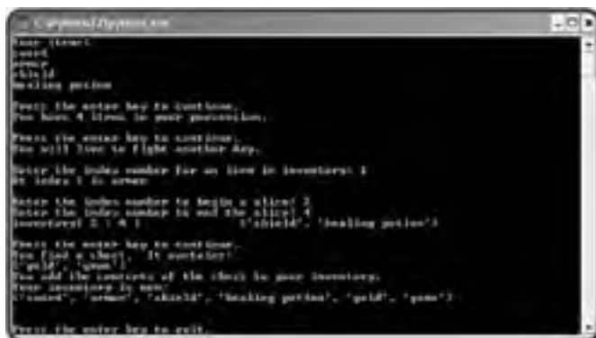
Figure 4.12: The hero's inventory is a tuple, which means it can be counted, indexed, sliced, and even concatenated with another tuple.
