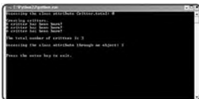
Figure 8.7: Critters are being born left and right! The program keeps track of all of them through a single, class attribute, which it displays through a static method.
