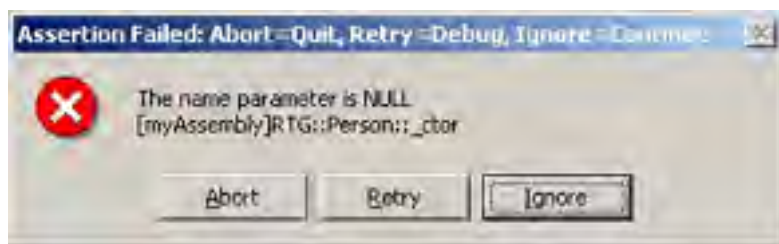
Figure 7-1. Assertion dialog box generated by DefaultTraceListener when AssertUiEnabled is set to true
