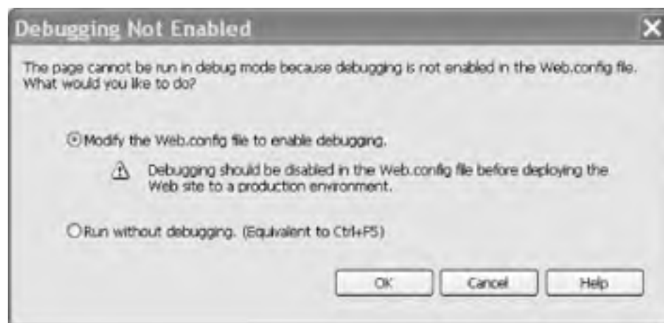
Figure 15-5. You'll see this if you start debugging before you have a Web.config file
