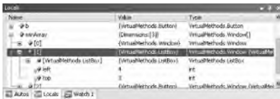
Figure 2-9. Locals window object expanded
