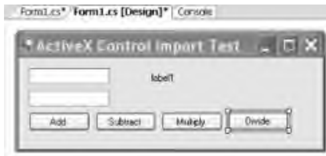
Figure 22-5. Building a Windows Form to test the CalcControl ActiveX control
