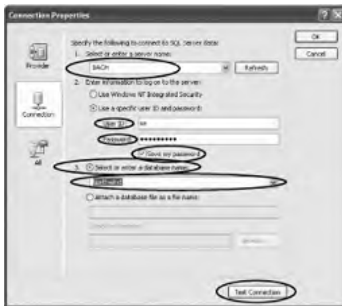
Figure 15-10. Setting the connection properties
