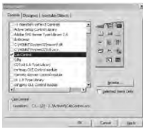
Figure 22-2. Adding the CalcControl to the VB6 toolbox
