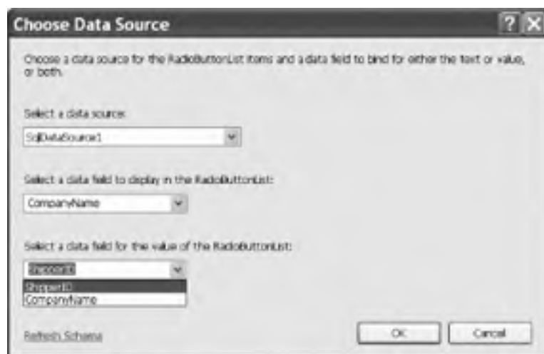
Figure 15-13. Binding fields to the radio button control
