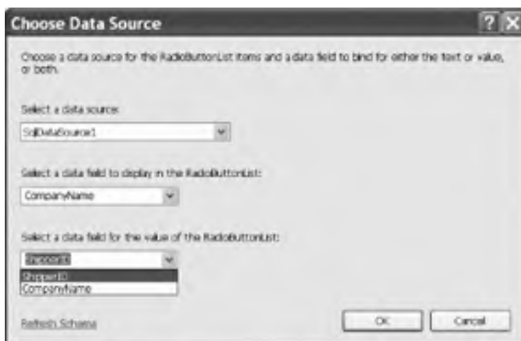
Figure 15-13. Binding fields to the radio button control
