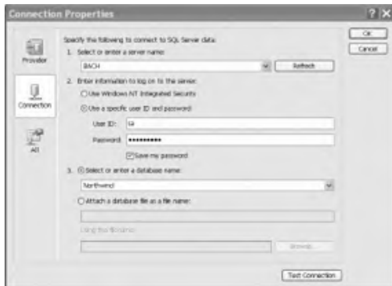
Figure 14-5. Setting the connection properties
