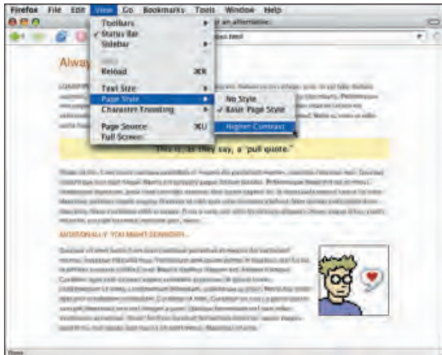
Figure 5-4: By changing the rel attribute of the second link element to "alternate stylesheet" and supplying a title, you implement some basic style switching.
