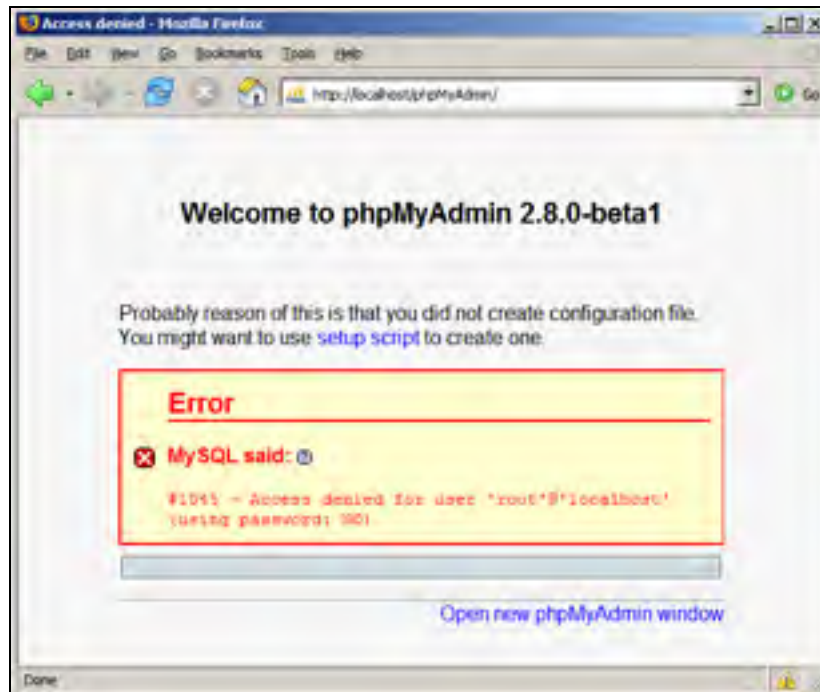
Figure A.4: phpMyAdmin Doesn't Have Access to MySQL
