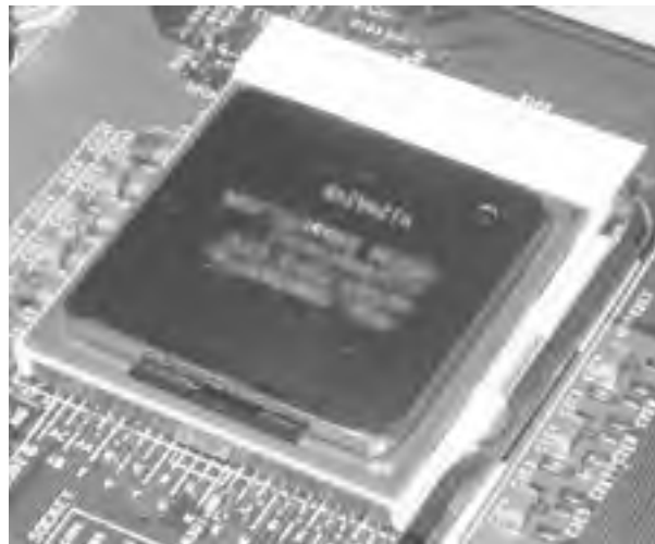
Figure 28-14. With the processor fully seated, lower the ZIF socket arm until it snaps into place parallel to the motherboard and is secured by the plastic latch
