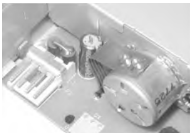
Figure 6-1. All 3.5" FDDs use this unshrouded 4-pin power connector (labeled P2 here)
