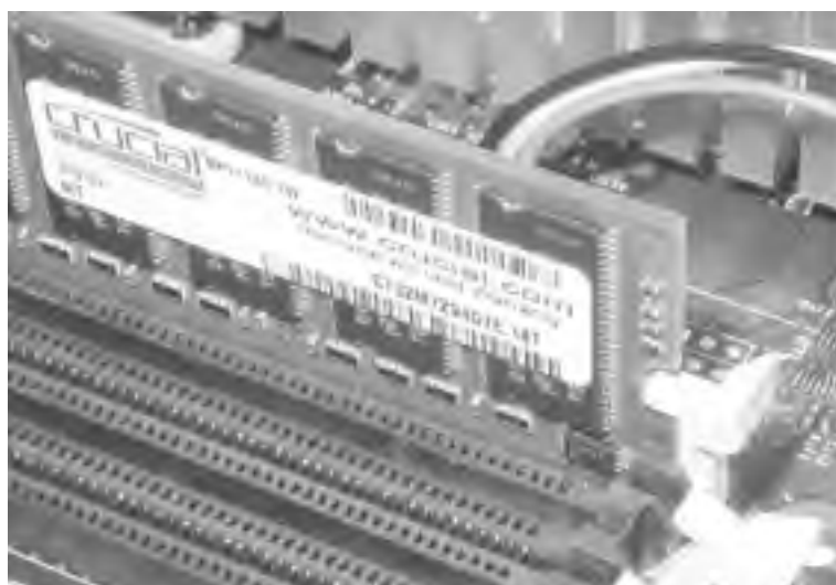
Figure 5-7. When the memory module is fully seated, the ejector arms pivot back to the vertical
