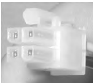
Figure 28-34. The ATX12V Supplementary Power Connector snaps into place
