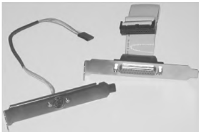
Figure 28-36. Typical port extenders for an AT motherboard
