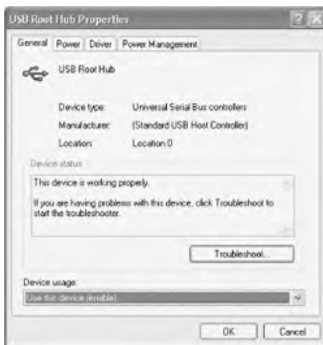
Figure 24-11. The Windows XP Root Hub Properties dialog displays detailed root hub information
