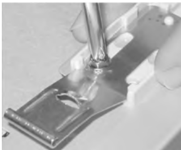
Figure 28-24. Secure the drive rails to the drive, making sure that the drive is electrically grounded to the chassis
