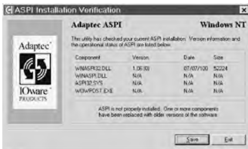
Figure 11-8. The ASPI check program showing that an early version (1.06) of ASPI is installed, and pointing out that the software is not properly installed
