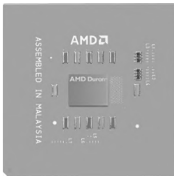
Figure 4-13. AMD Duron processor (image courtesy of Advanced Micro Devices, Inc.)
