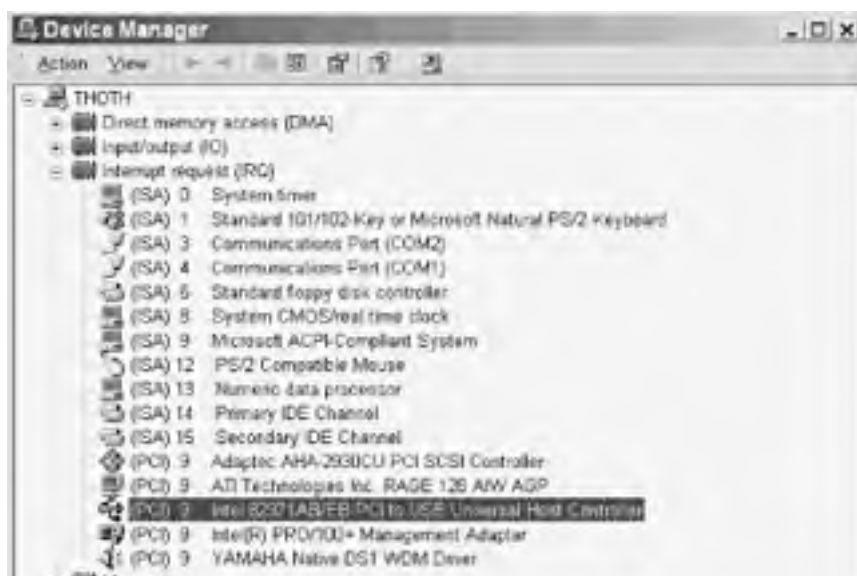
Figure 24-13. Windows 2000 Device Manager shows this system shares one interrupt among the USB HCI and four other devices
