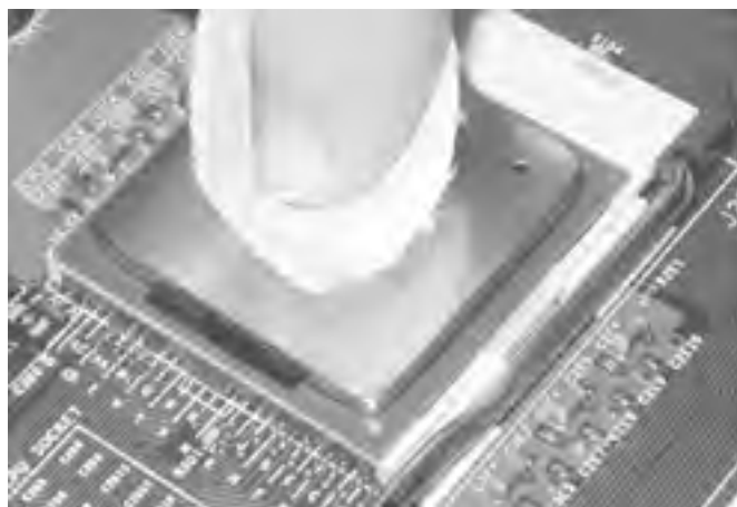
Figure 28-15. Polish the processor carefully before applying thermal compound
