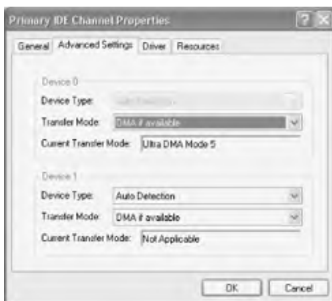
Figure 14-3. Windows XP shows that UDMA-5 (ATA-100) transfer mode is in use
