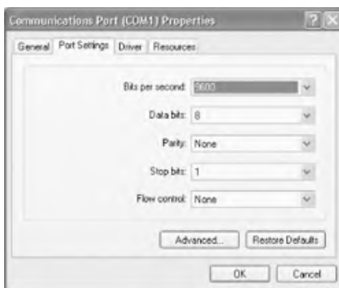
Figure 22-11. Use the Windows 2000/XP Port Settings dialog to change default speed and framing parameters
