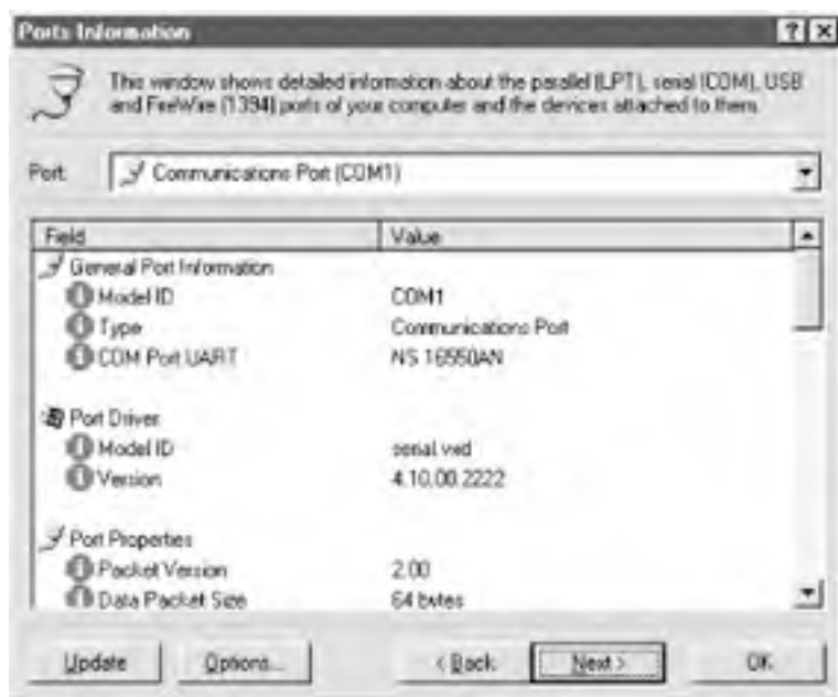
Figure 22-3. Using SiSoft Sandra Ports Information to view serial port configuration on a Windows 98 system
