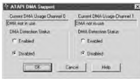
Figure 14-2. In Windows NT, use Dmacheck.exe to view and set DMA options
