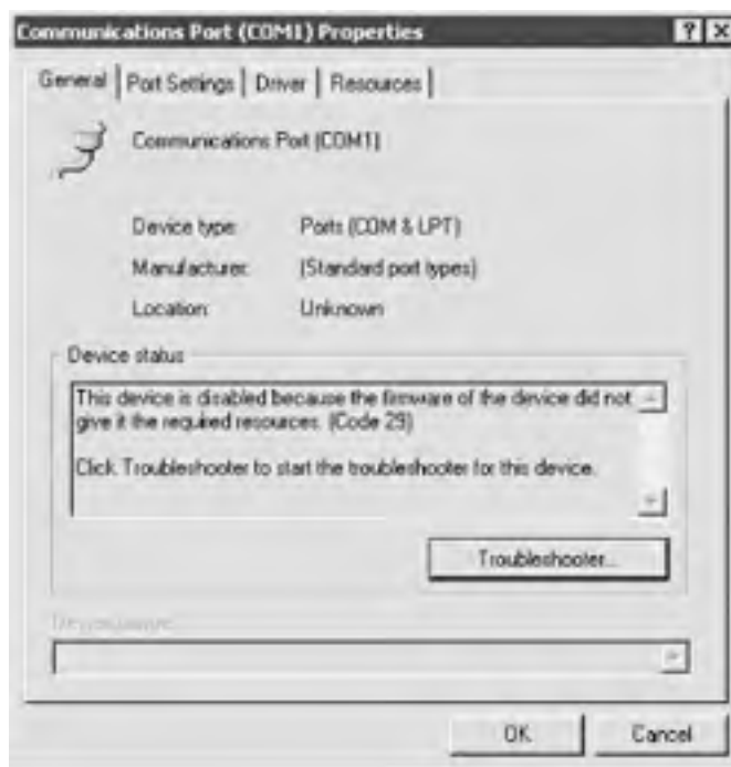
Figure 22-14. Windows displays Device status as disabled when it does not recognize a port
