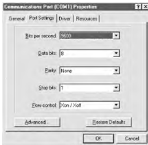
Figure 22-6. Use the Port Settings page to configure communication parameters for the port
