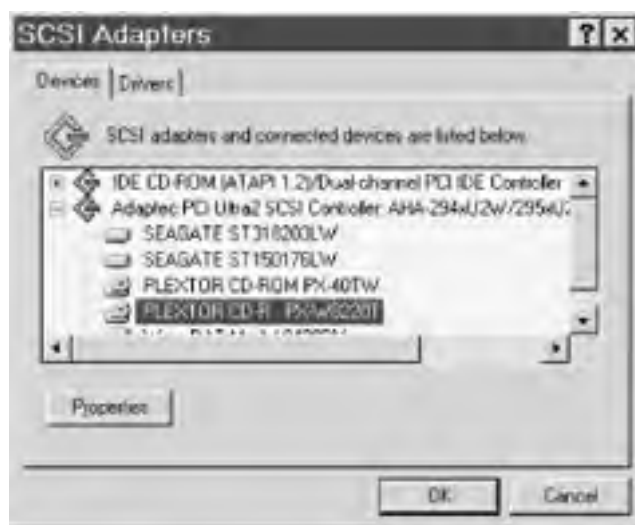
Figure 11-3. The Windows NT 4 SCSI Adapters dialog displays all installed IDE and SCSI devices
