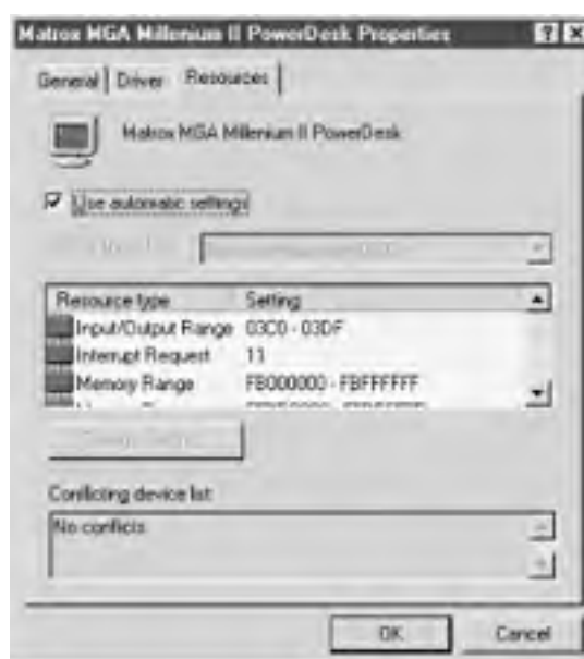
Figure 1-10. The Properties sheet for a device lists all resources allocated to that device
