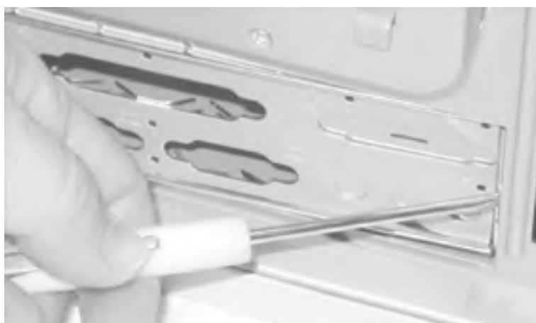
Figure 28-8. If necessary, use a small flat-blade screwdriver to pop the template
