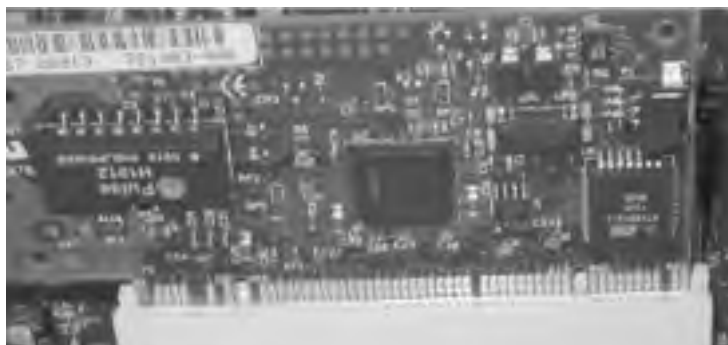
Figure 2-6. An expansion card properly aligned and ready to seat
