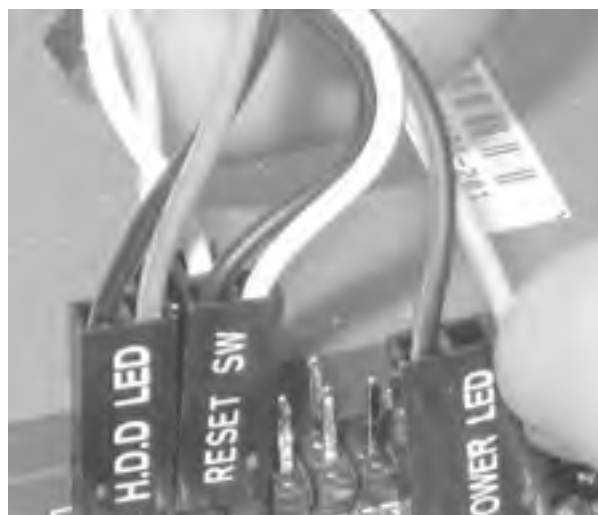
Figure 28-39. Connect cables for front-panel switches and indicators to the motherboard
