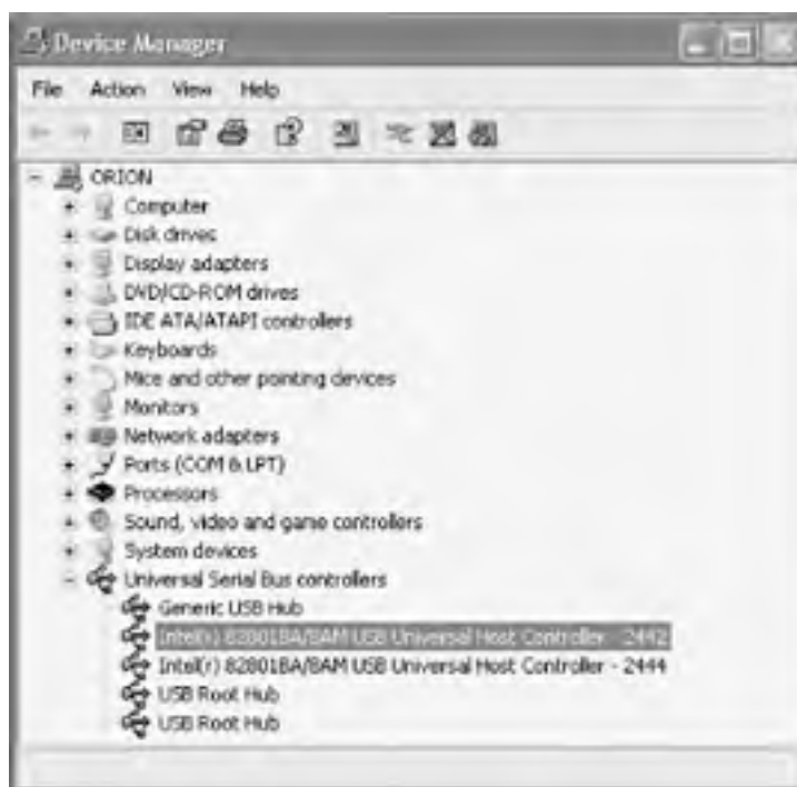
Figure 24-9. Windows XP Device Manager shows this system uses two Intel 82801BA/BAM UHCIs
