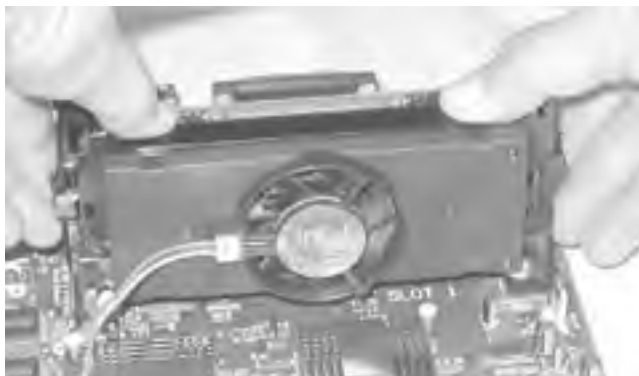
Figure 4-18. Press firmly until the processor seats fully
