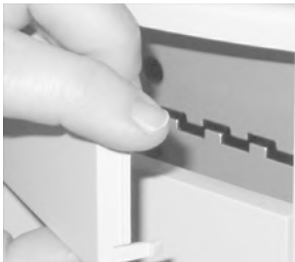
Figure 28-2. Removing a drive bay bezel with the main front bezel still in place (an anti-RFI plate is visible behind the bezel)
