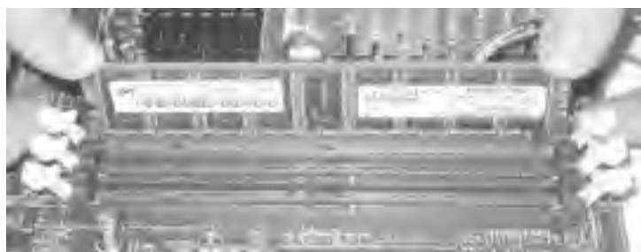
Figure 5-6. Align the DIMM module and press straight down until it seats
