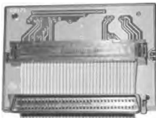
Figure 13-5. LVD SCSI cable with a built-in active terminator
