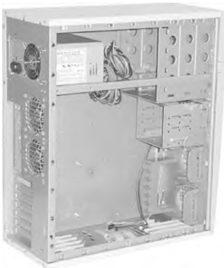
Figure 28-1. The Antec SX840 mid-tower case with side panel removed (note the two standard 80mm fans at rear and positions for two optional 80mm fans at front)
