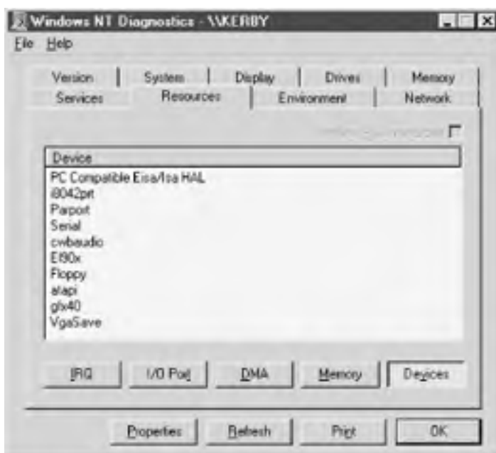
Figure 1-15. The Resources page Devices view shows a list of all installed devices
