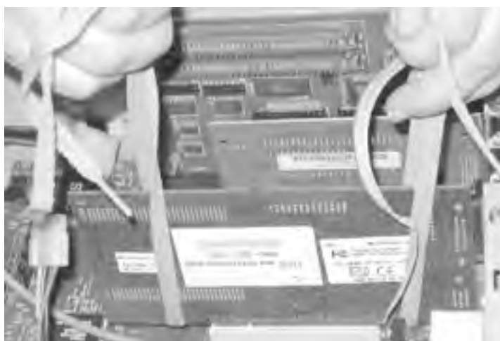
Figure 2-8. Pulling a recalcitrant expansion card the safe way
