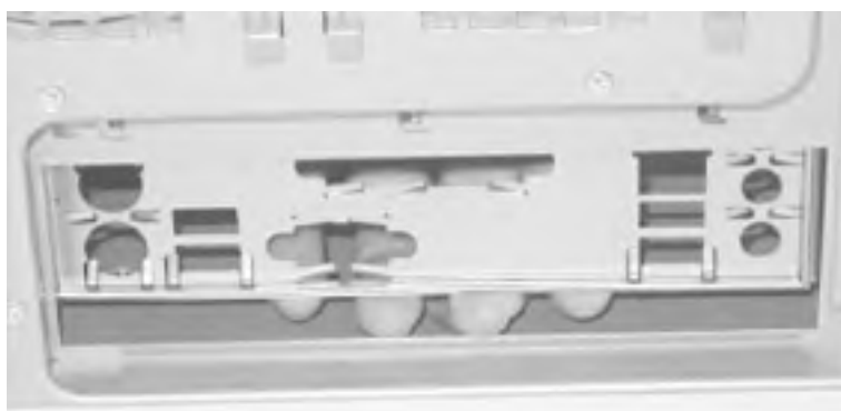
Figure 28-9. Insert the I/O template from inside the case and press gently until it snaps into place
