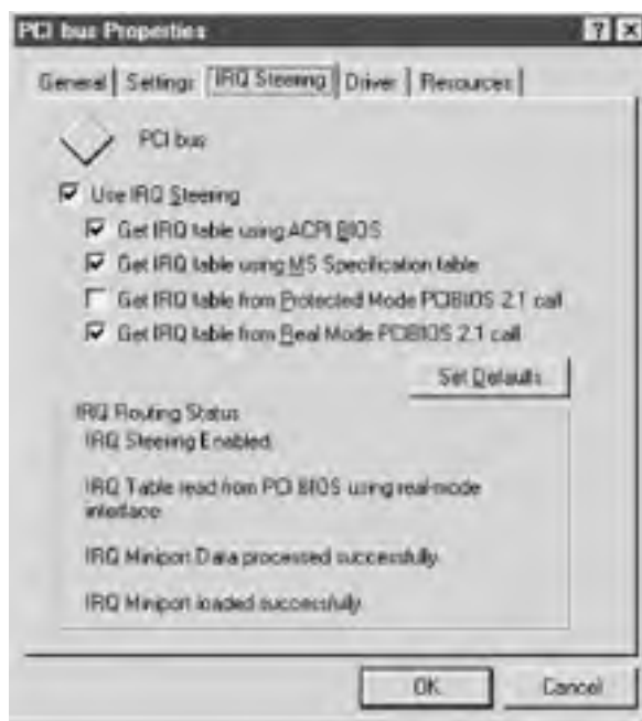
Figure 1-4. The IRQ Steering page of the PCI bus Properties dialog allows you to enable or disable Windows 98 IRQ Steering, configure it, and view its current status
