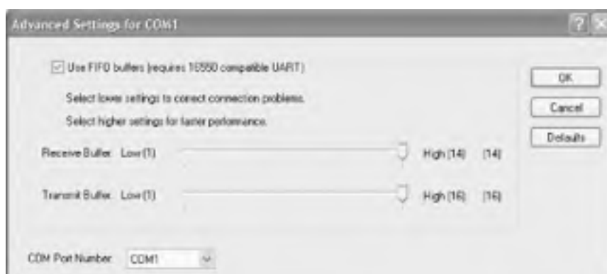
Figure 22-12. Adjust the Receive Buffer and Transmit Buffer sliders for optimum performance
