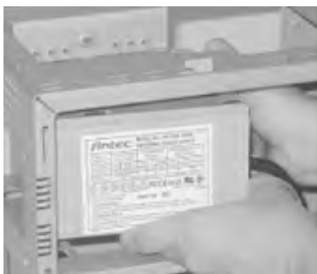
Figure 26-5. Slide the power supply into position
