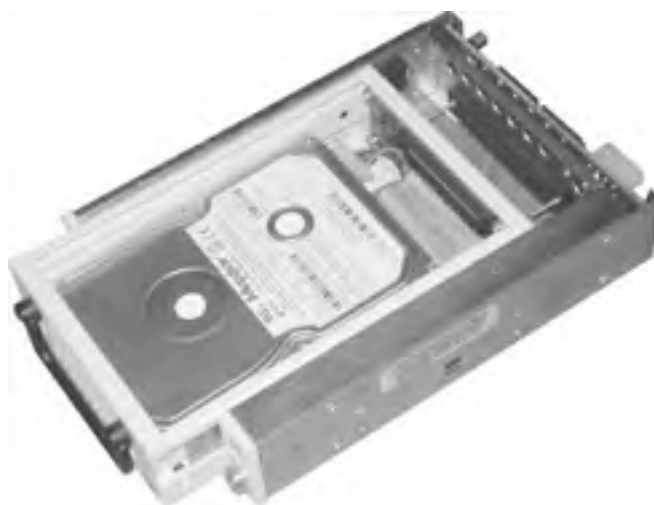
Figure 8-2. StorCase Data Express DE-100 frame, with carrier partially inserted
