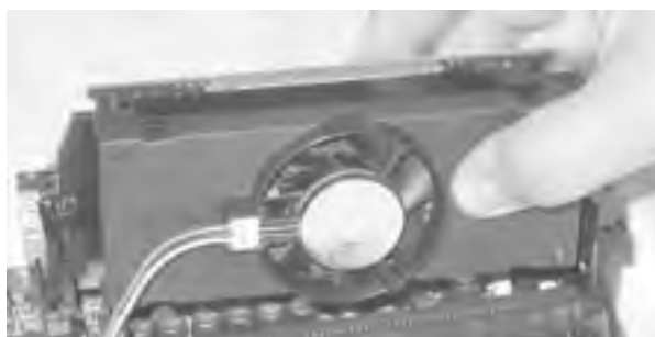
Figure 4-17. Guide the processor into place, aligning the keying tab in the slot with that in the processor's card-edge connector
