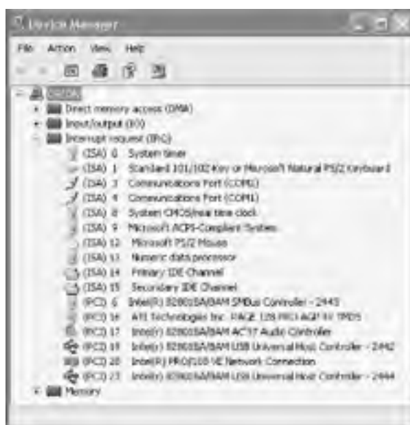
Figure 1-6. Windows XP Device Manager displays used and available IRQs
