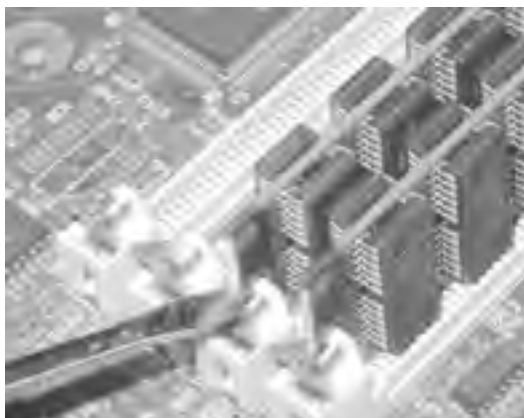
Figure 5-5. While maintaining gentle pressure on the module, use a small screwdriver to press down on the locking tabs until they release
