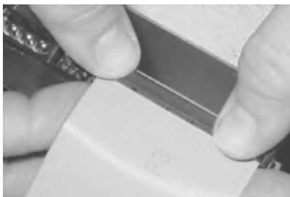
Figure 28-26. Connecting the data cable to the Seagate Barracuda ATA IV hard drive (this drive uses an Ultra ATA cable, which is easily discernible from a standard ATA cable by the finer wires)
