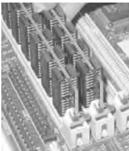
Figure 5-4. Rotate the SIMM to vertical and make sure the locking tabs snap into place
