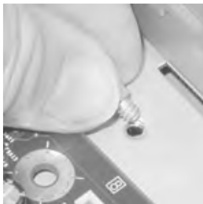
Figure 28-11. Install a brass standoff spacer for each motherboard mounting hole
