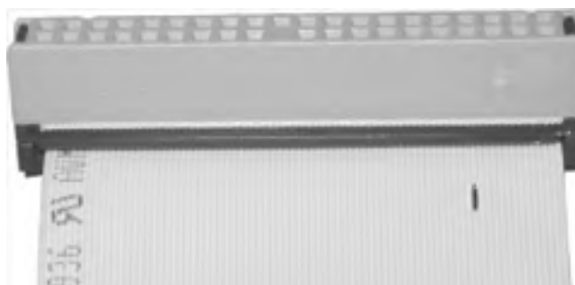
Figure 13-1. An Ultra DMA cable, showing pin 34 cut
