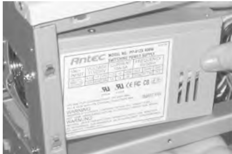
Figure 28-5. Insert the screws (typically four) to secure the power supply
