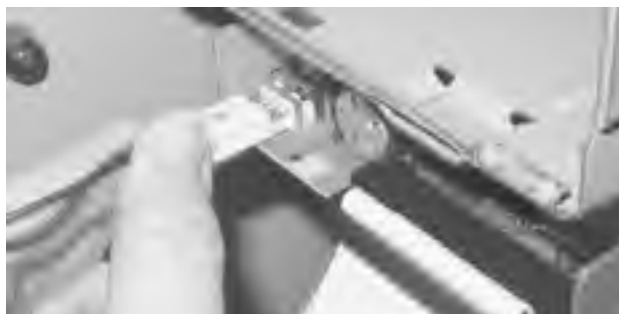
Figure 6-6. Connect the power cable to the FDD, making sure the connector is aligned properly with the pins
