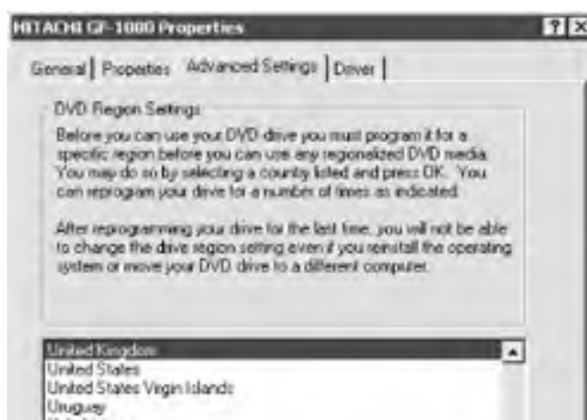
Figure 12-1. Using the Advanced Settings page of the drive Properties dialog to set the DVD Region Code
