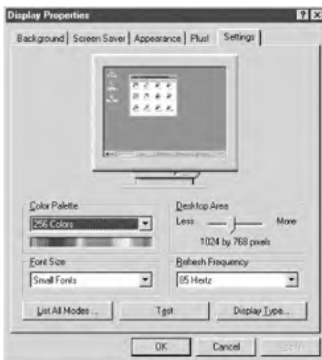
Figure 15-4. Use the Display Properties Settings page in Windows NT 4 to configure all video settings
