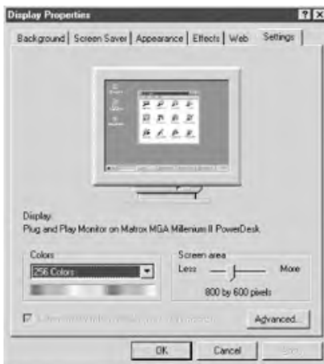
Figure 15-2. Use the Display Properties Settings page to configure hardware settings for your video adapter and monitor
