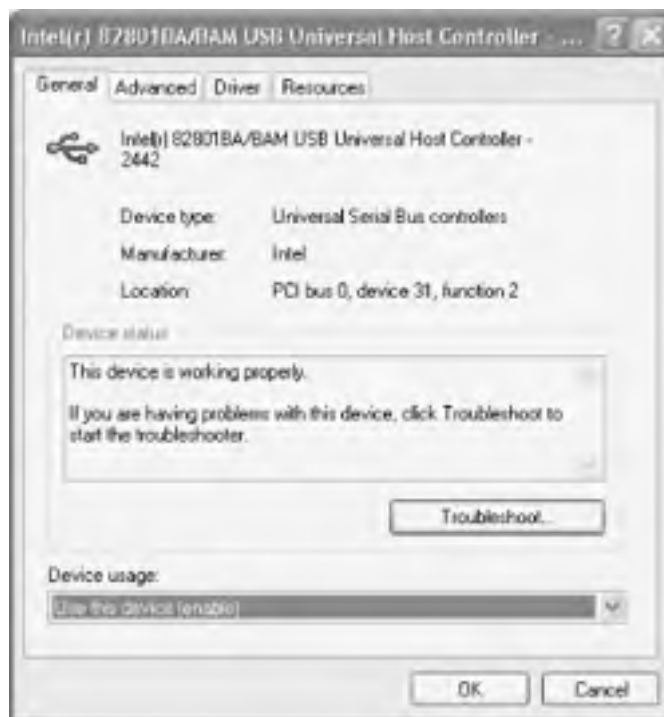
Figure 24-10. The Windows XP HCI Properties dialog displays detailed HCI information
