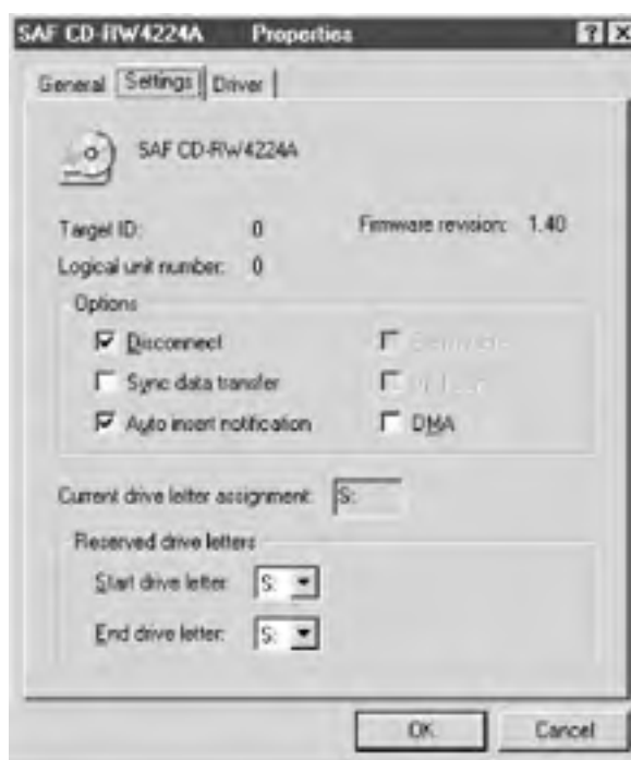
Figure 11-2. The Windows 98SE device Properties dialog shows that firmware revision 1.40 is installed on this CD writer
