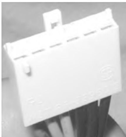
Figure 28-32. The Auxiliary ATX Power Connector plug
