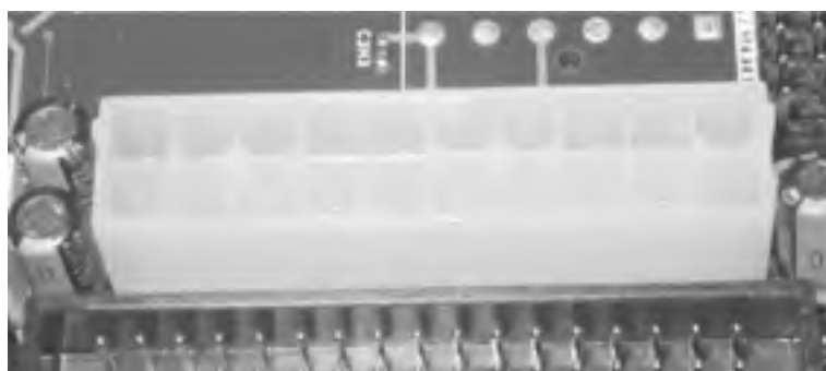
Figure 28-31. The main ATX power connector jack
