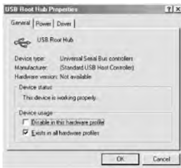
Figure 24-6. The Windows 9X Root Hub Properties dialog displays detailed root hub information
