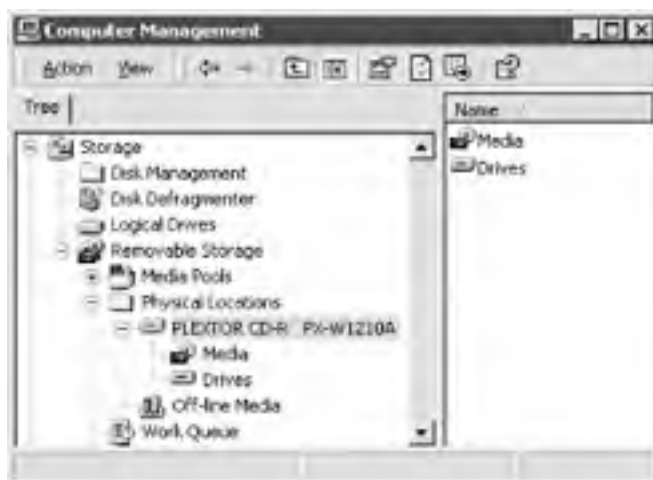
Figure 11-5. Using Windows 2000 Computer Management to view properties for the CD writer
