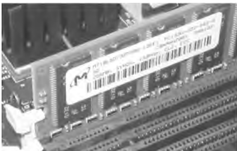
Figure 28-22. When the memory module is seated properly, the plastic retaining arm on each end automatically pivots into place, locking the module into the slot
