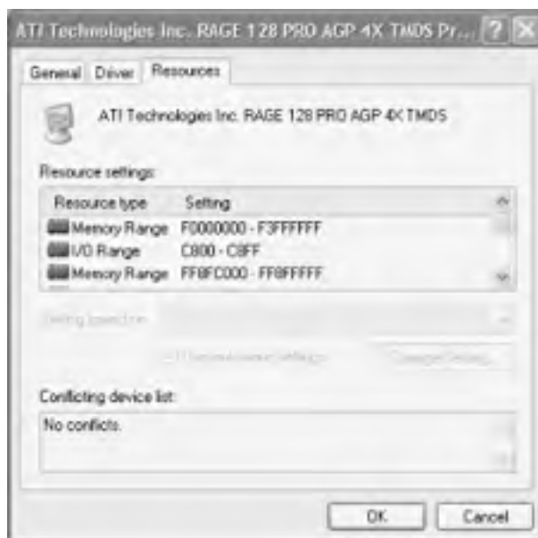
Figure 1-7. The Properties sheet for a device lists all resources allocated to that device
