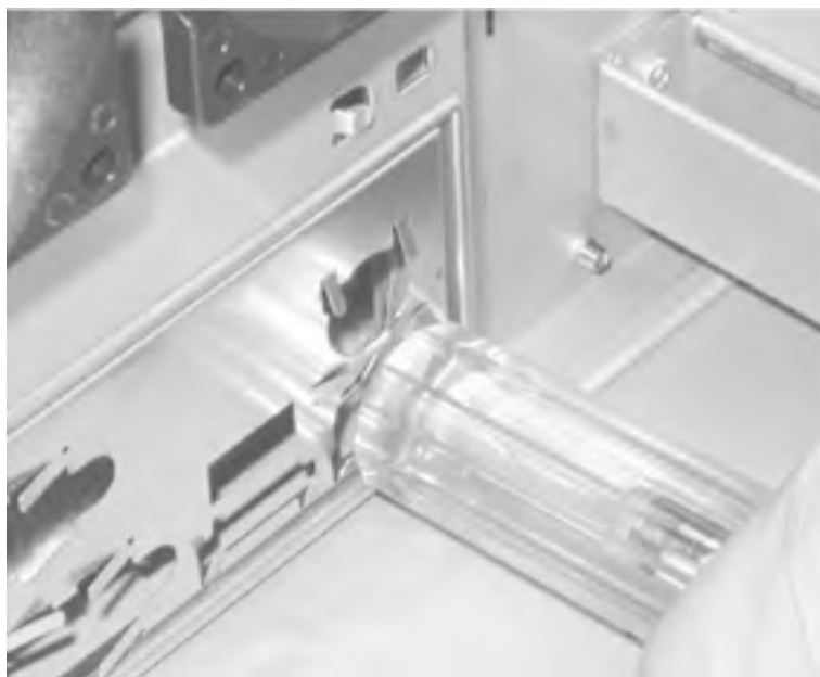
Figure 28-10. If the template refuses to seat, press gently with the handle of screwdriver until you feel it snap into place
