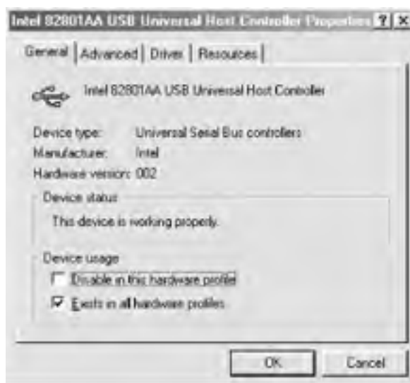
Figure 24-5. The Windows 9X HCI Properties dialog displays detailed HCI information
