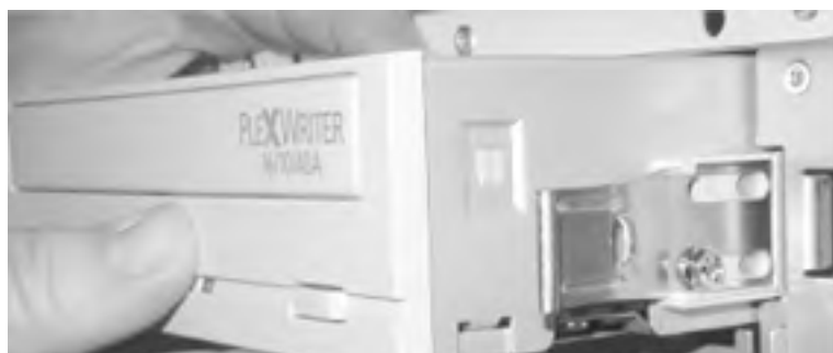
Figure 28-29. The traditional arrangement, in which rails mounted to the drive slide into matching slots in the chassis and are secured by a front screw or clips
