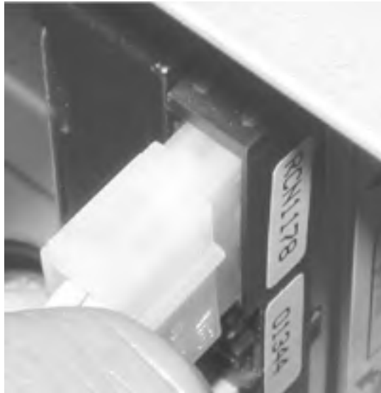
Figure 28-38. Connect power cables to the drives
