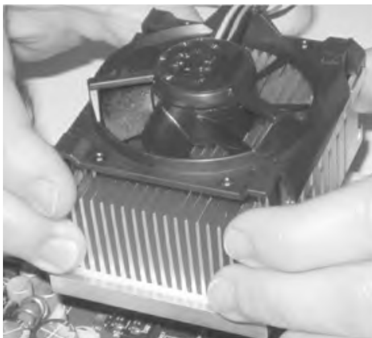
Figure 28-17. After applying thermal compound, align the heatsink squarely on top of the processor
