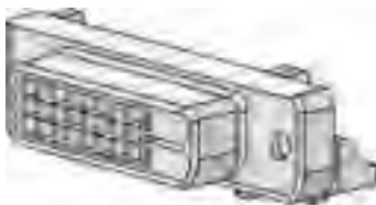
Figure 16-3. DVI-I hybrid digital/analog connector
