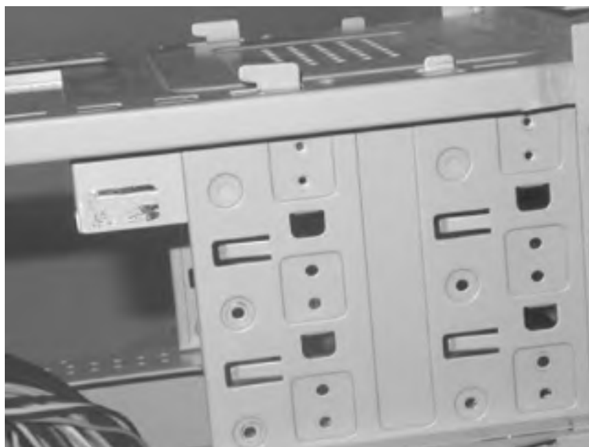
Figure 28-27. A typical mini-tower arrangement, where drives secure directly to the chassis
