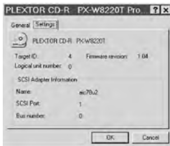
Figure 11-4. The Windows NT device Properties dialog shows that firmware revision 1.04 is installed on this CD writer
