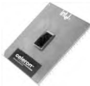
Figure 4-5. Intel Celeron processor in FC-PGA package (photo courtesy of Intel Corporation)
