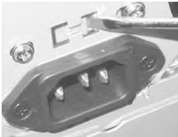
Figure 28-6. If the power supply has a voltage selector switch, make sure to set it correctly
