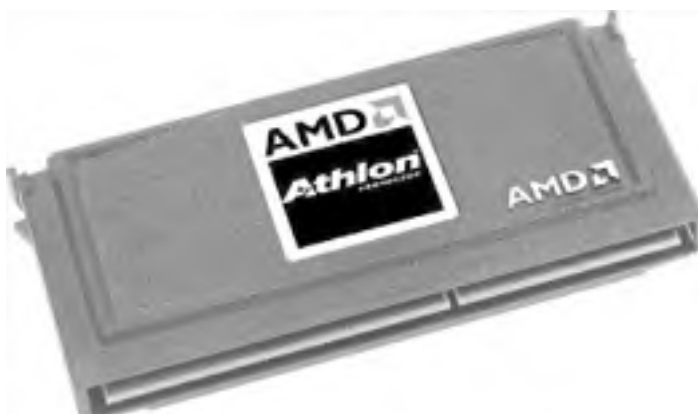
Figure 4-10. A Slot A Athlon processor (image courtesy of Advanced Micro Devices, Inc.)
