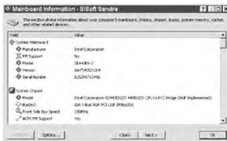
Figure 3-2. SiSoft Sandra identifies the chipset as an Intel 440BX
