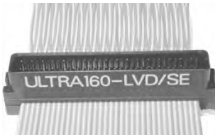
Figure 13-4. SCSI P cable with 68-pin high-density connector
