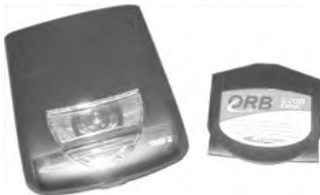
Figure 8-1. An external UltraSCSI Castlewood ORB 2.2 drive and cartridge
