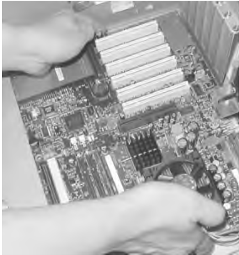
Figure 28-12. Compare motherboard mounting holes against chassis standoff positions to make sure everything lines up
