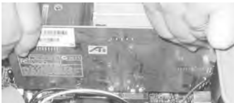
Figure 28-43. When you're sure the card is aligned, press down firmly with both thumbs until it seats fully
