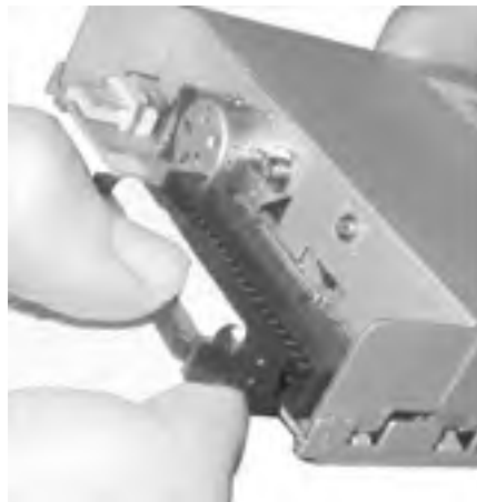
Figure 6-4. Connect the cable to the FDD, with pin 1 oriented properly and all pins aligned
