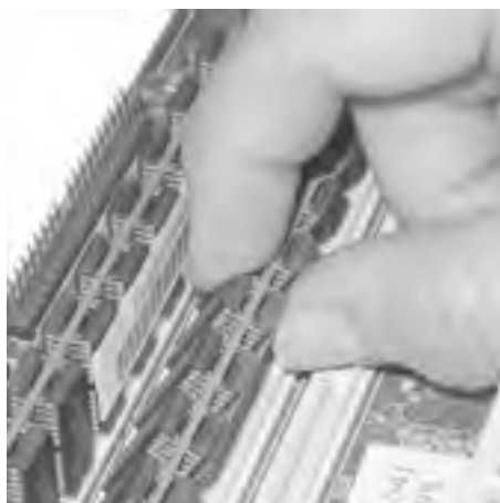
Figure 5-3. Insert the SIMM at a 45 degree angle
