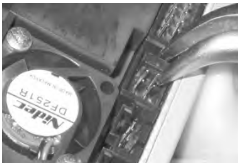
Figure 28-23. Using needle-nose pliers to set the drive select jumper on the rear panel of the Plextor PlexWriter to Master
