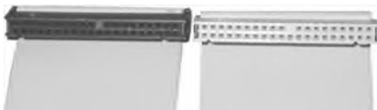
Figure 13-2. Standard 40-wire cable (left) and 80-wire cable
