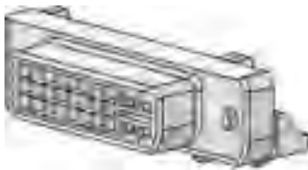
Figure 16-3. DVI-I hybrid digital/analog connector
