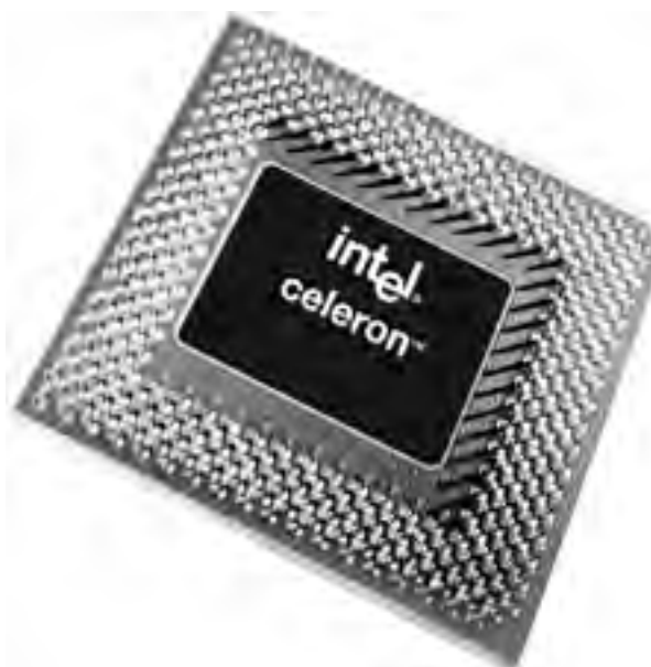
Figure 4-4. Intel Celeron processor in PPGA package (photo courtesy of Intel Corporation)
