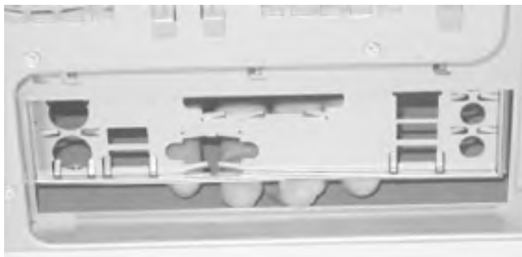
Figure 28-10. Using the handle of a screwdriver to gently press a template that refuses to seat
