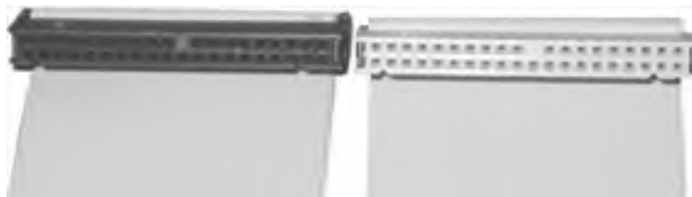
Figure 13-2. Standard 40-wire ATA cable (left) and Ultra DMA 80-wire cable
