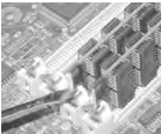
Figure 5-5. Using a small screwdriver to press down on the locking tabs until they release, while maintaining gentle pressure on the module
