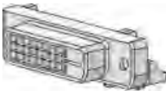
Figure 16-3. DVI-I hybrid digital/analog connector
