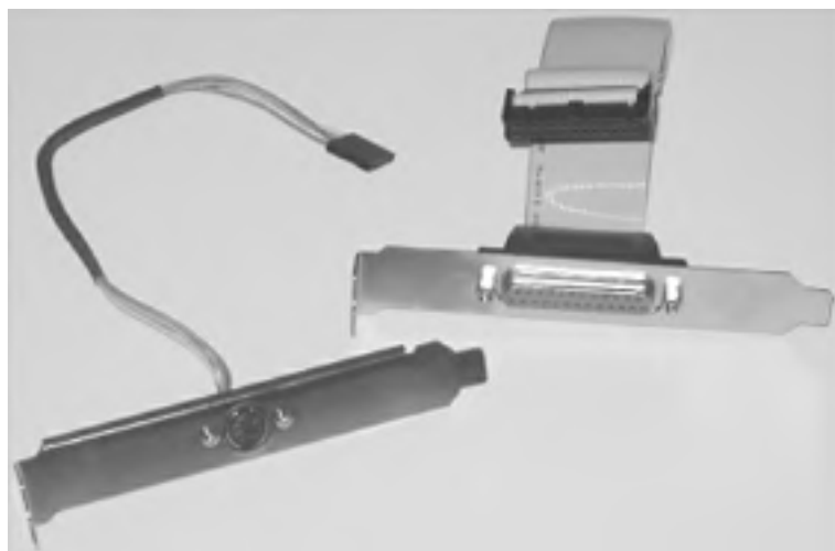
Figure 28-36. Typical port extenders for an AT motherboard (on the left is a PS/2 mouse connector, on the right is a DB25 serial port connector)
