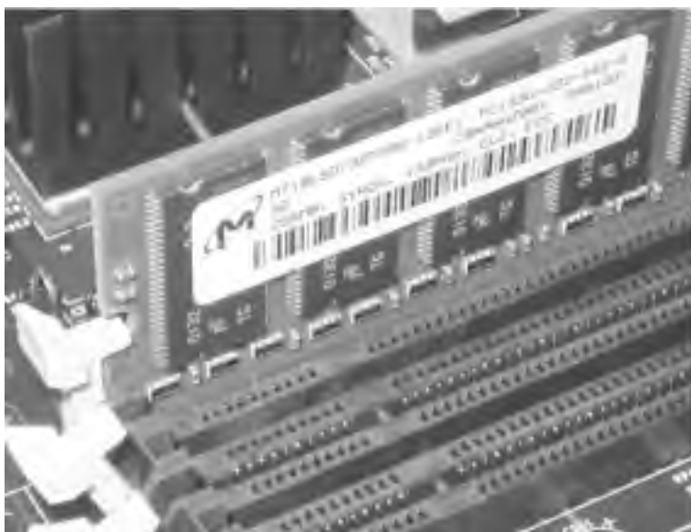
Figure 28-22. When the memory module is seated properly, the plastic retaining arm on each end automatically pivots into place, locking the module into the slot
