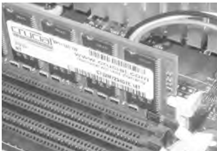
Figure 5-7. The ejector arms pivoting back to the vertical when the memory module is fully seated
