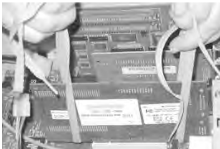
Figure 2-8. Barbara pulling a recalcitrant expansion card the safe way
