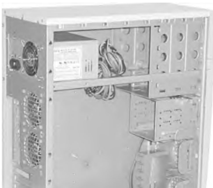
Figure 28-1. The Antec SX840 mid-tower case with side panel removed (note the two standard 80mm fans at rear and positions for two optional 80mm fans at front)
