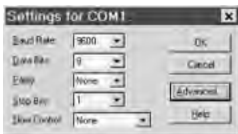
Figure 22-9. The Windows NT 4 Settings dialog, where you configure communication parameters for the port
