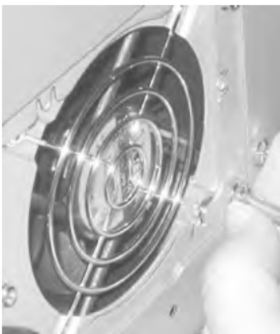
Figure 28-5. Inserting the screws (typically four) to secure the power supply
