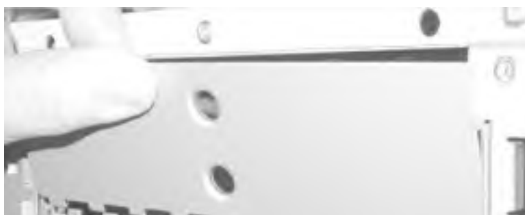
Figure 28-3. Removing an anti-RFI plate with the main front bezel removed
