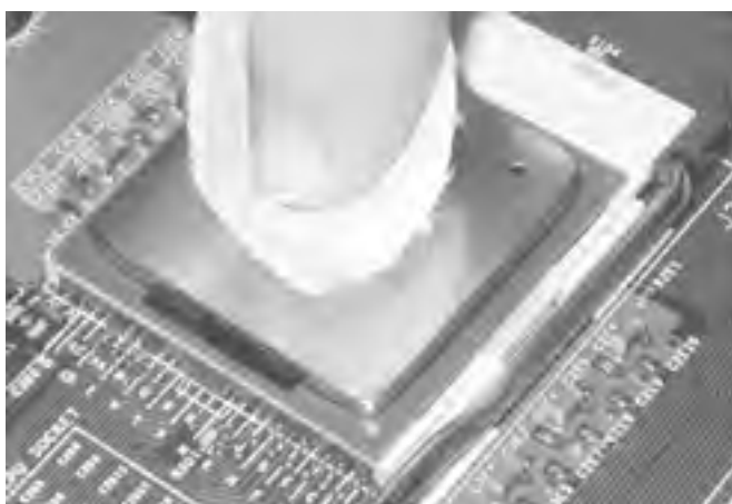
Figure 28-15. Polishing the processor carefully before applying thermal compound
