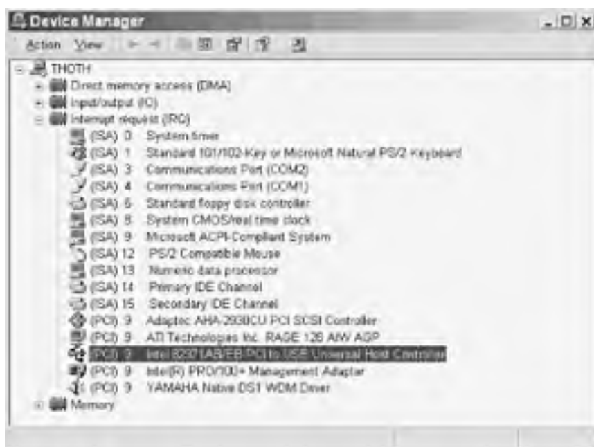
Figure 24-13. Windows 2000 Device Manager showing that this system shares one interrupt among the USB HCI and four other devices
