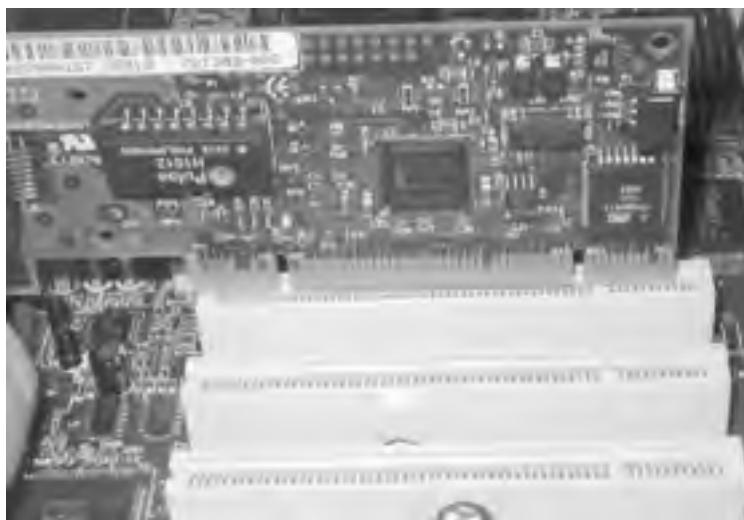
Figure 2-7. The same card in a cheap case, not aligning properly with the expansion slot
