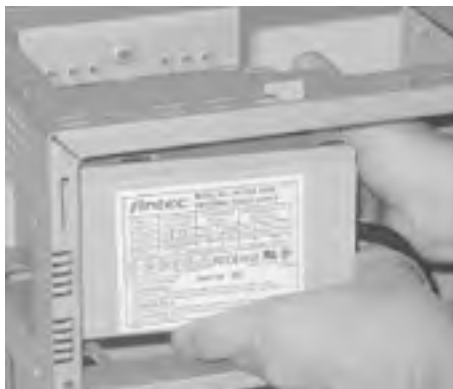
Figure 26-5. Sliding the power supply into position
