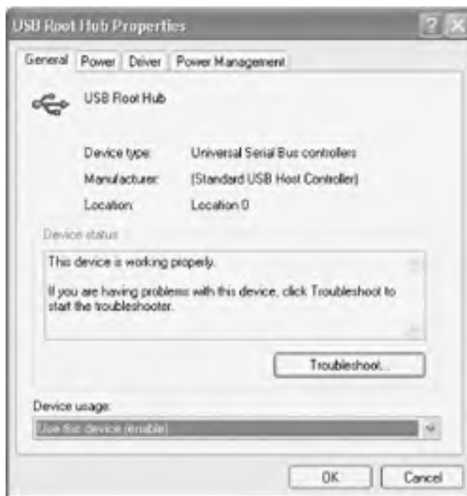
Figure 24-11. The Windows XP Root Hub Properties dialog displaying detailed root hub information
