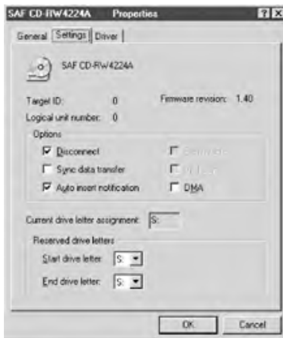
Figure 11-2. The Windows 98SE device Properties dialog, which shows that firmware revision 1.40 is installed on this CD writer
