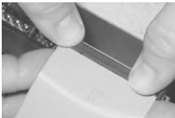
Figure 28-26. Connecting the data cable to the Seagate Barracuda ATA V hard drive (this drive uses an Ultra ATA cable, which is easily discernible from a standard ATA cable by the finer wires)
