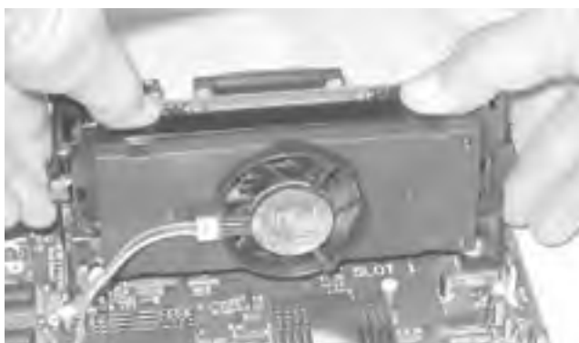
Figure 4-18. Using both thumbs to press firmly until the processor seats fully
