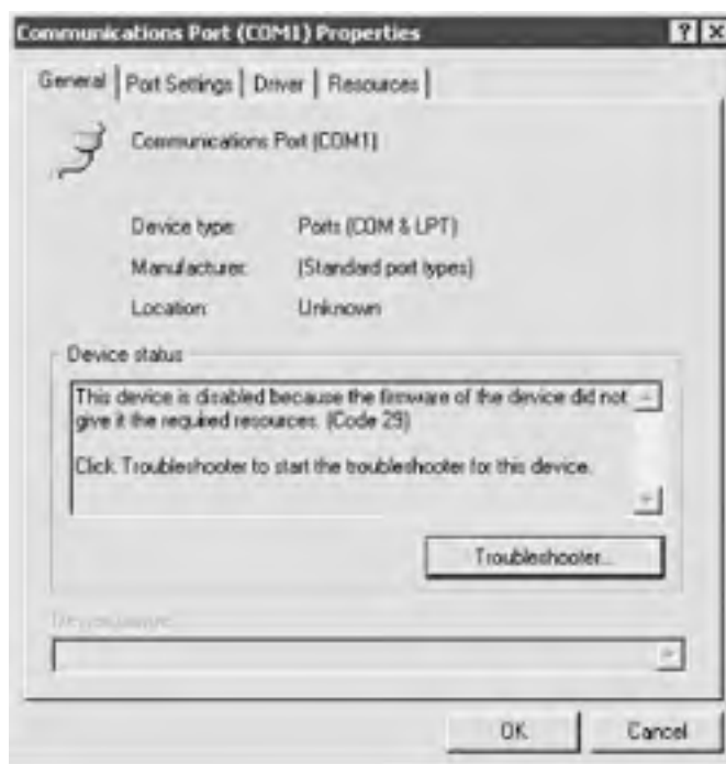
Figure 22-14. Windows displaying Device status as disabled when it does not recognize a port
