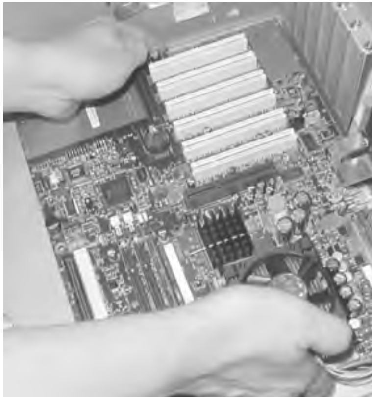
Figure 28-12. Comparing motherboard mounting holes against chassis stand-off positions to make sure everything lines up
