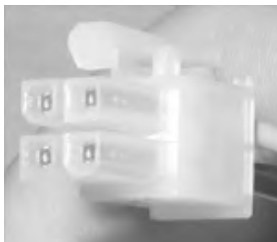
Figure 28-34. If you forget to insert the ATX12V Supplementary Power Connector, your Pentium 4 motherboard will not boot.
