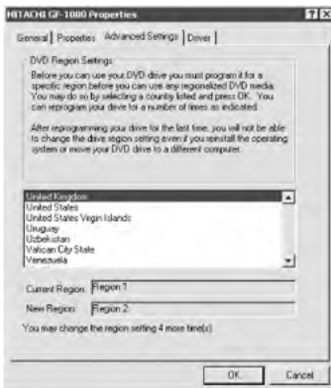
Figure 12-1. Using the Advanced Settings page of the Properties dialog to reset the DVD Region Code with Windows 2000 Professional
