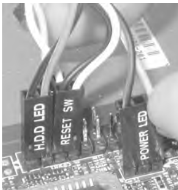
Figure 28-39. Connecting cables for front-panel switches and indicators to the motherboard
