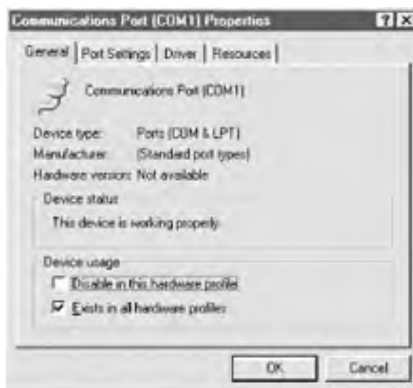
Figure 22-5. The General page of Communications Port Properties displaying the operational status of the port
