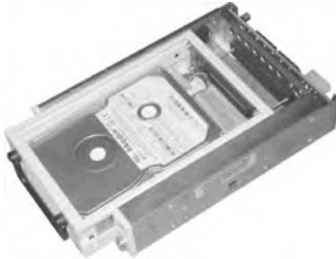
Figure 8-1. StorCase Data Express DE-100 frame, with carrier partially inserted
