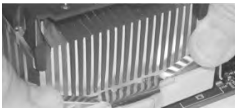
Figure 28-18. Snapping both heatsink support brackets over the matching connectors on the heatsink retention mechanism
