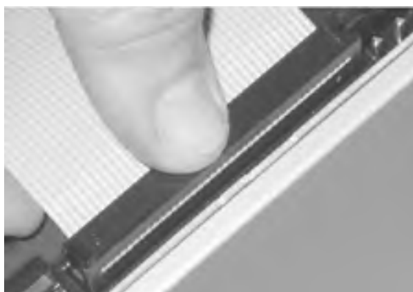
Figure 28-26. Connecting the data cable to the Seagate Barracuda ATA V hard drive (this drive uses an Ultra ATA cable, which is easily discernible from a standard ATA cable by the finer wires)
