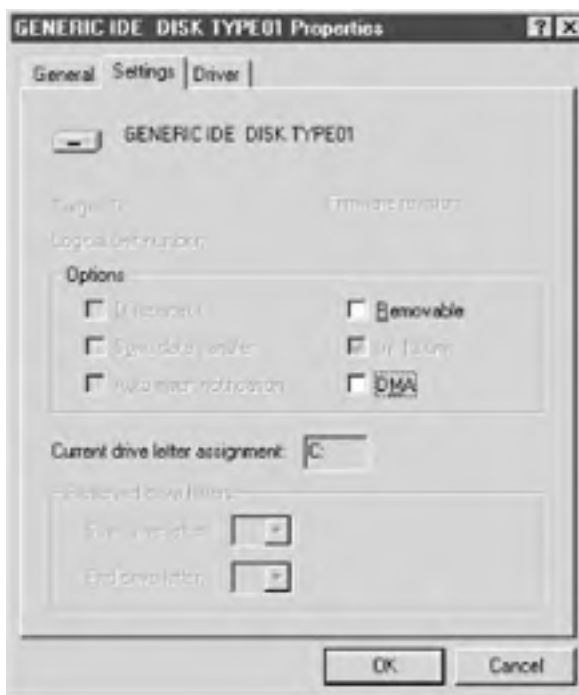
Figure 14-3. In Windows 9X, marking the DMA checkbox on the Settings page of the disk Properties dialog to enable DMA transfers
