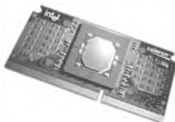
Figure 4-3. Intel Celeron processor in SEPP package (photo courtesy of Intel Corporation)
