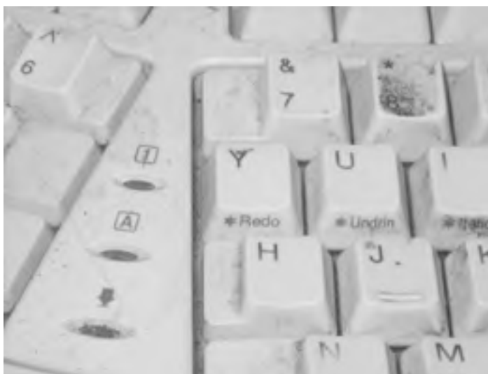
Figure 19-7. The same keyboard after a trip through the dishwasher
