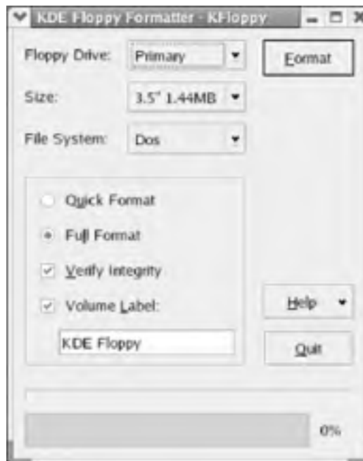
Figure 6-1. The KDE Floppy Formatter avoids having to mount the diskette or remember command-line options
