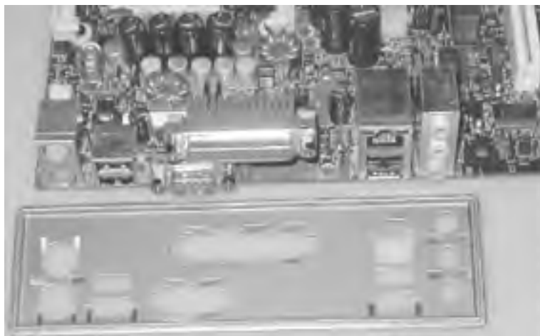
Figure 28-7. A motherboard I/O panel and matching I/O template
