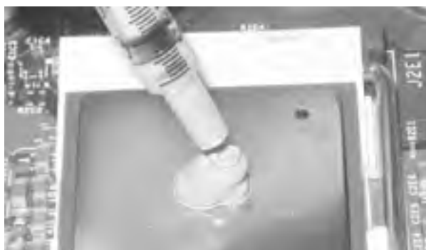
Figure 28-16. Applying the supplied thermal compound as a small pile at the center of the processor
