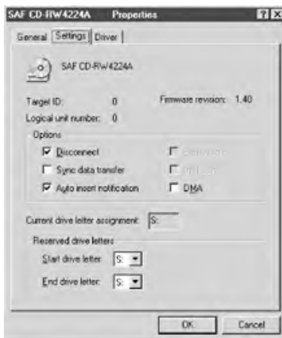
Figure 11-5. The device Properties sheet from within the Device Manager, where you can view or change the status of AIN under Windows 9x
