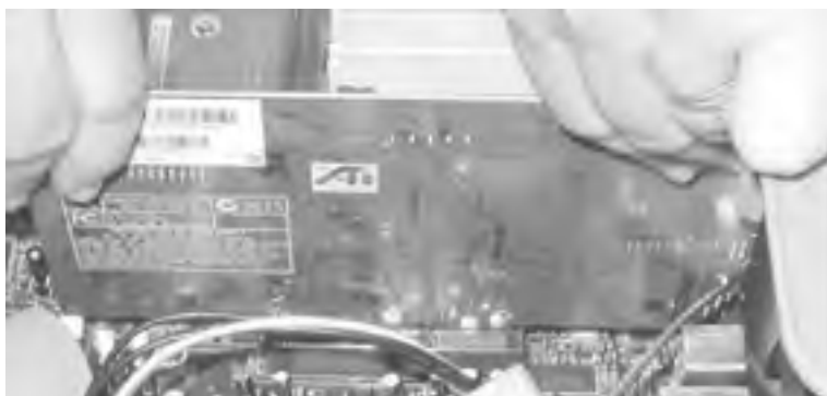
Figure 28-43. Using both thumbs to press the card straight down until it seats fully (be sure the card is aligned first)
