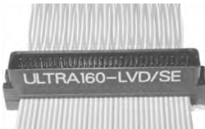
Figure 13-6. SCSI P cable with 68-pin high-density connector
