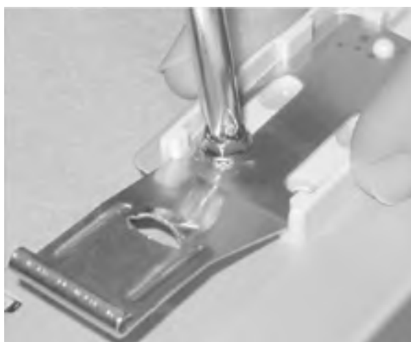
Figure 28-24. Securing the drive rails to the drive, making sure that the drive is electrically grounded to the chassis
