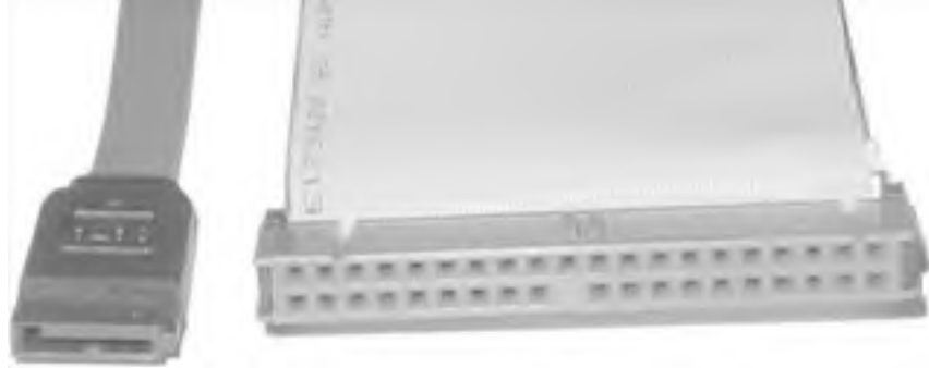
Figure 13-4. SATA cable (left) and UDMA 80-wire ATA cable
