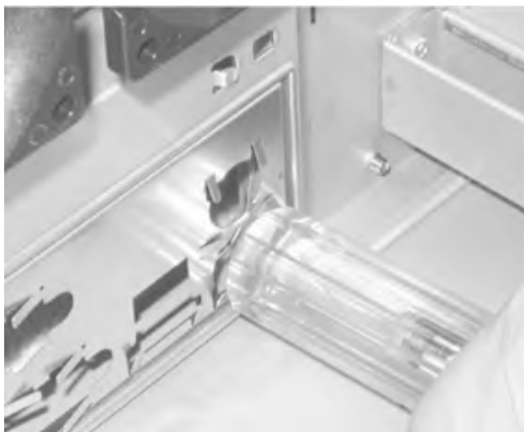
Figure 28-10. Using the handle of a screwdriver to gently press a template that refuses to seat
