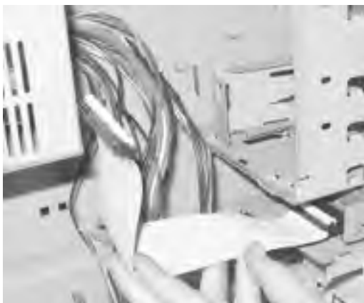
Figure 6-6. Sliding the FDD into the drive bay, making sure the cable feeds smoothly into the case interior
