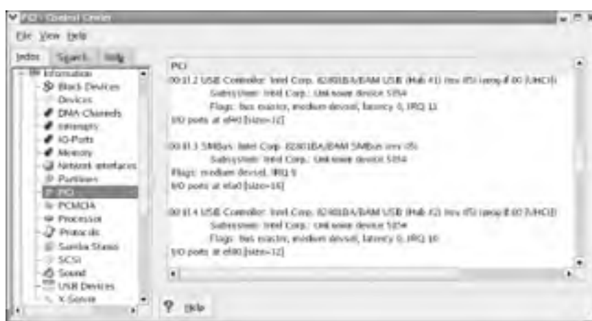
Figure 24-14. KDE Control Center displaying HCI type, I/O ports, and interrupts
