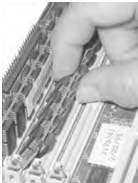
Figure 5-3. Inserting the SIMM at a 45-degree angle
