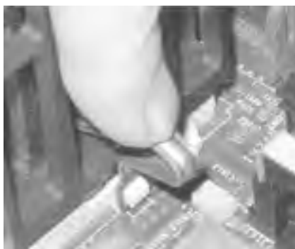
Figure 4-16. Attaching the heatsink securely using the locking clips
