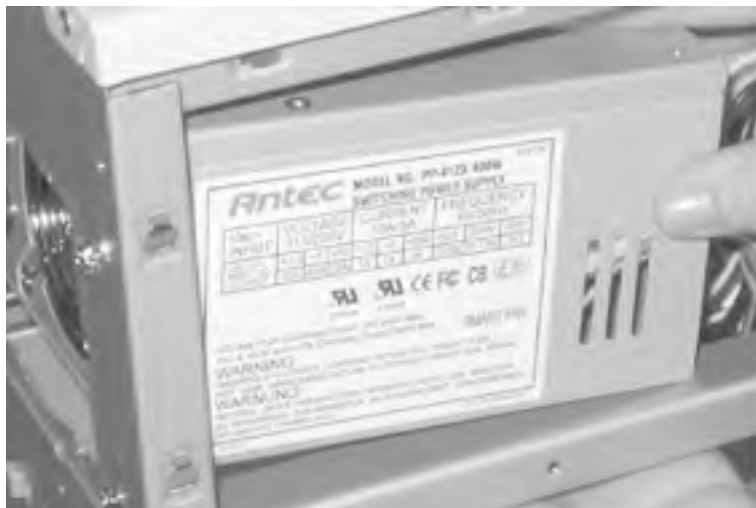
Figure 28-5. Inserting the screws (typically four) to secure the power supply
