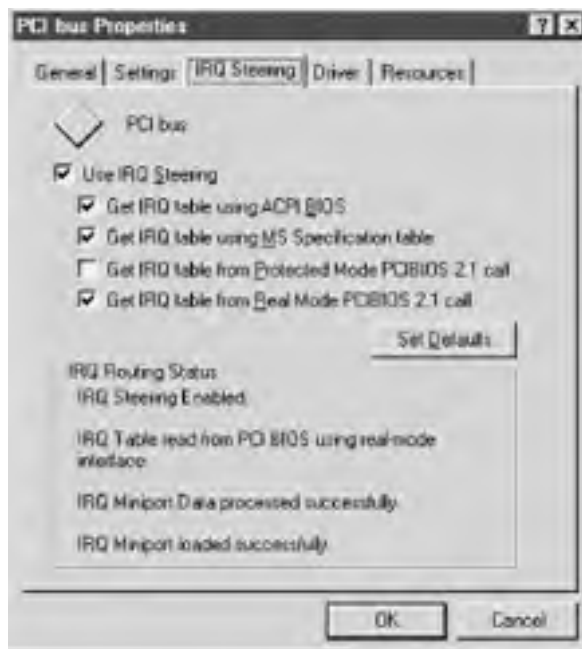
Figure 1-4. The IRQ Steering page of the PCI bus Properties dialog, which allows you to enable or disable Windows 98 IRQ Steering, configure it, and view its current status
