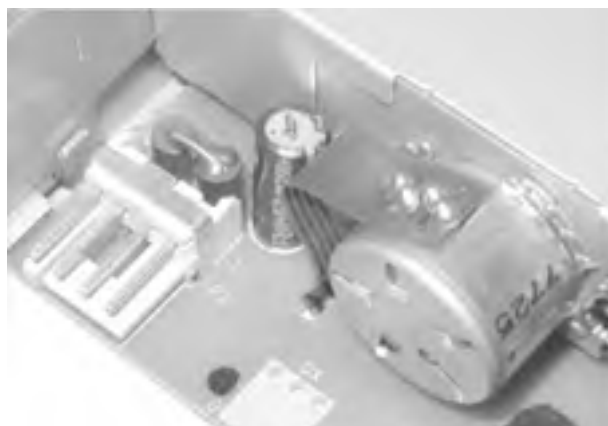
Figure 6-2. Unshrouded 4-pin power connector (labeled P2 here), used by all 3.5-inch FDDs
