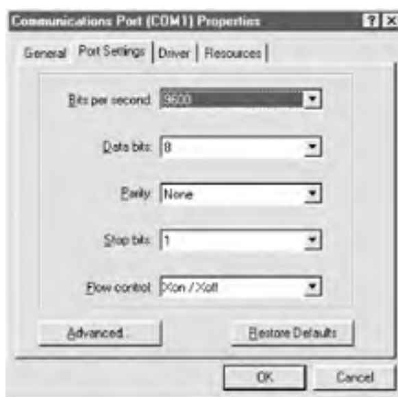
Figure 22-6. The Port Settings page, where you configure communication parameters for the port
