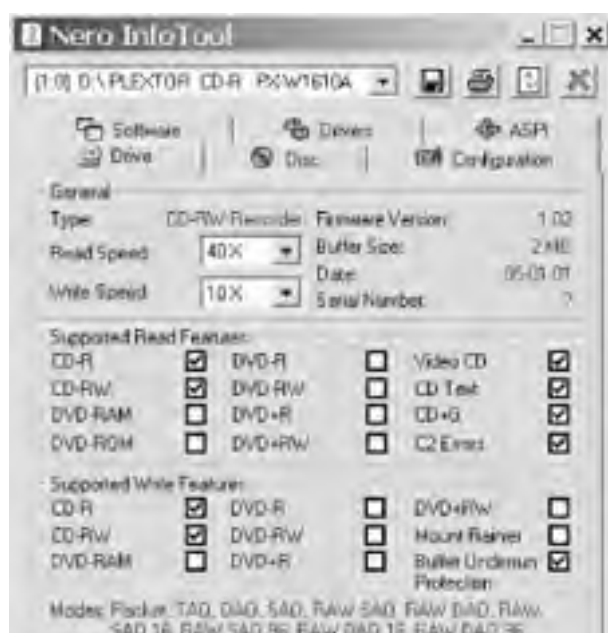
Figure 11-1. Nero InfoTool displaying the characteristics of this CD writer, showing the current firmware revision as 1.02
