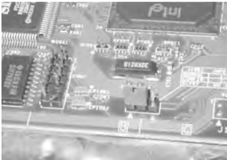
Figure 2-3. A typical PC jumper (bottom center) set to close pins 1 and 2
