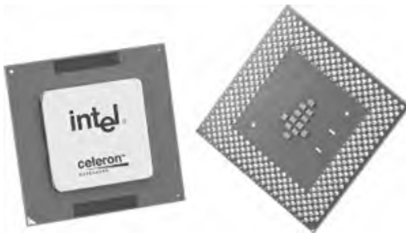
Figure 4-6. Intel Celeron processor in FC-PGA2 package (photo courtesy of Intel Corporation)
