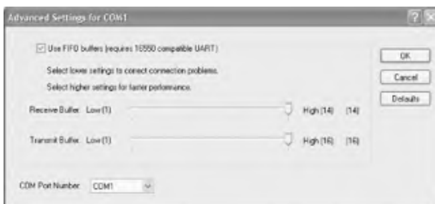
Figure 22-12. The Receive Buffer and Transmit Buffer sliders, which you can adjust for optimum performance
