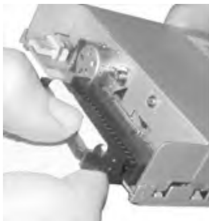
Figure 6-5. Connecting the cable to the FDD, with Pin 1 oriented properly and all pins aligned
