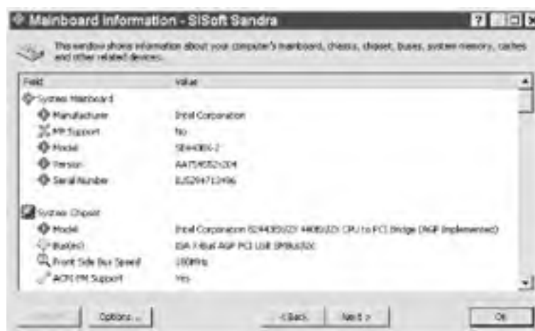
Figure 3-2. SiSoft Sandra identifying the chipset as an Intel 440BX
