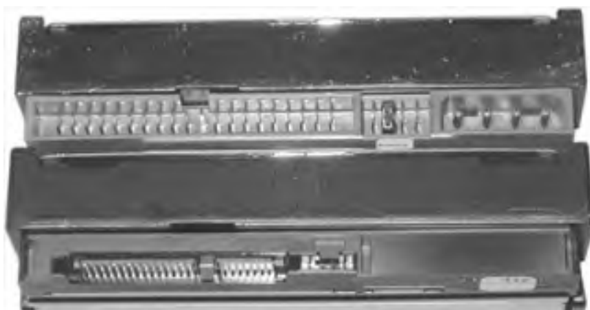
Figure 14-1. Two similar hard drives, with PATA (top) and SATA interfaces
