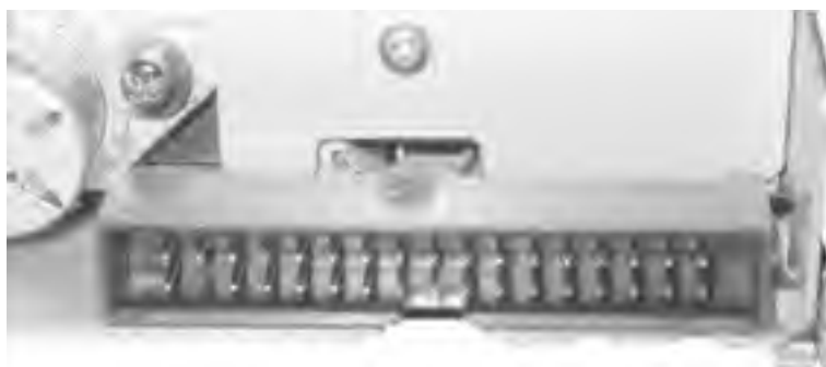
Figure 6-4. An NEC 3.5-inch FDD, which uses a shrouded cable connector rather than the typical bare pins (note the missing pin at lower left, which keys the connector)
