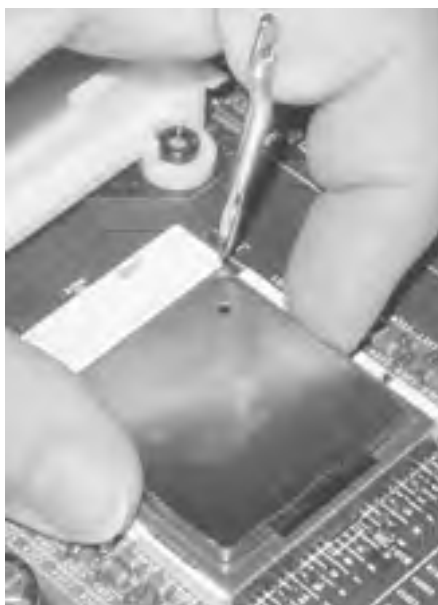
Figure 28-13. With the ZIF arm fully raised, carefully aligning the processor, making sure Pin 1 on the CPU corresponds to Pin 1 on the socket, and dropping the processor into place
