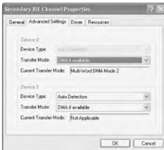
Figure 10-9. The Secondary IDE Channel Properties dialog, which shows that this drive is operating in Multi-Word DMA Mode 2
