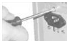
Figure 26-6. Securing the power supply by inserting the four screws (be sure to align it properly first)
