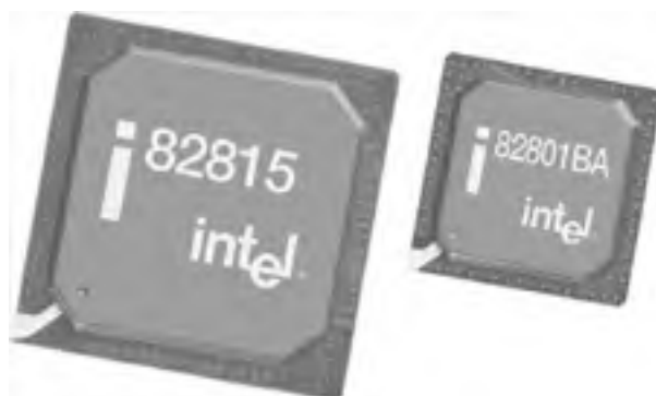
Figure 3-3. The Intel 815E chipset (image courtesy of Intel Corporation)
