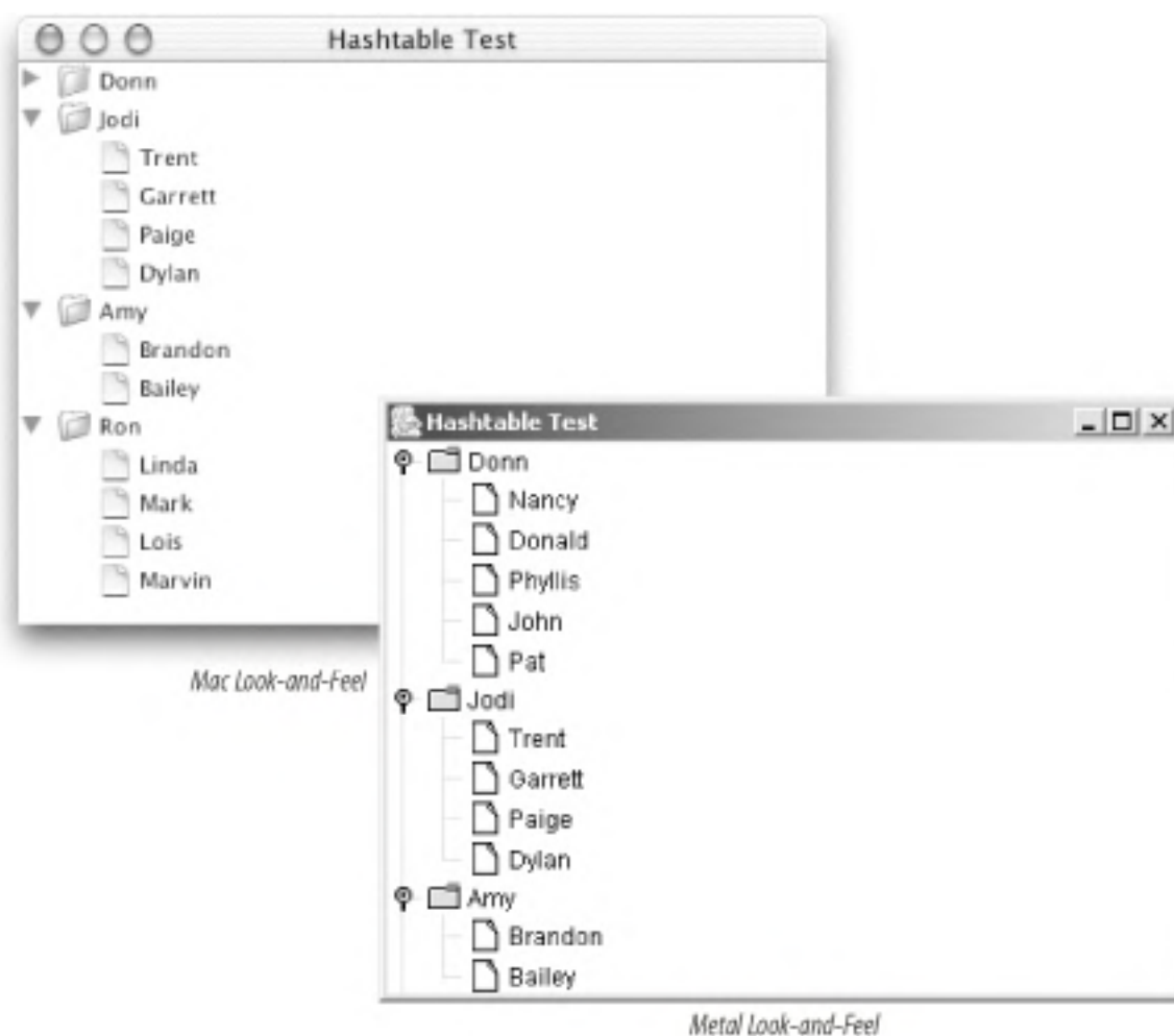
Figure 17-7. JTrees built from a hashtable and a DefaultTreeModel in Mac and Metal L&Fs
