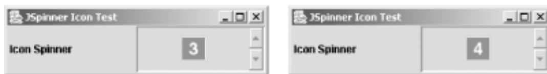
Figure 7-17. Our IconEditor used in a JSpinner (before and after pressing the up arrow)
