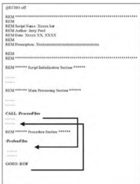
Figure 7.7: Internal procedures are created using the CALL command and a LABEL statement.
