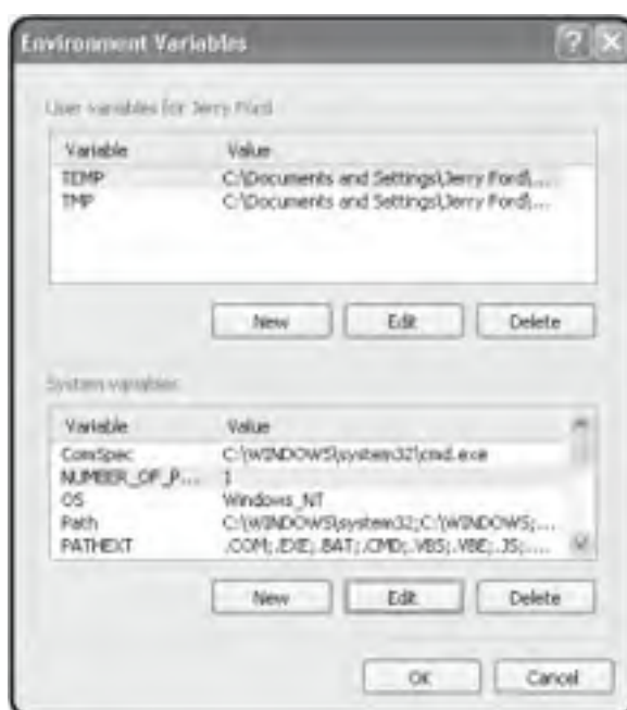
Figure 4.6: On Windows XP, both user and system environment variables can be viewed and modified from the Environment Variables dialog.
