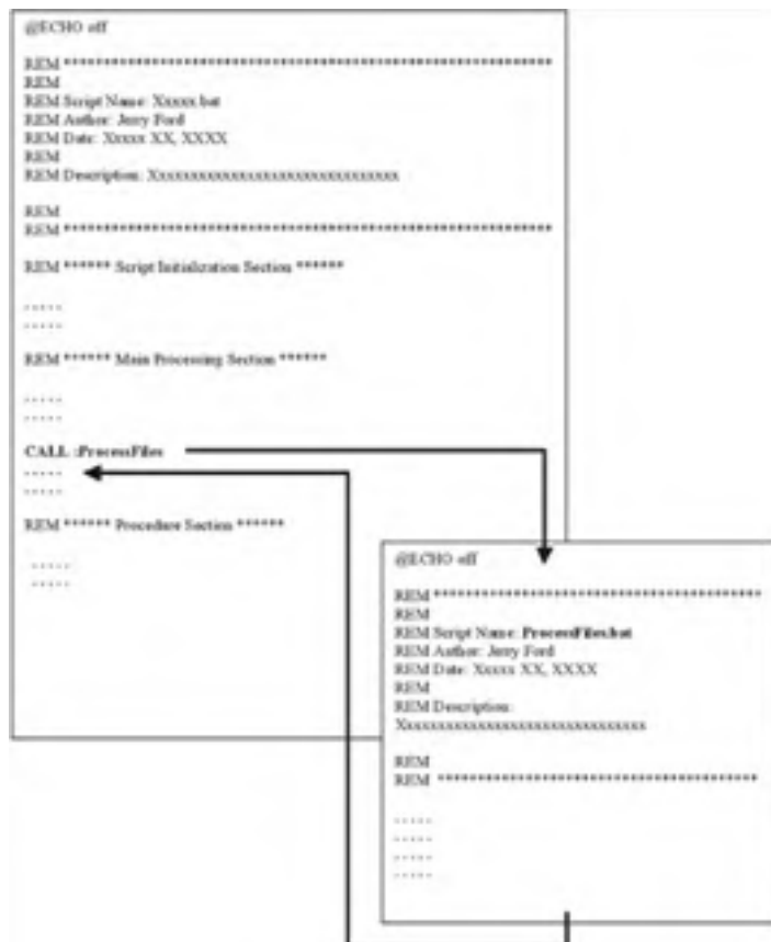
Figure 7.8: An external procedure allows a script to execute another script and wait on the called script to finish executing before resuming its own execution.
