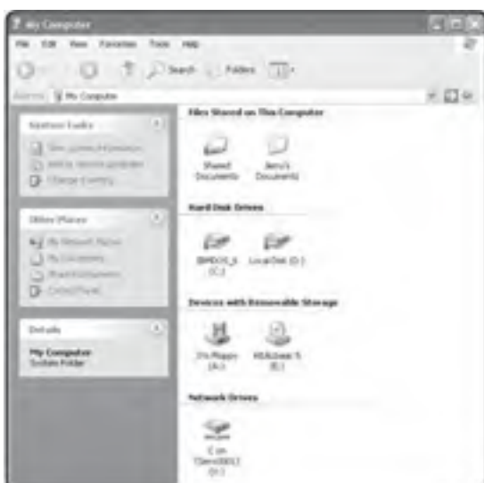
Figure A.2: The mapped network drive appears as an icon with a network cable connection shown beneath it.
