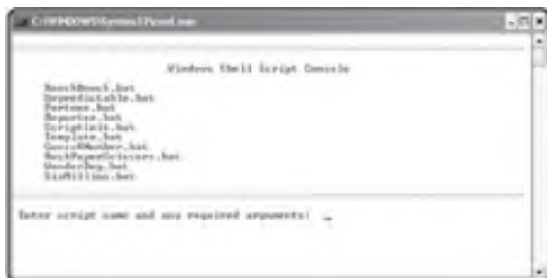
Figure 6.7: Using the FOR command to create a menu made up of file names.
