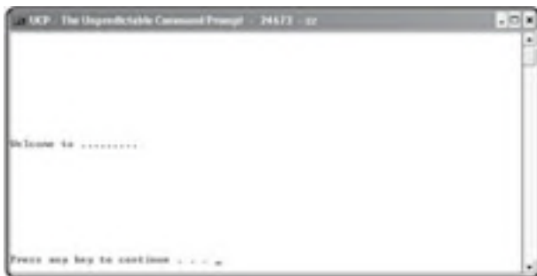
Figure 6.8: Using the FOR loop to pad the display screen with blank lines.
