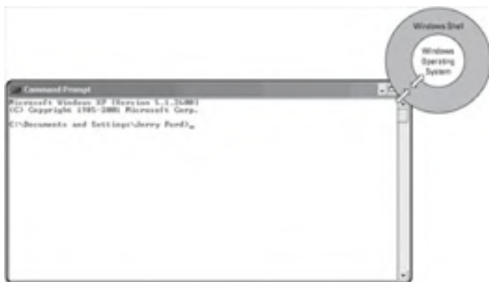
Figure 1.6: The Windows shell accepts input from the Windows command console and translates it into a format that can be used by the operating system.
