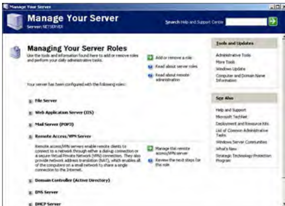
Figure 10.6. Manage Your Server enables you to configure a server for new roles, automatically adding new services (such as RRAS) and software as required.
