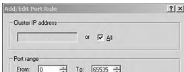
Figure 12.9. Each cluster can support multiple port ranges, as long as they don't overlap.
