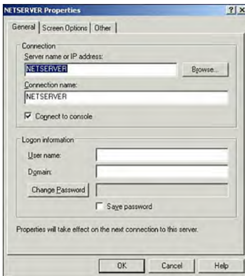
Figure 11.2. Connecting to the terminal server console session using the Remote Desktops console.
