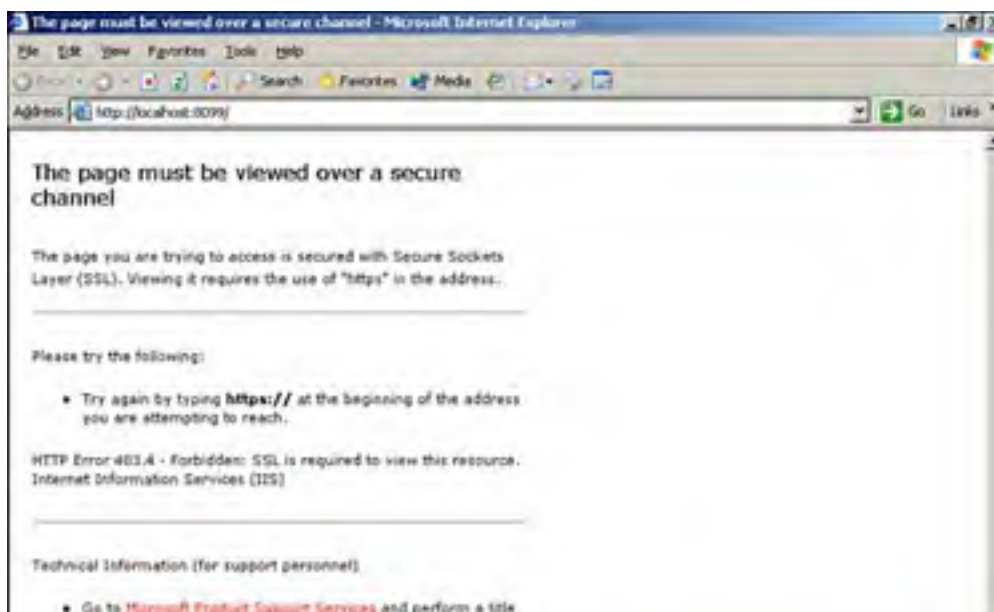
Figure 7.14. Notice that encryption could not be enforced here because the localhost URL was used rather than the server's actual name.
