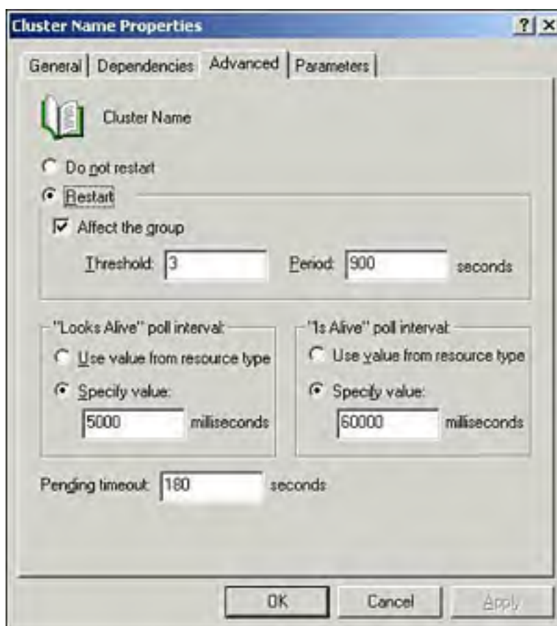
Figure 12.4. The default values for the advanced properties are sufficient in most environments.
