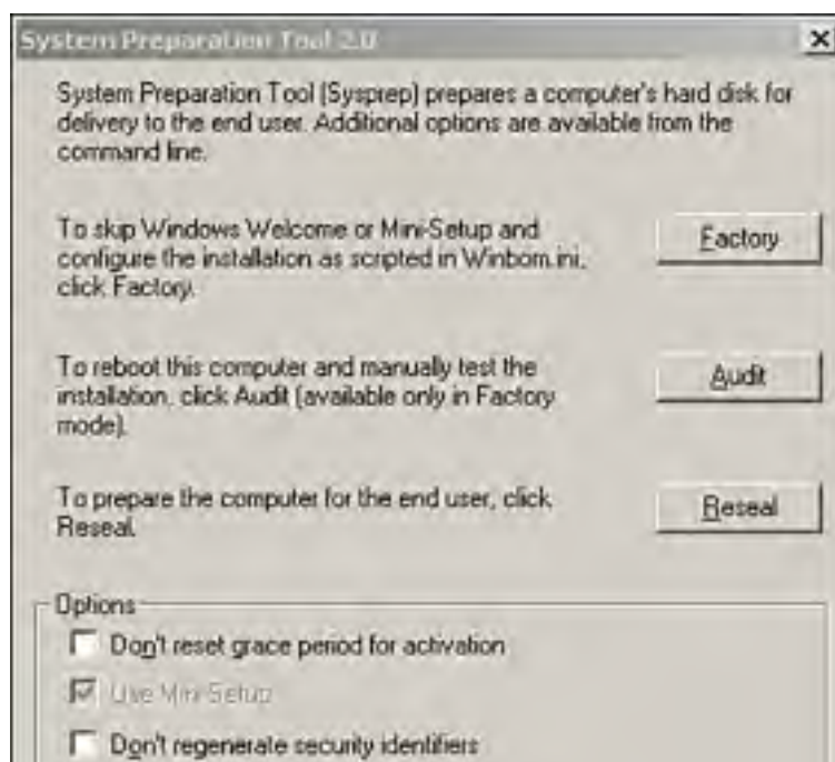
Figure 2.6. The new system preparation Factory Mode provides a means to install additional applications or drivers.
