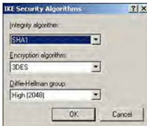
Figure 10.2. 2,048-bit encryption is roughly twice as strong as the strongest encryption previously available in Windows.
