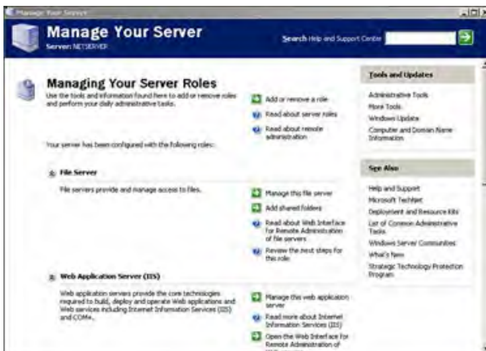
Figure 2.4. The Manage Your Server Wizard starts automatically after installation and enables the configuration of the server for its particular role.
