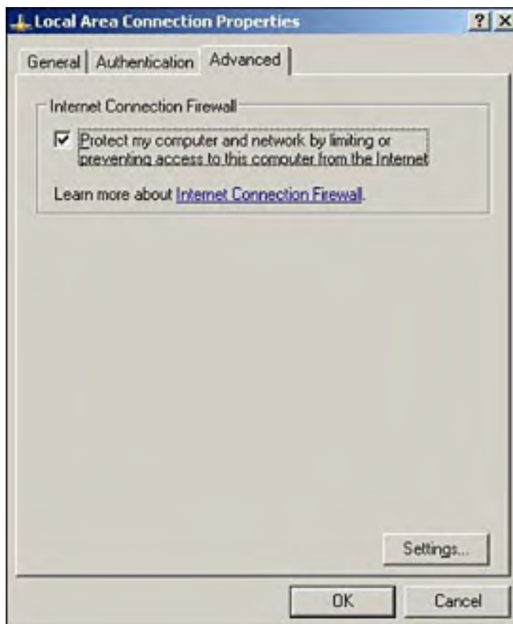
Figure 10.4. ICF can be used to protect any network connection on a server.
