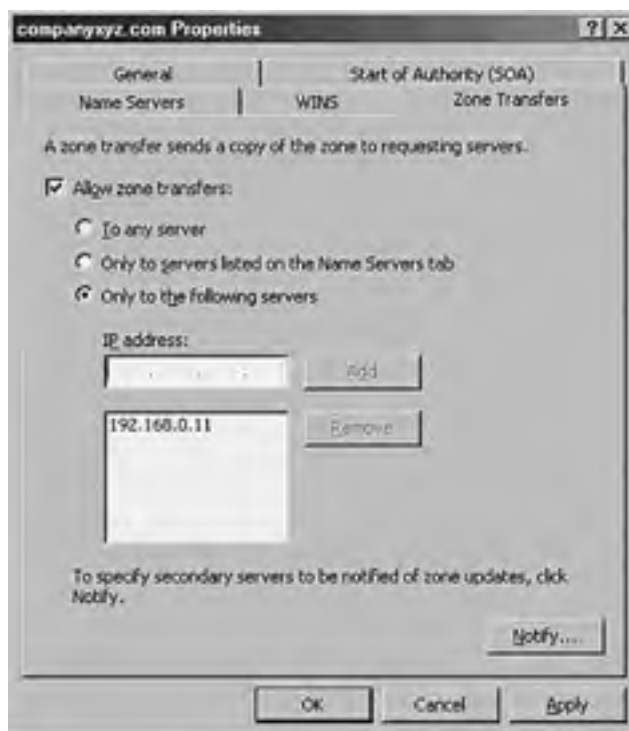
Figure 13.14. Setting up zone transfers.
