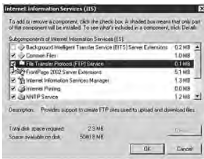
Figure 19.4. Installing FTP Services.
