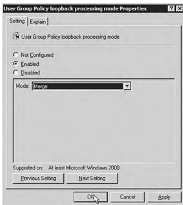
Figure 20.2. Enabling loopback processing mode.
