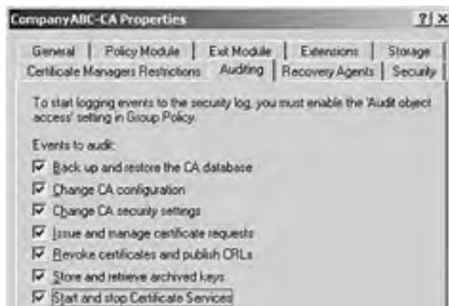
Figure 3.3. Enabling auditing on the Certification Authority.
