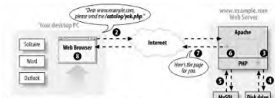
Figure 1-2. Client and server communication with PHP
