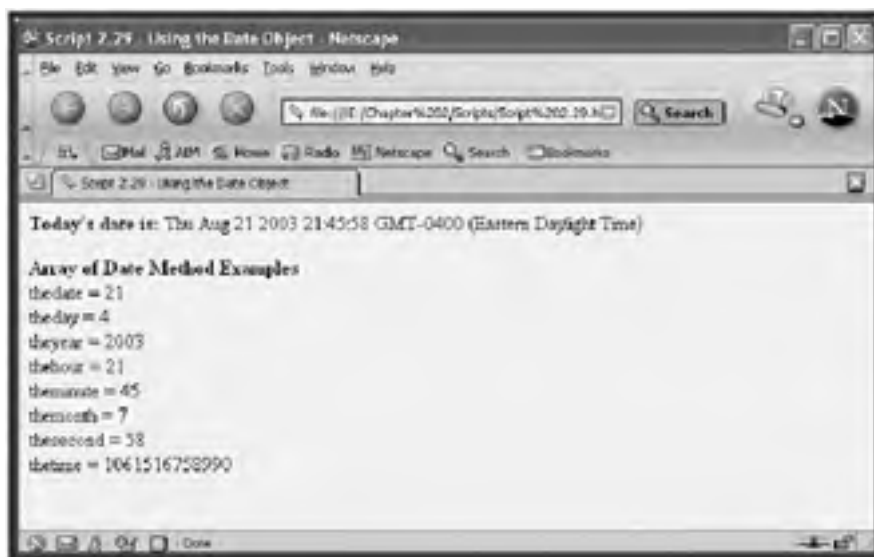
Figure 2.21. Using an array to store and display the results of data gathered using the Date object's methods
