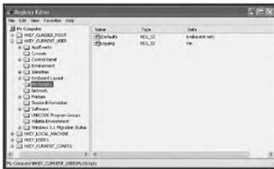
Figure 7.12. Verifying that the new registry subkey and value have been added under the HKEY_Current_User root key
