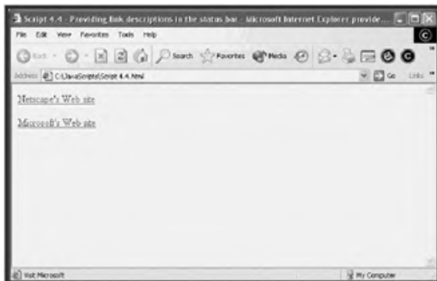
Figure 4.4. Posting descriptive messages on the browser's status bar when a visitor moves the mouse pointer over a link
