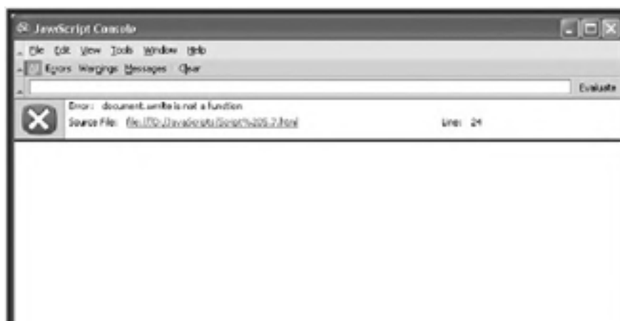
Figure 5.8. Netscape Communicator provides a built-in JavaScript debugger that allows you to view error messages and test command syntax.
