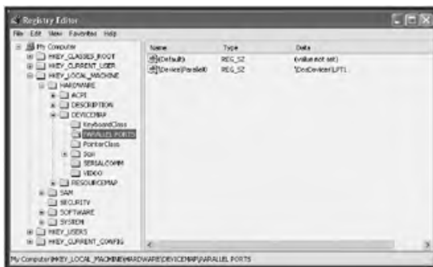
Figure 7.11. Viewing the structure of the Windows registry using the Regedit utility
