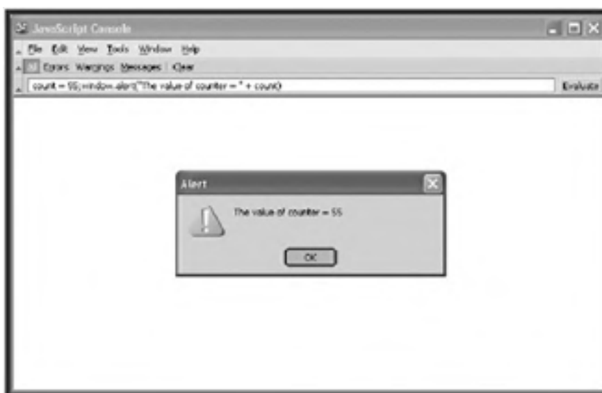
Figure 5.9. You can type JavaScript commands into the Netscape JavaScript Console to test their results.
