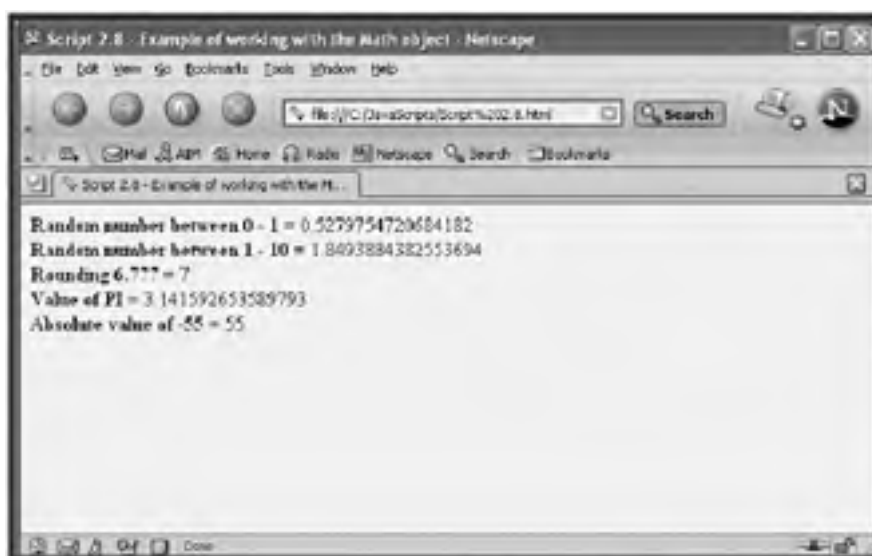
Figure 2.5. An example of how to access the Math object's properties and methods
