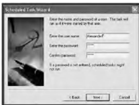
Figure 7.19. Setting up a scheduled task to run using a user account with sufficient security privileges
