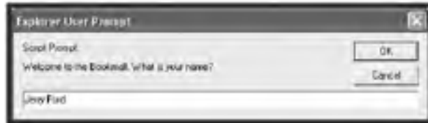
Figure 5.10. The document object's prompt() method provides the perfect tool for interactively collecting small pieces of information from visitors.
