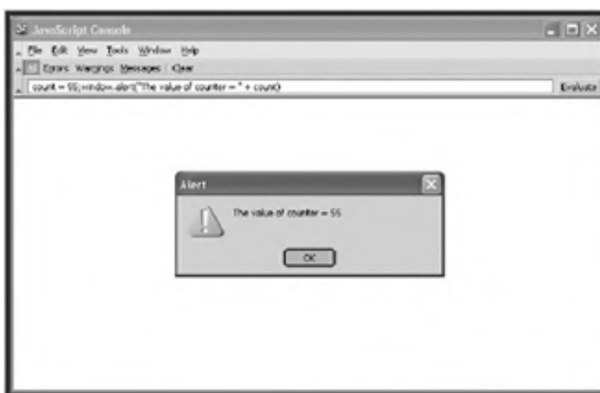
Figure 5.9. You can type JavaScript commands into the Netscape JavaScript Console to test their results.
