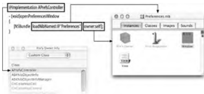
Figure 3-2. The File's Owner relationship between a nib and an object in an application
