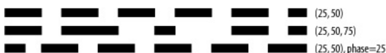
Figure 4-6. Line dash patterns: each line is 400 points long with a line thickness of 10 points
