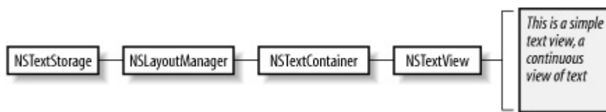
Figure 5-5. Configuration of the core classes for displaying a body of continuous text
