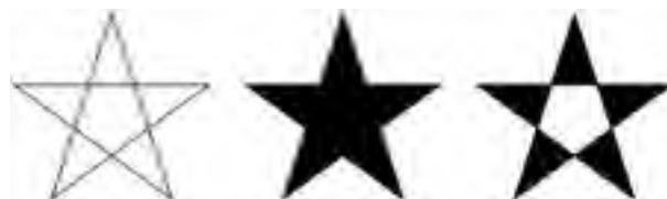
Figure 4-10. Stars illustrating (from left) the path with no fill, the default non-zero winding rule, and the even-odd winding rule
