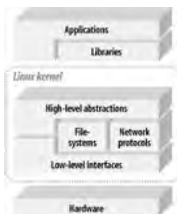
Figure 2-4. Architecture of a generic Linux system
