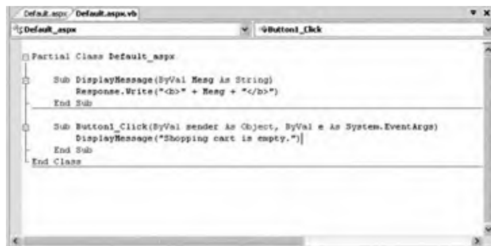
Figure 7-3 The message displayed by the DisplayMessage() subroutine is passed to this subroutine when the subroutine is called.
