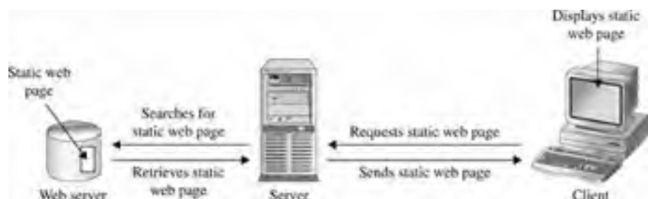
Figure 1-1 A static web page is stored on a web server and sent to a browser.
