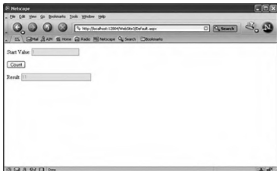
Figure 5-7 If the visitor enters 1 as the start value, the ASP.NET displays 11 as the result.
