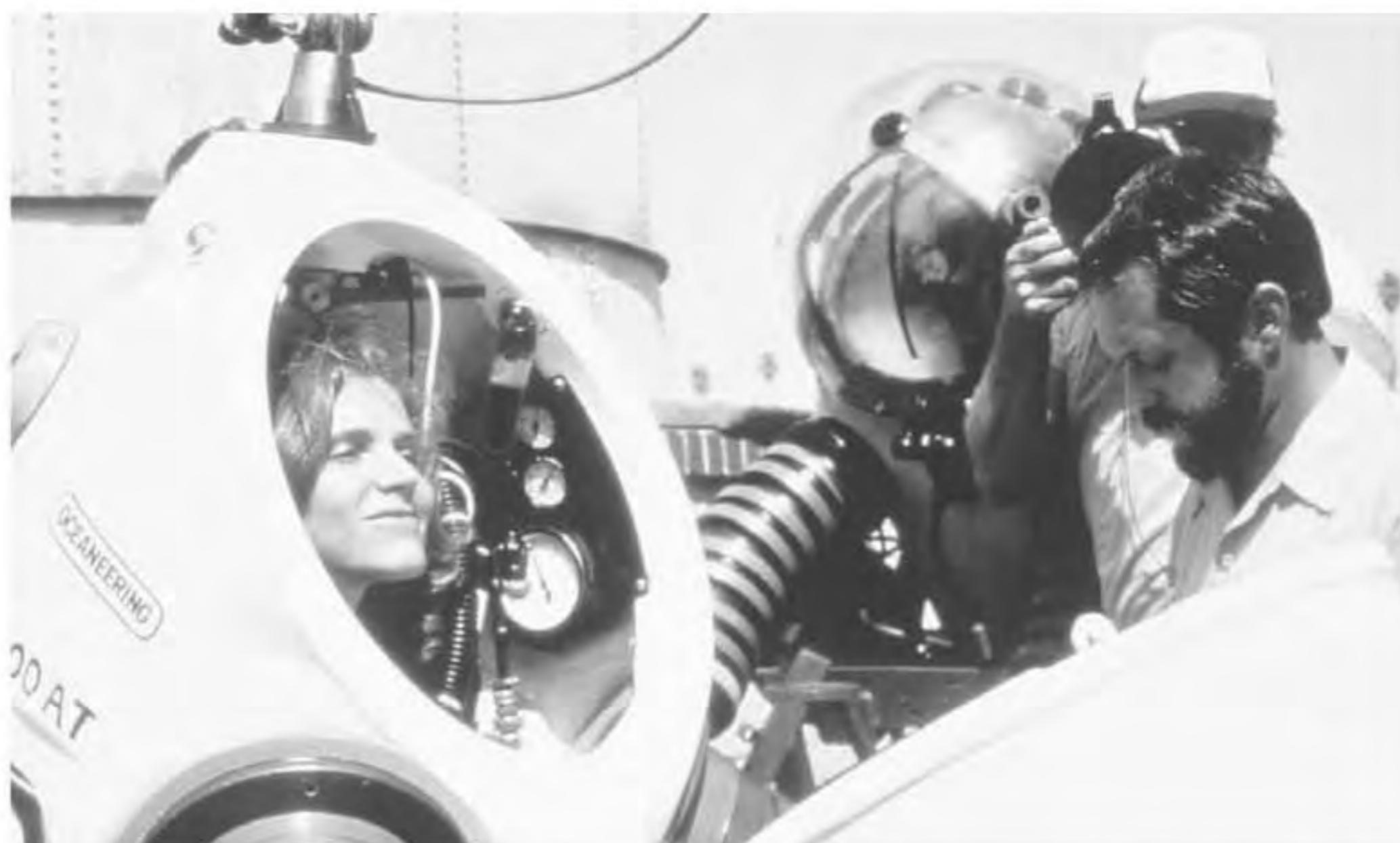
The JIM suit is a rigid suit that functions as a mini-submersible, carrying one person underwater for exploration. Here Dr. Sylvia Earle prepares for a dive. NOAA/OAR National Undersea Research Program
