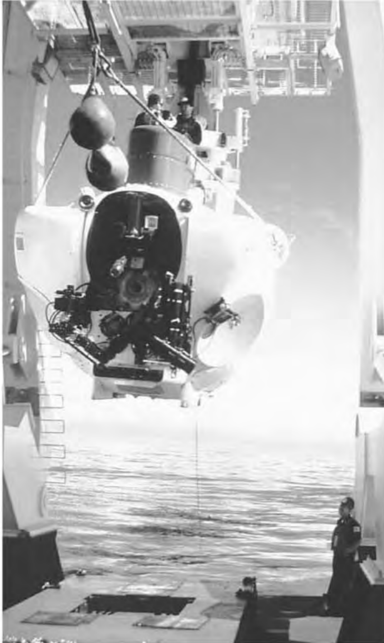
The DVS Turtle is a diving submersible; a state-of-the-art vessel that has allowed humans to investigate previously unseen areas of the ocean. Here it is being taken aboard the U.S. Navy support ship Laney Chouest in California's Monterey Bay. NOAA/OAR National Undersea Research Program; J. Butler
