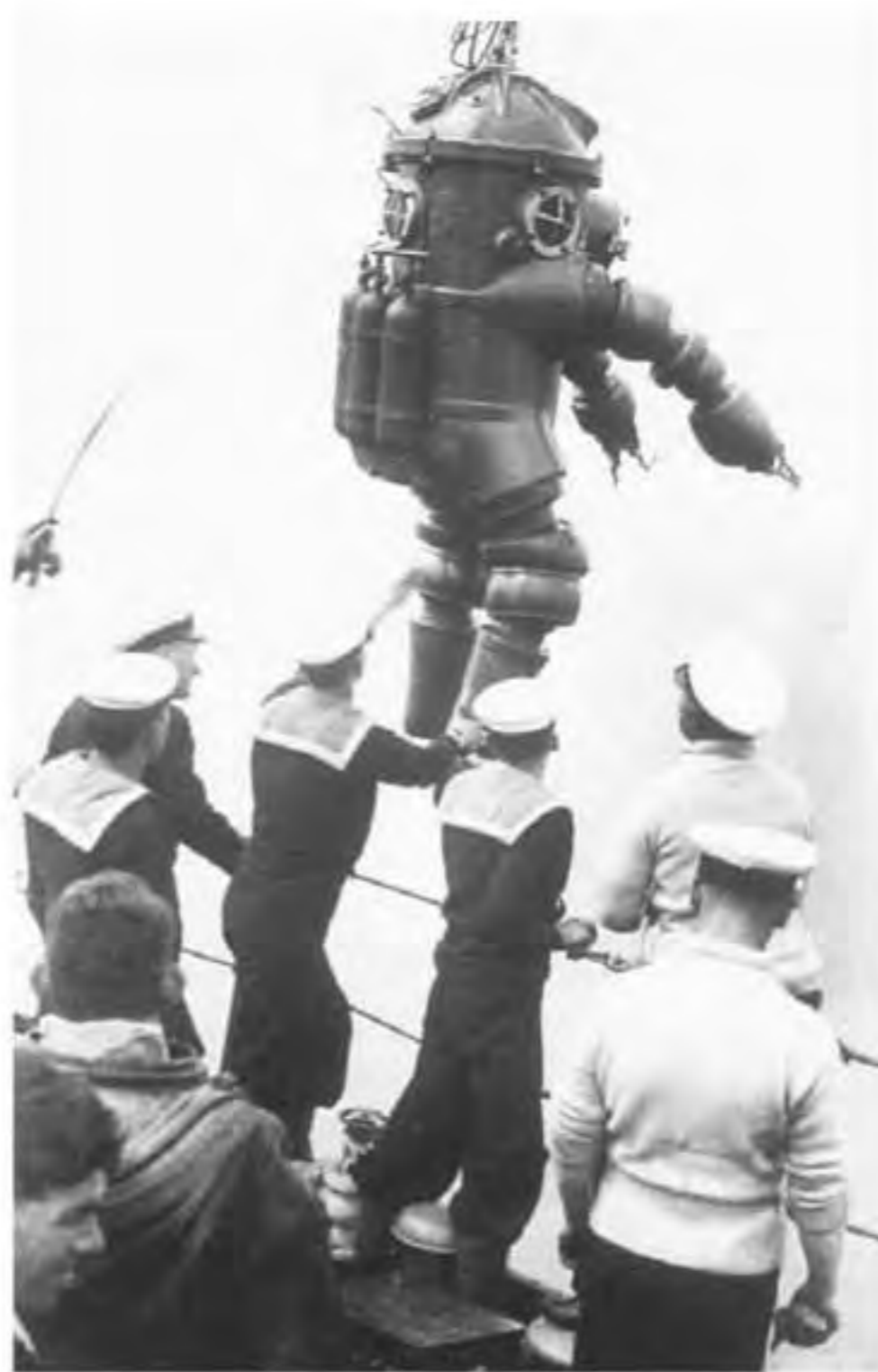
State of the art in 1915: The diving suit had come a long way since its invention in 1819. Here, the diver (outfitted in J. Peress' 1-atm dive suit) prepares to be lowered into the water to explore the wreckage of the Lusitania , the British luxury liner downed by the Germans during World War I. NOAA/OAR National Undersea Research Program
