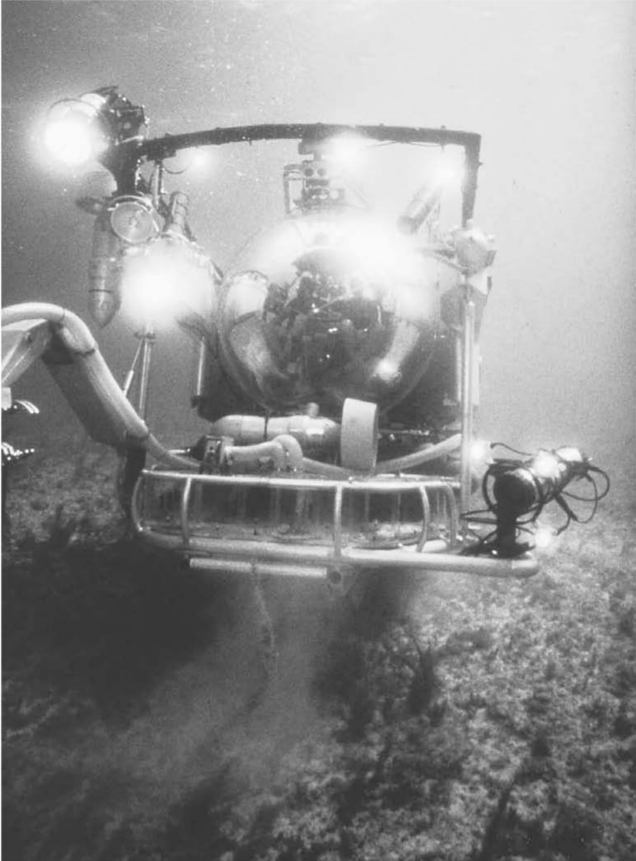
The Johnson Sea Link is an underwater sphere that allows pilot and observer to explore the depths. NOAA/OAR National Undersea Research Program
