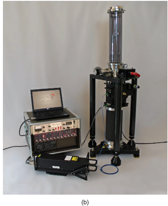
Figure 11.4 (a) Schematic of an Absolute Gravity meter indicating the dropping chamber and laser measurement system. (b) The Micro-g LaCoste FG5-X Absolute Gravity meter, the latest in the FG5 series. Pictures from Micro-g LaCoste.
