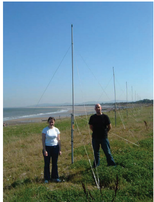
Figure 4.5 Surface currents measured by high-frequency radar over an offshore grid, by reflected Doppler shift analysis. Regional coverage of the approach to the port of Liverpool is obtained at lower cost than deploying in situ meters, as there are no moving parts or offshore installations. The image shows the aerial network of the radar site at Formby, UK, operated by the National Oceanography Centre. Photographs from John Howarth, NOC.
