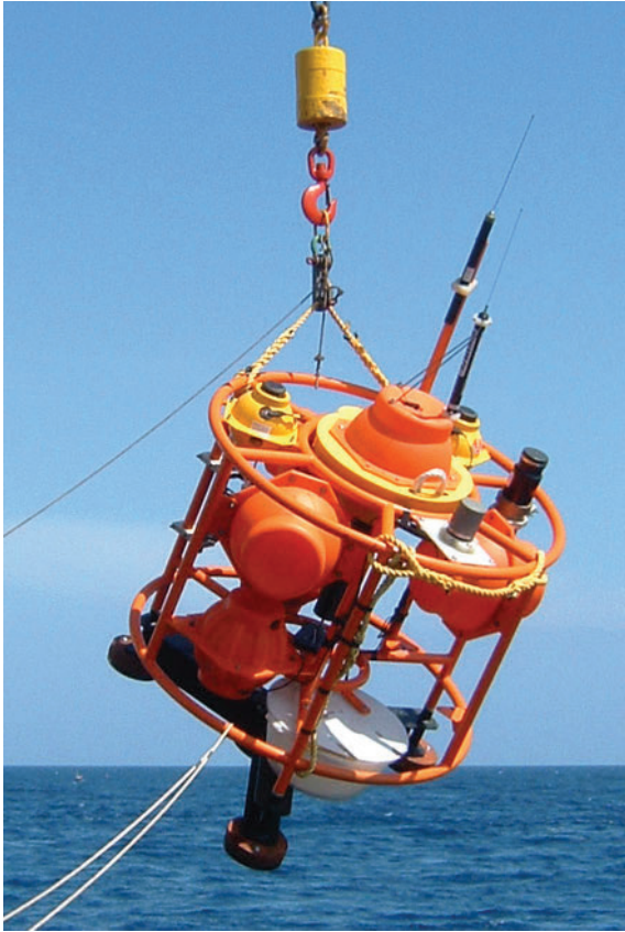
Figure 2.9 The National Oceanography Centre (NOC) deep-sea pressure gauge MYRTLE (Multi-Year Return Tide Level Equipment), ready for deployment. Photograph from NOC.
