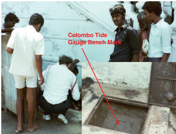
Figure 2.1 Locating a long-hidden Tide Gauge Bench Mark at Colombo, Sri Lanka. Photograph by David Pugh.
