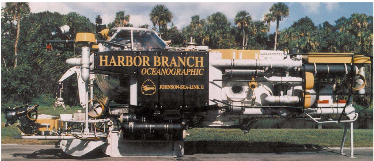
Figure 3 Johnson-Sea-Link I and II , 1971 and 1976. Owned and operated by Harbor Branch Oceanographic Institution. Length 7.2 m, beam 2.5 m, height 3.1 m, weight 10 400 kg, crew 2, observers 2, duration 3–5 hours.
