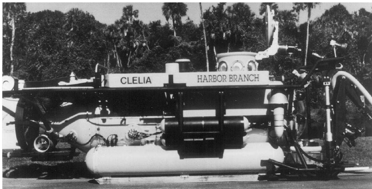
Figure 2 Perry PC 1204 Clelia , 1976. Owned and operated by Harbor Branch Oceanographic Institution. Length 6.7 m, beam 2.4 m, height 2.4 m, weight 8160 kg, crew 1, observers 2, duration 3–5 hours.
