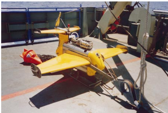
Figure 3 CSIRO (Australia) modified SeaSoar with a Sea-Bird Electronics Inc. conductivity, temperature and depth (CTD) instrument.
