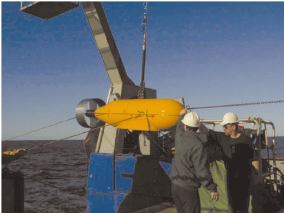
Figure 8 The CSIRO (Australia) multifrequency towed vehicle used for fish stock measurements. Note the ribbon-faired cable.
