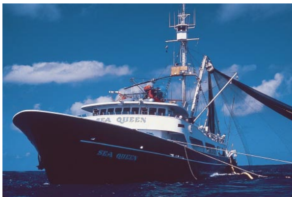
Figure 9 A modern purse-seine vessel of 1200 tonnes capacity; note the helicopter on board (courtesy of Dave Bratten, Inter-American Tropical Tuna Commission).
