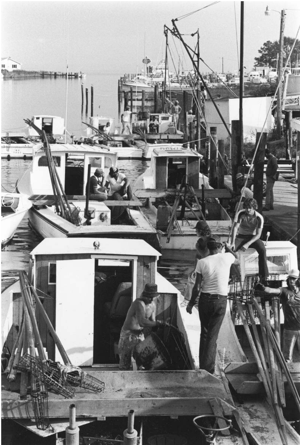
Figure 1 Post-harvest activities on shallow-draft tonging boats in Chesapeake Bay, Maryland, USA. Note the array of tongs, and the sorting or culling platform in the boat in the left foreground. (Photograph by Skip Brown, courtesy of Maryland Sea Grant.)
