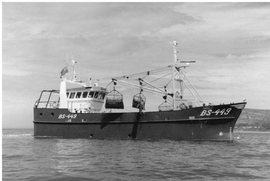
Figure 3 Harvesting vessel Mytilus with blue mussel dredges in Conwy Bay, Wales. (Photograph courtesy of Dr Eric Edwards.)
