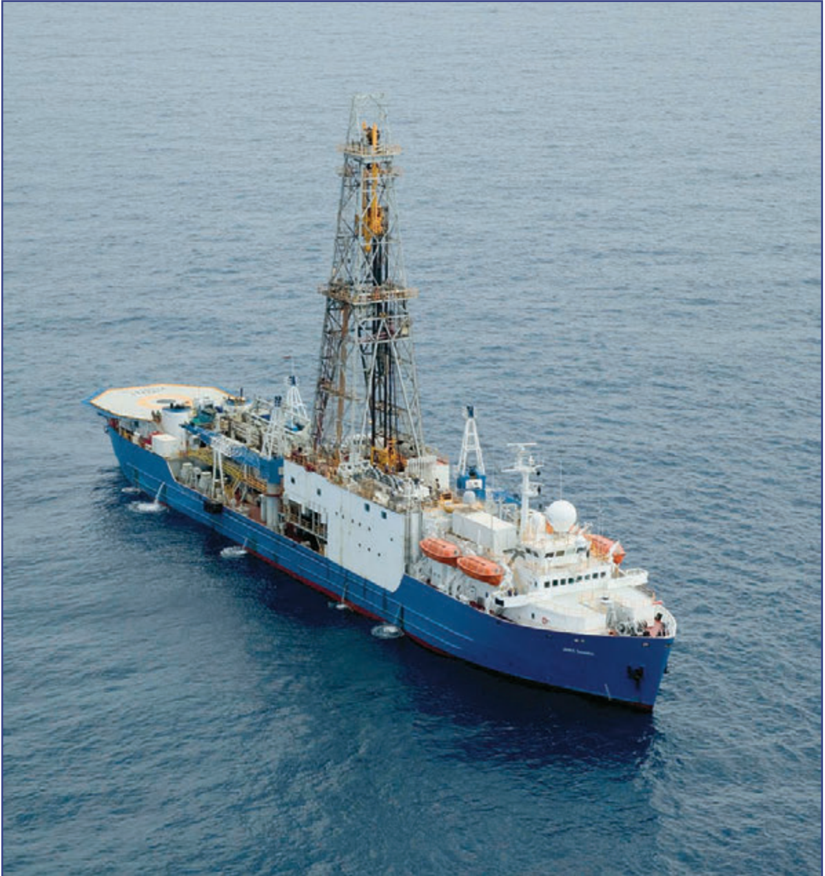
JOIDES Resolution is the research ship that was built in the 1970s for JOIDES (Joint Oceanographic Institutions for Deep Earth Sampling). It carries more than 5.5 miles (9 km) of drill pipe, allowing it to take samples from deep below the ocean floor. (Ocean Drilling Program, Texas A&M University)
