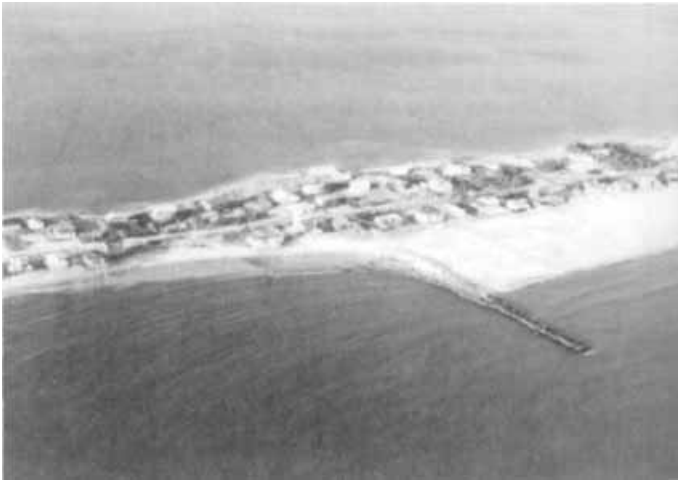
Figure 12.3 Groin field at Westhampton Beach, New York (from Nersesian, Kraus, and Carson 1992).
