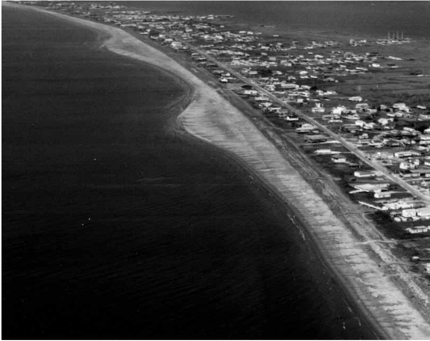
Figure 11.22 Salients on Grand Isle, Louisiana, due to offshore borrow pits (Combe and Soileau 1987).
