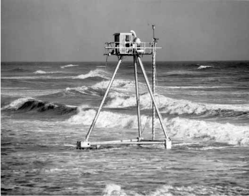
Figure 6.2 The Corps of Engineers' CRAB surveying vehicle (photograph courtesy of W.A. Birkemeier of the Field Research Facility, Duck, North Carolina).
