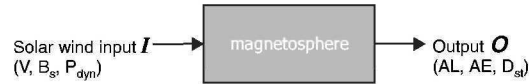
Figure 1. Representation of the magnetosphere in a data-derived approach. Input parameters are represented here by the solar wind speed v , southward component of the interplanetary magnetic field B_s , and dynamical pressure P_{dyn} , while the output is represented by the auroral indices AL and AE reflecting the substorm activity, and the disturbance storm-time index D_{st} .
