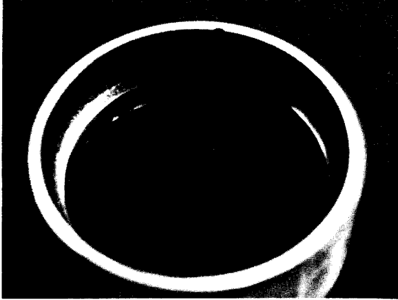
Fig. 5-36. Shallow Flaking on Outer Race of Bearing.
