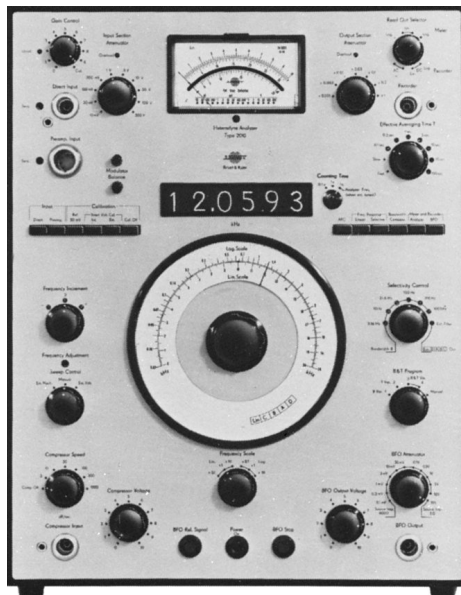
FIGURE 10.25 Heterodyne analyzer. (Courtesy of Bruel and Kjaer Instruments, Inc., Marlborough, MA.)
