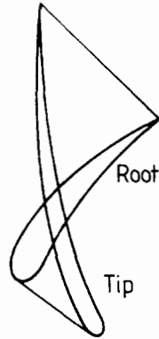
Figure 4.26 Root and tip sections of a typical compressor rotor blade illustrating the degree of twist.
