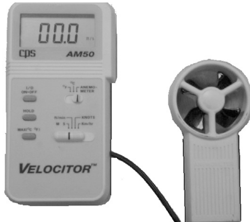
Figure 24.4 Vane anemometer (Business Edge)
