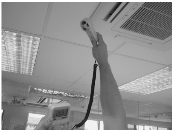
Figure 24.5 Vane anemometer in use (Business Edge)
