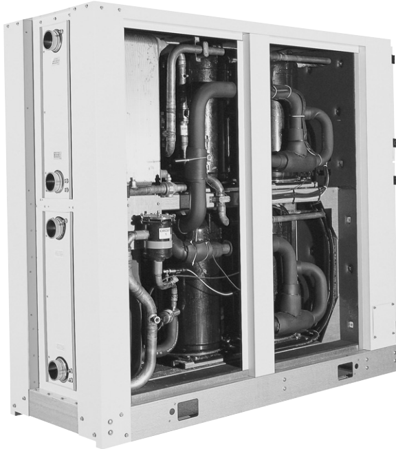
Figure 13.8 Water-cooled water chiller, nominal 250 kW capacity with two R407C refrigerant circuits, brazed plate heat exchangers (1 evaporator, 2 condensers), and multiple scroll compressors (Airedale)
