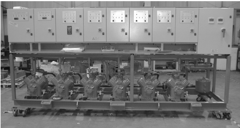
Figure 13.4 Semi-hermetic compressor pack (Arctic Circle)
