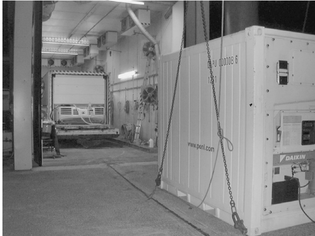
Figure 19.3 Test chamber capable of taking the largest permissible road vehicles (Cambridge Refrigeration Technology)
