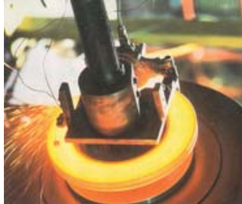
In a disc brake, hydraulic pressure forces friction pads to squeeze a metal disc that rotates on the same axle as the wheel. Here a disc brake is being tested.
