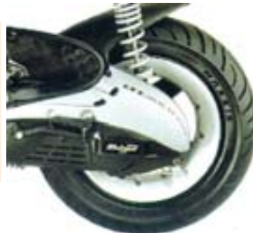
Helical spring suspension of a two-wheeler.
