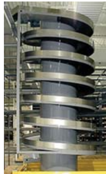
A spiral elevator conveyor for material handling.
