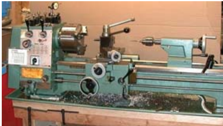
A lathe is a machine for shaping a piece of metal, by rotating it rapidly along its axis while pressing against a fixed cutting or abrading tool.
