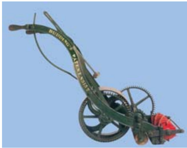
Lawn-mover is a combination of kinematic links.
