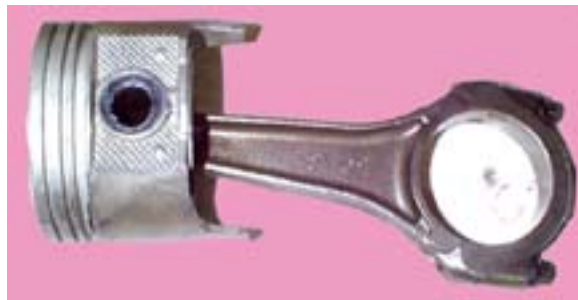
Piston and piston rod of an IC engine.
