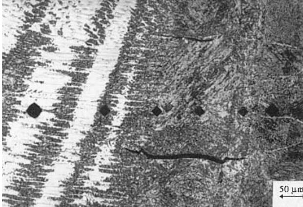
**Figure 10.7** Banding near fusion boundary of a carbon steel welded with an austenitic stainless steel filler metal. Reprinted from Rowe et al. (25). Courtesy of American Welding Society.
