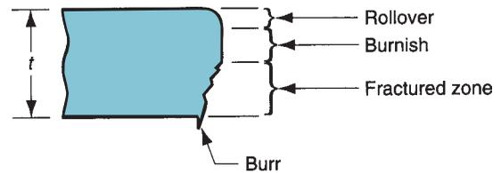
FIGURE 20.2 Characteristic sheared edges of the work.
