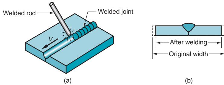
**FIGURE 30.31** (a) Butt welding two plates; (b) shrinkage across the width of the welded assembly; (c) transverse and longitudinal residual stress pattern; and (d) likely warping in the welded assembly.
