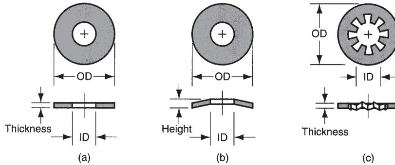
holes in the assembled parts, (3) increase spring tension, (4) protect part surfaces, (5) seal the joint, and (6) resist inadvertent unfastening [13]. Three washer types are illustrated in Figure 32.8.
