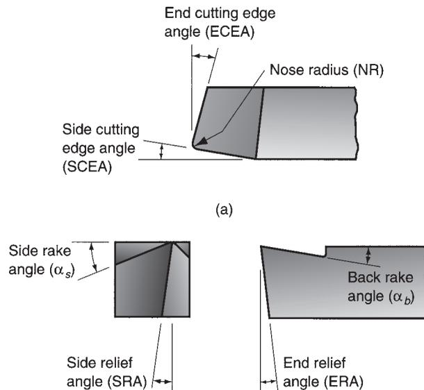
**FIGURE 23.7** (a) Seven elements of single-point tool geometry, and (b) the tool signature convention that defines the seven elements.
