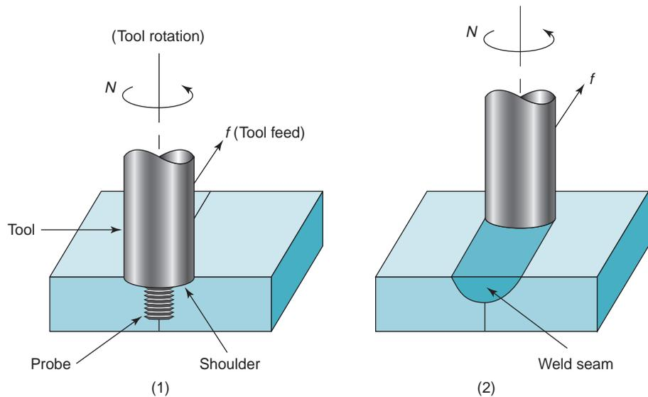
and mixing does not melt the metal but softens it to a highly plastic condition. As the tool is fed forward along the joint, the leading surface of the rotating probe forces the metal around it and into its wake, developing forces that forge the metal into a weld seam. The shoulder serves to constrain the plasticized metal flowing around the probe.
