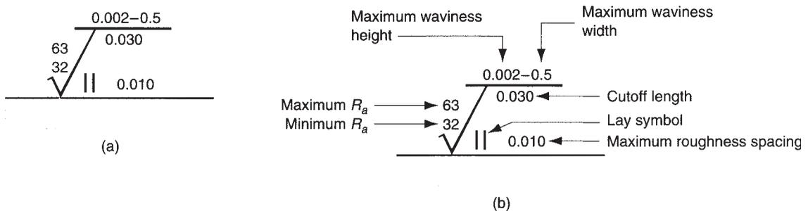
**FIGURE 5.16** Surface texture symbols in engineering drawings: (a) the symbol, and (b) symbol with identification labels. Values of  $R_a$  are given in microinches; units for other measures are given in inches. Designers do not always specify all of the parameters on engineering drawings.
