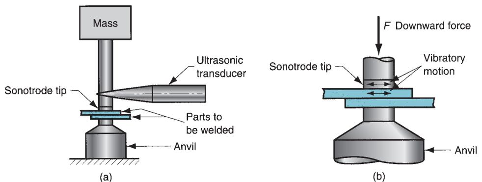
**FIGURE 30.30** Ultrasonic welding (USW): (a) general setup for a lap joint; and (b) close-up of weld area.
