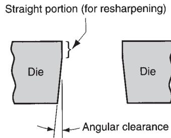
FIGURE 20.7 Angular clearance.
