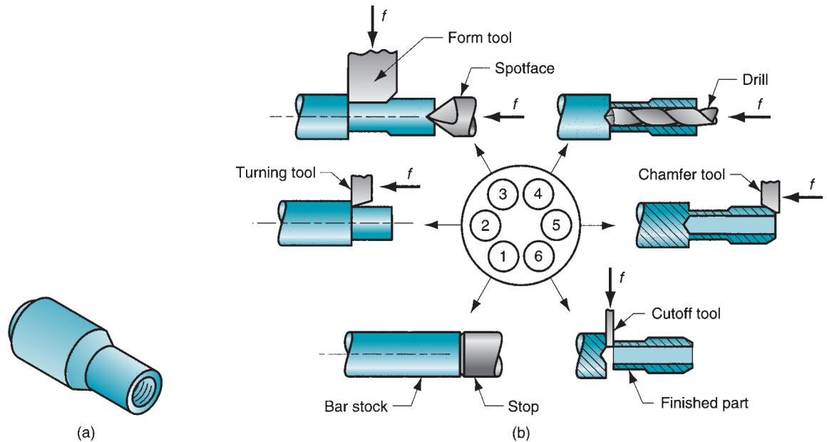
**FIGURE 22.9** (a) Type of part produced on a six-spindle automatic bar machine; and (b) sequence of operations to produce the part: (1) feed stock to stop, (2) turn main diameter, (3) form second diameter and spotface, (4) drill, (5) chamfer, and (6) cutoff.
