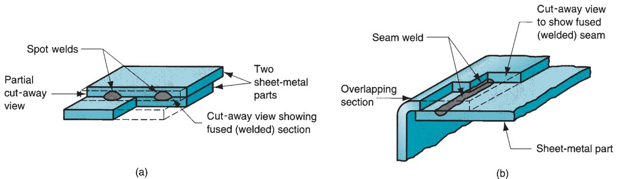
**FIGURE 29.6** (a) Spot weld; and (b) seam weld.
