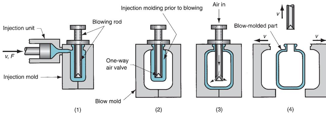
**FIGURE 13.32** Injection blow molding: (1) parison is injection molded around a blowing rod; (2) injection mold is opened and parison is transferred to a blow mold; (3) soft polymer is inflated to conform to the blow mold; and (4) blow mold is opened, and blown product is removed.
