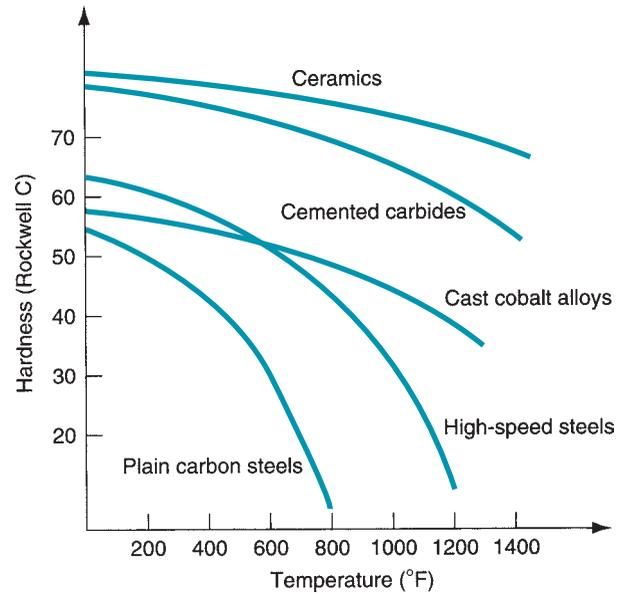
**FIGURE 23.6** Typical hot hardness relationships for selected tool materials. Plain carbon steel shows a rapid loss of hardness as temperature increases. High-speed steel is substantially better, whereas cemented carbides and ceramics are significantly harder at elevated temperatures.
