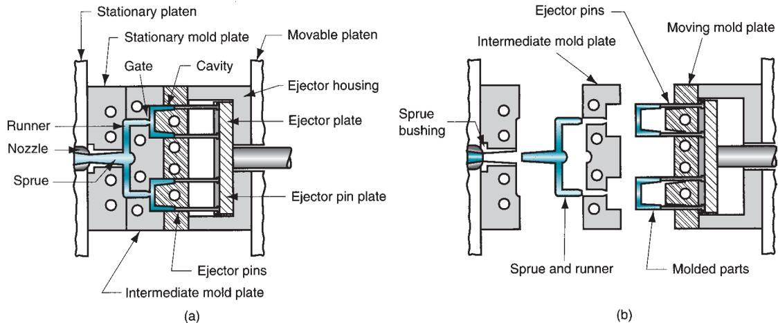
FIGURE 13.24 Three-plate mold: (a) closed, and (b) open.
