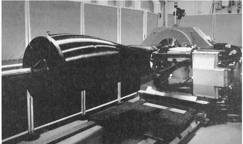
**FIGURE 15.10** Filament winding machine. (Courtesy of Cincinnati Milacron.)
