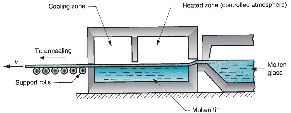
**FIGURE 12.7** The float process for producing sheet glass.
