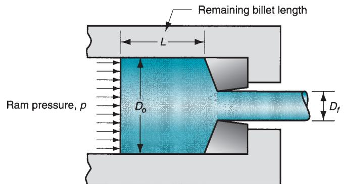
**FIGURE 19.33** Pressure and other variables in direct extrusion.
