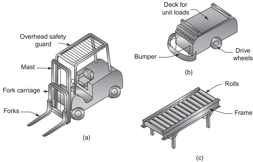
**FIGURE 39.1** Several types of material handling equipment: (a) fork lift truck, (b) automated guided vehicle, and (c) roller conveyor.
