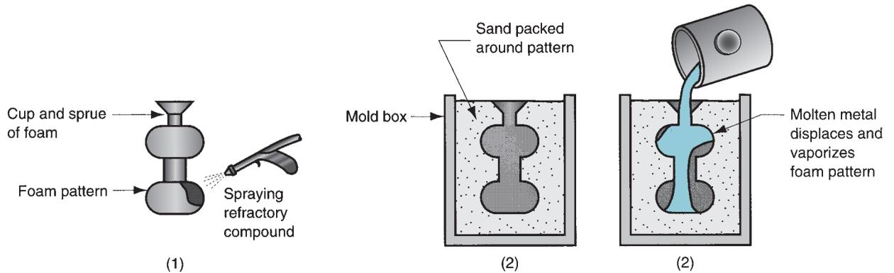
**FIGURE 11.7** Expanded polystyrene casting process: (1) pattern of polystyrene is coated with refractory compound; (2) foam pattern is placed in mold box, and sand is compacted around the pattern; and (3) molten metal is poured into the portion of the pattern that forms the pouring cup and sprue. As the metal enters the mold, the polystyrene foam is vaporized ahead of the advancing liquid, thus allowing the resulting mold cavity to be filled.
