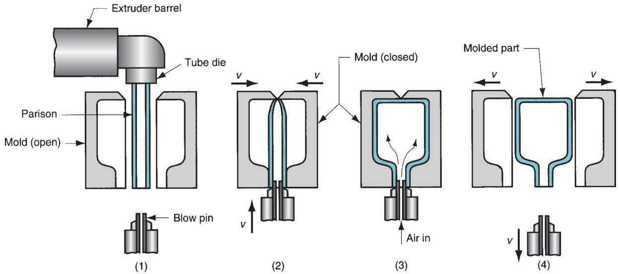
**FIGURE 13.30** Extrusion blow molding: (1) extrusion of parison; (2) parison is pinched at the top and sealed at the bottom around a metal blow pin as the two halves of the mold come together; (3) the tube is inflated so that it takes the shape of the mold cavity; and (4) mold is opened to remove the solidified part.
