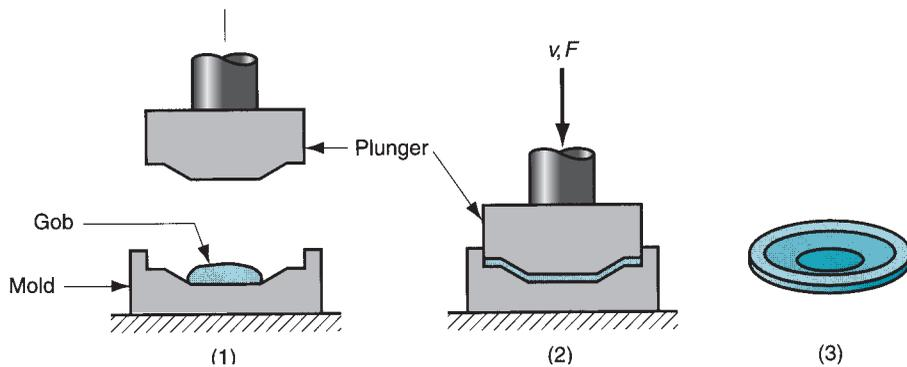
**FIGURE 12.3** Pressing of a flat glass piece: (1) a gob of glass fed into mold from the furnace; (2) pressing into shape by plunger; and (3) plunger is retracted and the finished product is removed. Symbols  $v$  and  $F$  indicate motion ( $v = \text{velocity}$ ) and applied force, respectively.
