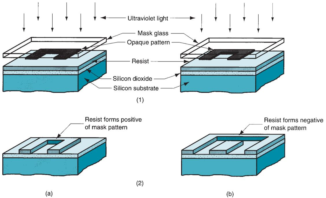
**FIGURE 34.9** Application of (a) positive resist and (b) negative resist in photolithography; for both types, the sequence shows: (1) exposure through the mask and (2) remaining resist after developing.
