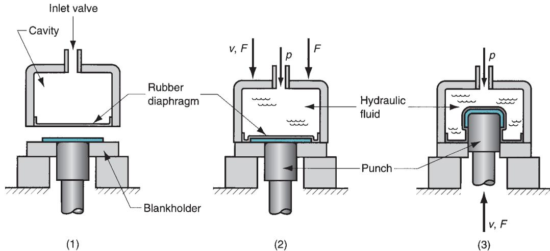
**FIGURE 20.29** Hydroform process: (1) start-up, no fluid in cavity; (2) press closed, cavity pressurized with hydraulic fluid; (3) punch pressed into work to form part. Symbols:  $v$  = velocity,  $F$  = applied force,  $p$  = hydraulic pressure.
