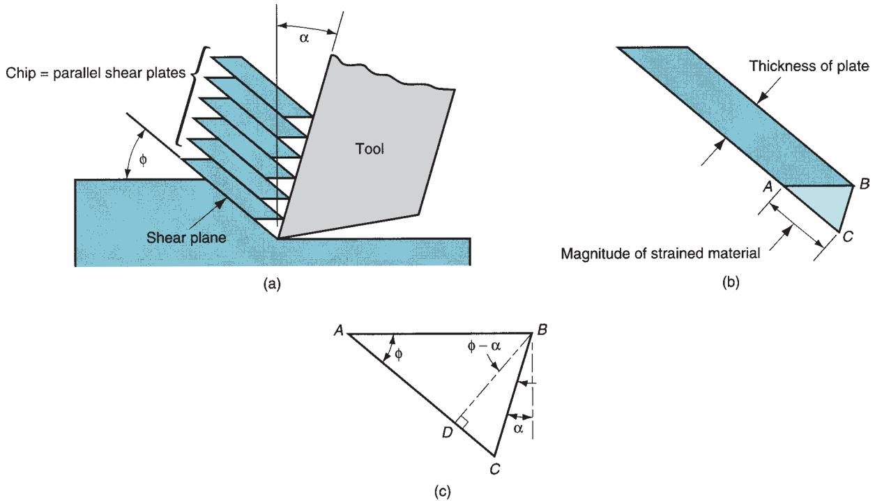
**FIGURE 21.7** Shear strain during chip formation: (a) chip formation depicted as a series of parallel plates sliding relative to each other; (b) one of the plates isolated to illustrate the definition of shear strain based on this parallel plate model; and (c) shear strain triangle used to derive Eq. (21.4).
