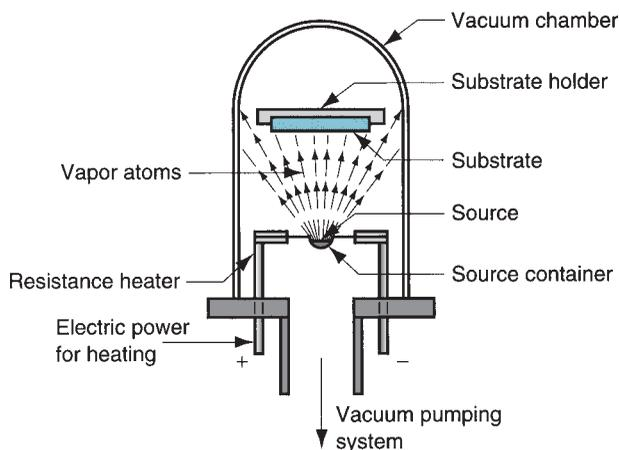
**FIGURE 28.6** Setup for vacuum evaporation physical vapor deposition.
