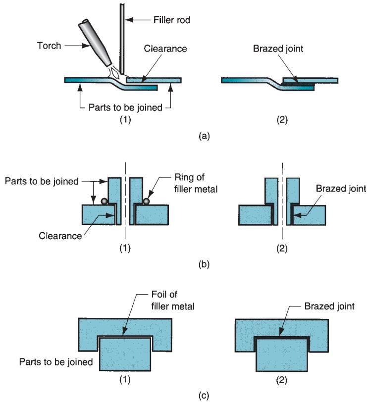
**FIGURE 31.4** Several techniques for applying filler metal in brazing: (a) torch and filler rod; (b) ring of filler metal at entrance of gap; and (c) foil of filler metal between flat part surfaces. Sequence: (1) before, and (2) after.
