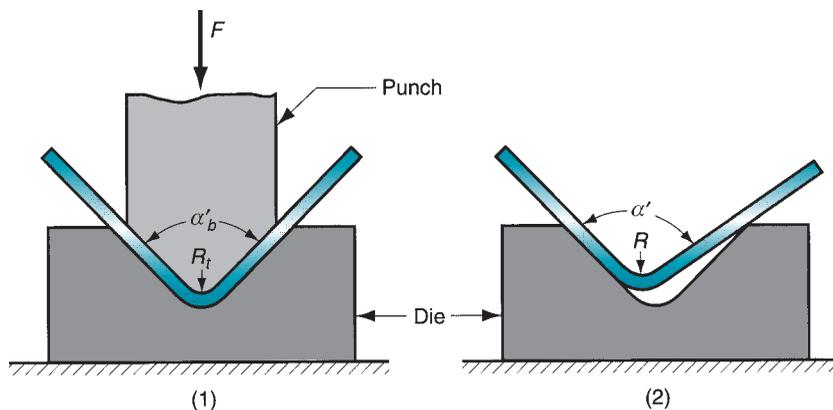
**FIGURE 20.13** Springback in bending shows itself as a decrease in bend angle and an increase in bend radius: (1) during the operation, the work is forced to take the radius  $R_t$  and included angle  $\alpha'_t$  = determined by the bending tool (punch in V-bending); (2) after the punch is removed, the work springs back to radius  $R$  and included angle  $\alpha'$ . Symbol:  $F$  = applied bending force.
