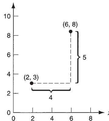
**FIGURE 38.8** Absolute vs. incremental positioning. The workhead is at point (2,3) and is to be moved to point (6,8). In absolute positioning, the move is specified by  $x = 6$ ,  $y = 8$ ; while in incremental positioning, the move is specified by  $x = 4$ ,  $y = 5$ .
