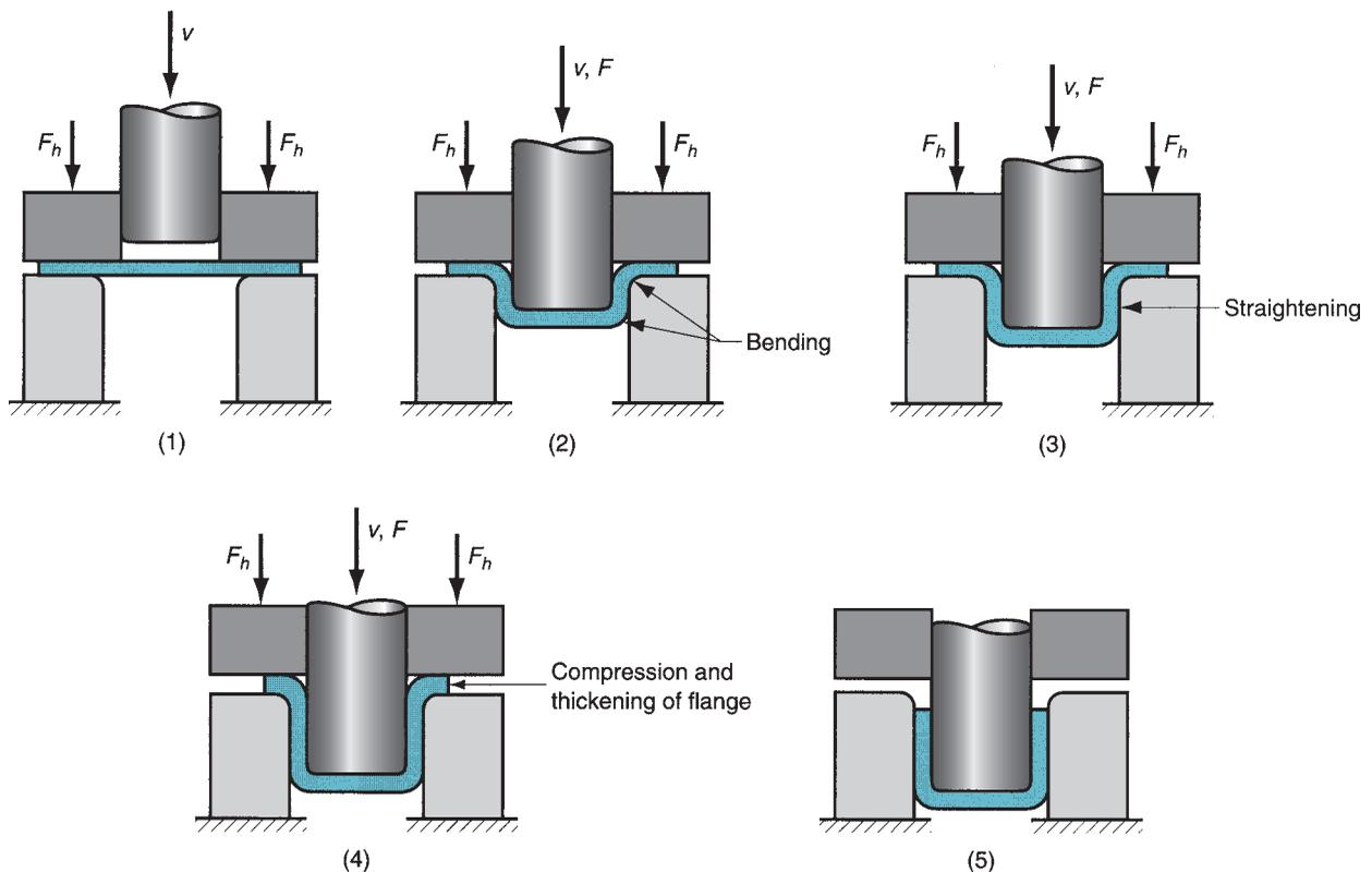
**FIGURE 20.20** Stages in deformation of the work in deep drawing: (1) punch makes initial contact with work, (2) bending, (3) straightening, (4) friction and compression, and (5) final cup shape showing effects of thinning in the cup walls. Symbols:  $v$  = motion of punch,  $F$  = punch force,  $F_h$  = blankholder force.
