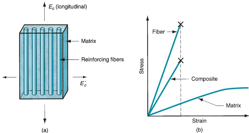
**FIGURE 9.5** (a) Model of a fiber-reinforced composite material showing direction in which elastic modulus is being estimated by the rule of mixtures. (b) Stress-strain relationships for the composite material and its constituents. The fiber is stiff but brittle, while the matrix (commonly a polymer) is soft but ductile. The composite's modulus is a weighted average of its components' moduli. But when the reinforcing fibers fail, the composite does likewise.
