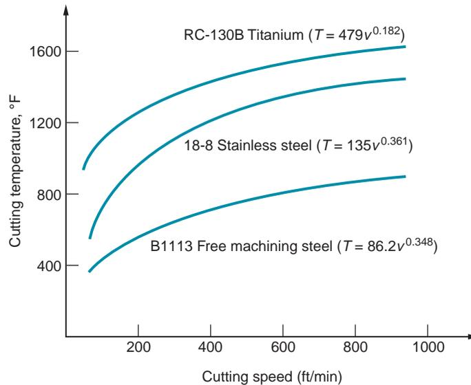
thermocouple junction. By properly connecting electrical leads to the tool and work-part (which is connected to the chip), the voltage generated at the tool–chip interface during cutting can be monitored using a recording potentiometer or other appropriate data-collection device. The voltage output of the tool–chip thermocouple (measured in mV) can be converted into the corresponding temperature value by means of calibration equations for the particular tool–work combination.
