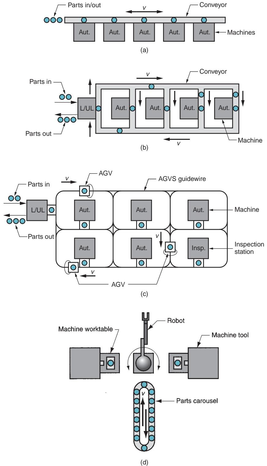
**FIGURE 39.11** Four of the five FMS layout types: (a) in-line, (b) ladder, (c) open field, and (d) robot-centered cell. Key: Aut = automated station; L/UL = load/unload station; Insp = inspection station; AGV = automated guided vehicle; AGVS = automated guided vehicle system.
