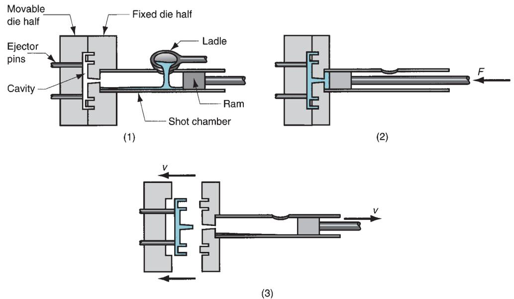
**FIGURE 11.14** Cycle in cold-chamber casting: (1) with die closed and ram withdrawn, molten metal is poured into the chamber; (2) ram forces metal to flow into die, maintaining pressure during cooling and solidification; and (3) ram is withdrawn, die is opened, and part is ejected. (Gating system is simplified.)
