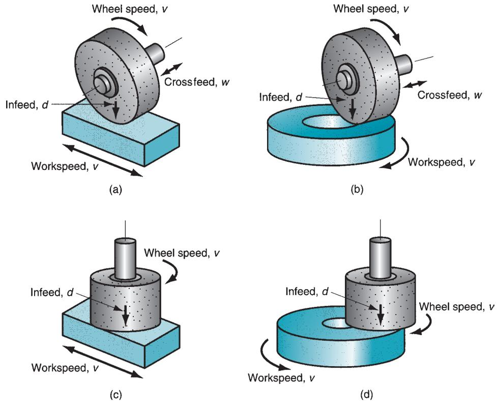
**FIGURE 25.7** Four types of surface grinding: (a) horizontal spindle with reciprocating worktable, (b) horizontal spindle with rotating worktable, (c) vertical spindle with reciprocating worktable, and (d) vertical spindle with rotating worktable.
