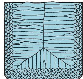
**FIGURE 10.5** Characteristic grain structure in a casting of a pure metal, showing randomly oriented grains of small size near the mold wall, and large columnar grains oriented toward the center of the casting.
