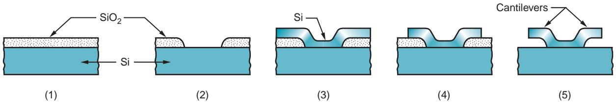
**FIGURE 36.10** Surface micromachining to form cantilevers: (1) on the silicon substrate is formed a silicon dioxide layer, whose thickness will determine the gap size for the cantilevered member; (2) portions of the  $\text{SiO}_2$  layer are etched using lithography; (3) a polysilicon layer is applied; (4) portions of the polysilicon layer are etched using lithography; and (5) the  $\text{SiO}_2$  layer beneath the cantilevers is selectively etched.
