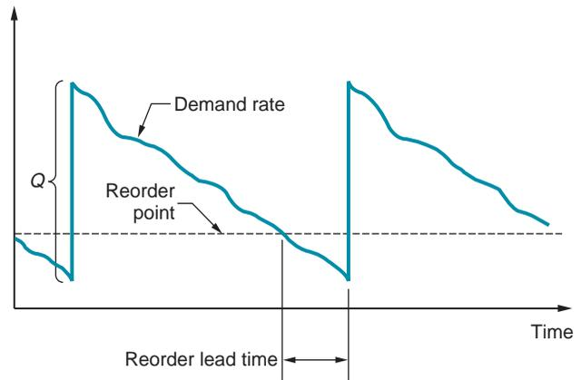
**FIGURE 41.3** Operation of a reorder point inventory system.
