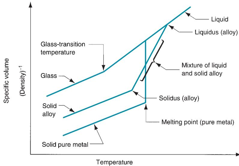
**FIGURE 4.1** Changes in volume per unit weight ( $1/\text{density}$ ) as a function of temperature for a hypothetical pure metal, alloy, and glass; all exhibiting similar thermal expansion and melting characteristics.
