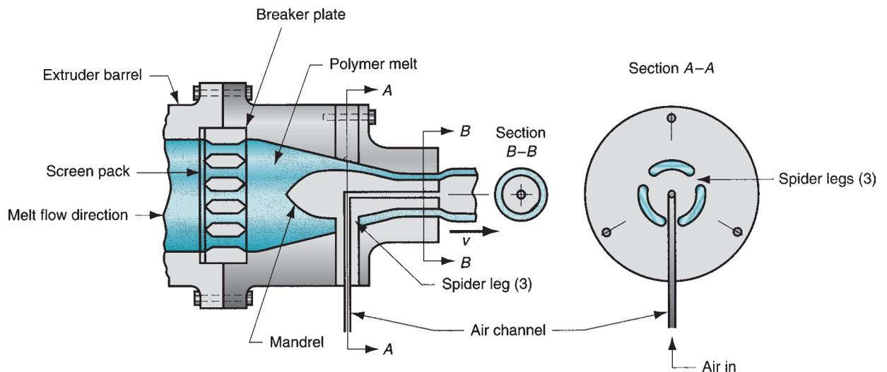
**FIGURE 13.10** Side view cross section of extrusion die for shaping hollow cross sections such as tubes and pipes; Section A-A is a front view cross section showing how the mandrel is held in place; Section B-B shows the tubular cross section just prior to exiting the die; die swell causes an enlargement of the diameter. (Some die construction details are simplified.)
