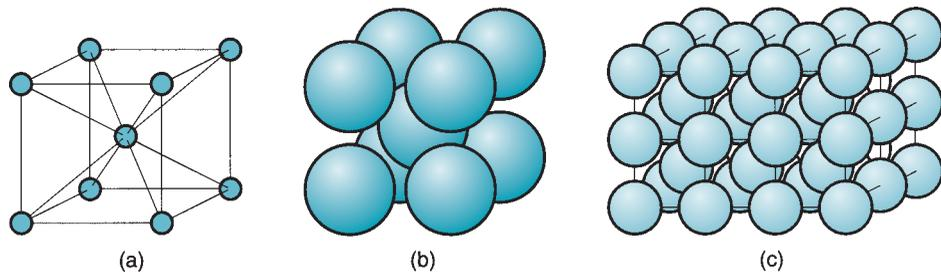
**FIGURE 2.7** Body-centered cubic (BCC) crystal structure: (a) unit cell, with atoms indicated as point locations in a three-dimensional axis system; (b) unit cell model showing closely packed atoms (sometimes called the hard-ball model); and (c) repeated pattern of the BCC structure.
