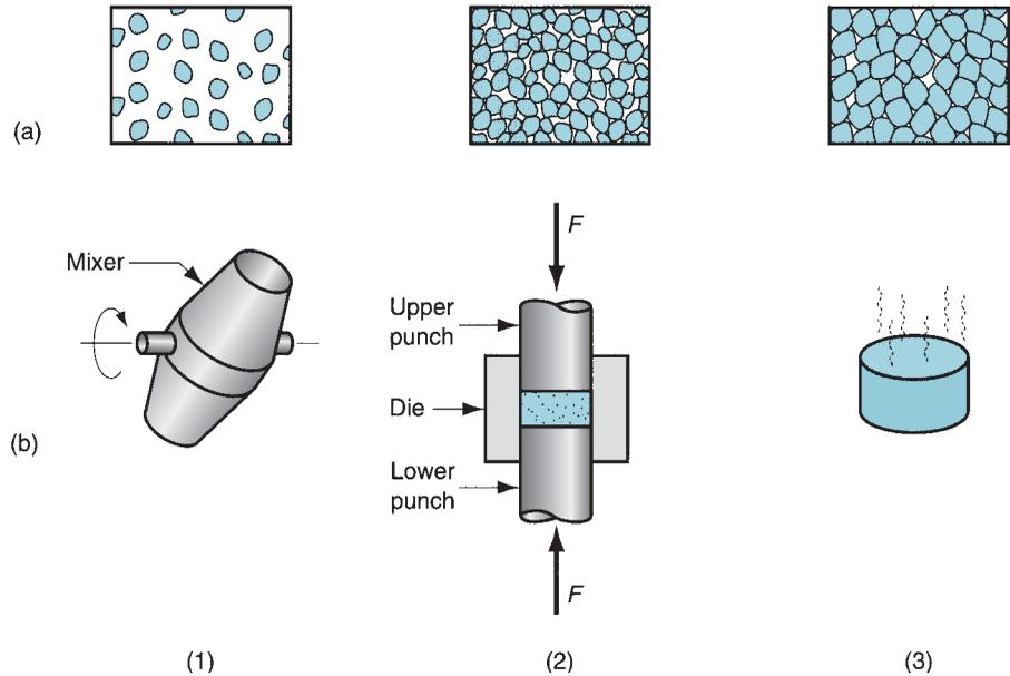
**FIGURE 16.7** The conventional powder metallurgy production sequence: (1) blending, (2) compacting, and (3) sintering; (a) shows the condition of the particles, whereas (b) shows the operation and/or workpart during the sequence.
