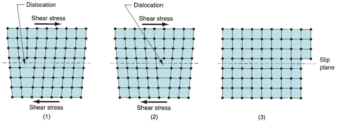
**FIGURE 2.12** Effect of dislocations in the lattice structure under stress. In the series of diagrams, the movement of the dislocation allows deformation to occur under a lower stress than in a perfect lattice.
