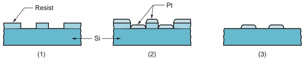
**FIGURE 36.11** The lift-off technique: (1) resist is applied to substrate and structured by lithography; (2) platinum is deposited onto surfaces; and (3) resist is removed, taking with it the platinum on its surface but leaving the desired platinum microstructure.
