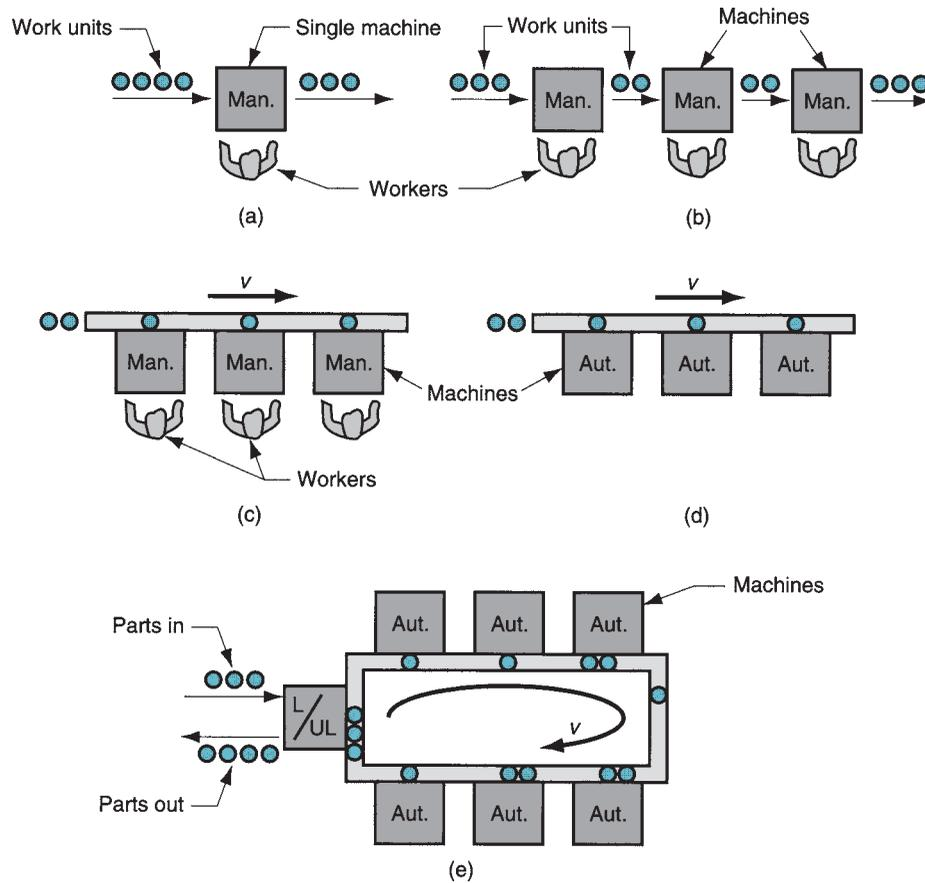
**FIGURE 39.10** Types of group technology machine cells: (a) single machine, (b) multiple machines with manual handling, (c) multiple machines with mechanized handling, (d) flexible manufacturing cell, and (e) flexible manufacturing system. Key: Man = manual operation; Aut = automated station.
