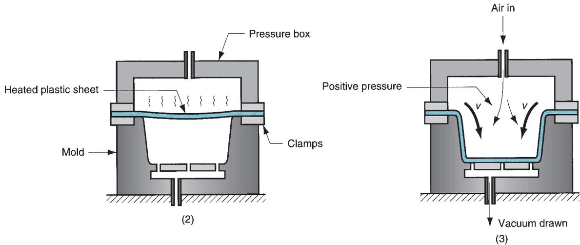
**FIGURE 13.36** Pressure thermoforming. The sequence is similar to the previous figure, the difference being: (2) sheet is placed over a mold cavity; and (3) positive pressure forces the sheet into the cavity.
