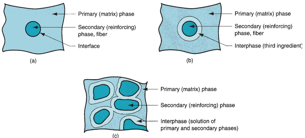
**FIGURE 9.4** Interfaces and interphases between phases in a composite material: (a) direct bonding between primary and secondary phases; (b) addition of a third ingredient to bond the primary and secondary phases and form an interphase; and (c) formation of an interphase by solution of the primary and secondary phases at their boundary.
