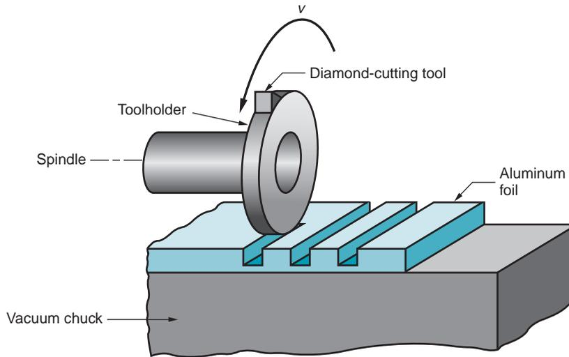
**FIGURE 36.15** Ultra-high-precision milling of grooves in aluminum foil.
