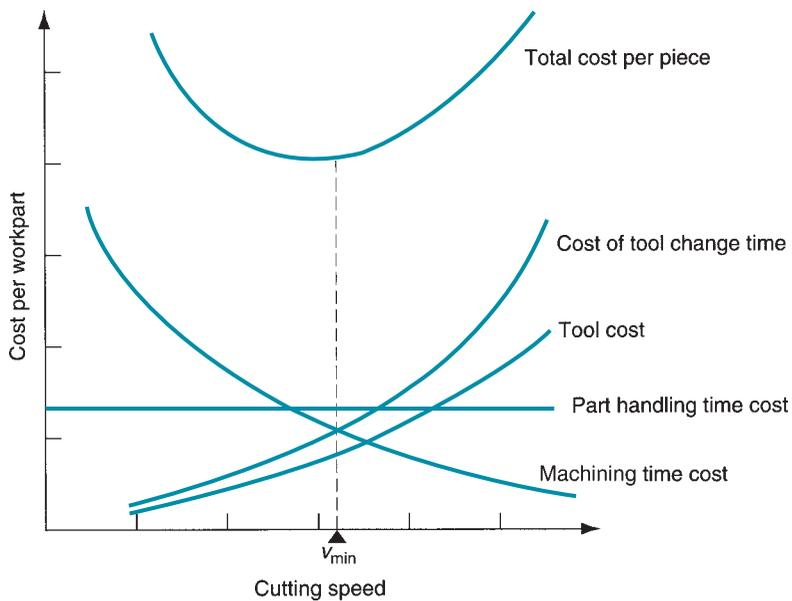
**FIGURE 24.4** Cost components in a machining operation plotted as a function of cutting speed. Total cost per piece is minimized at a certain value of cutting speed. This is the speed for minimum cost per piece.
