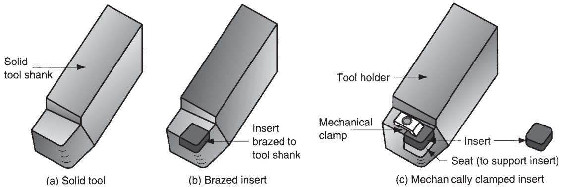
**FIGURE 23.9** Three ways of holding and presenting the cutting edge for a single-point tool: (a) solid tool, typical of HSS; (b) brazed insert, one way of holding a cemented carbide insert; and (c) mechanically clamped insert, used for cemented carbides, ceramics, and other very hard tool materials.
