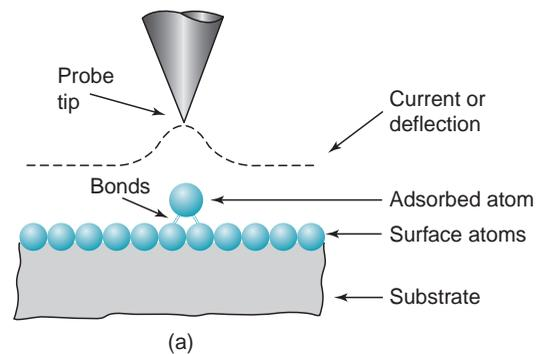
**FIGURE 37.4** Manipulation of individual atoms by means of scanning tunneling microscopy techniques: (a) probe tip is maintained a distance from the surface that is sufficient to avoid disturbance of adsorbed atom and (b) probe tip is moved closer to the surface so that the adsorbed atom is attracted to the tip.
