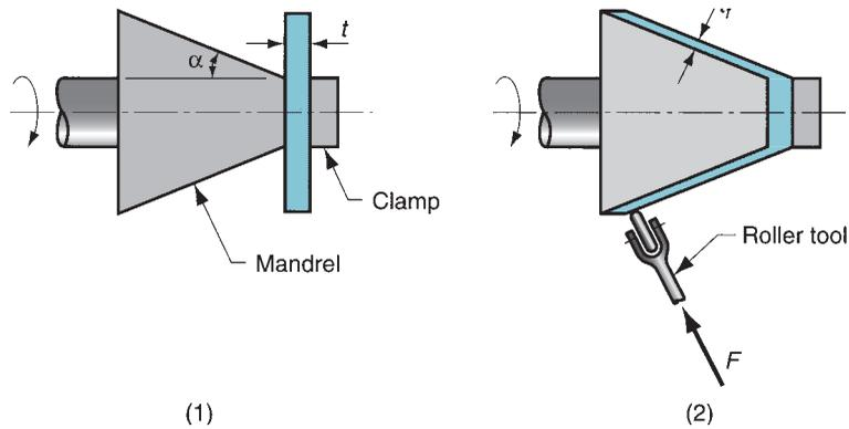
**FIGURE 20.43** Shear spinning: (1) setup and (2) completion of process.
