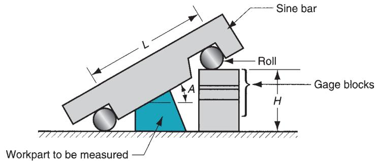
**FIGURE 5.11** Setup for using a sine bar.
