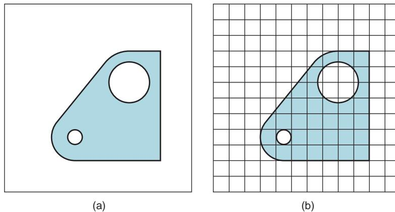
**FIGURE 42.9** Image acquisition and digitizing: (a) the scene consists of a dark-colored part against a light background; (b) a  $12 \times 12$  matrix of pixels imposed on the scene.
