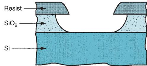
**FIGURE 34.13** Profile of a properly etched layer.
