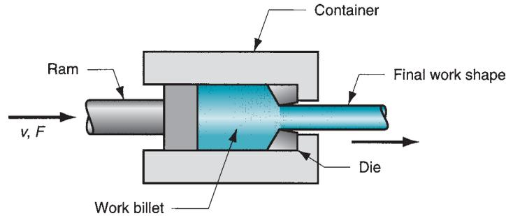
**FIGURE 19.30** Direct extrusion.
