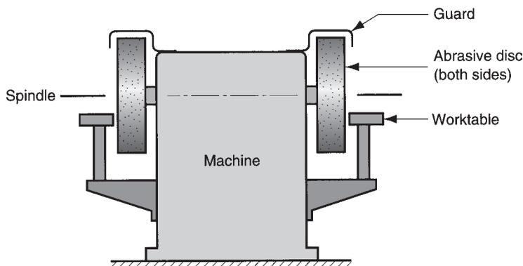
**FIGURE 25.14** Typical configuration of a disk grinder.
