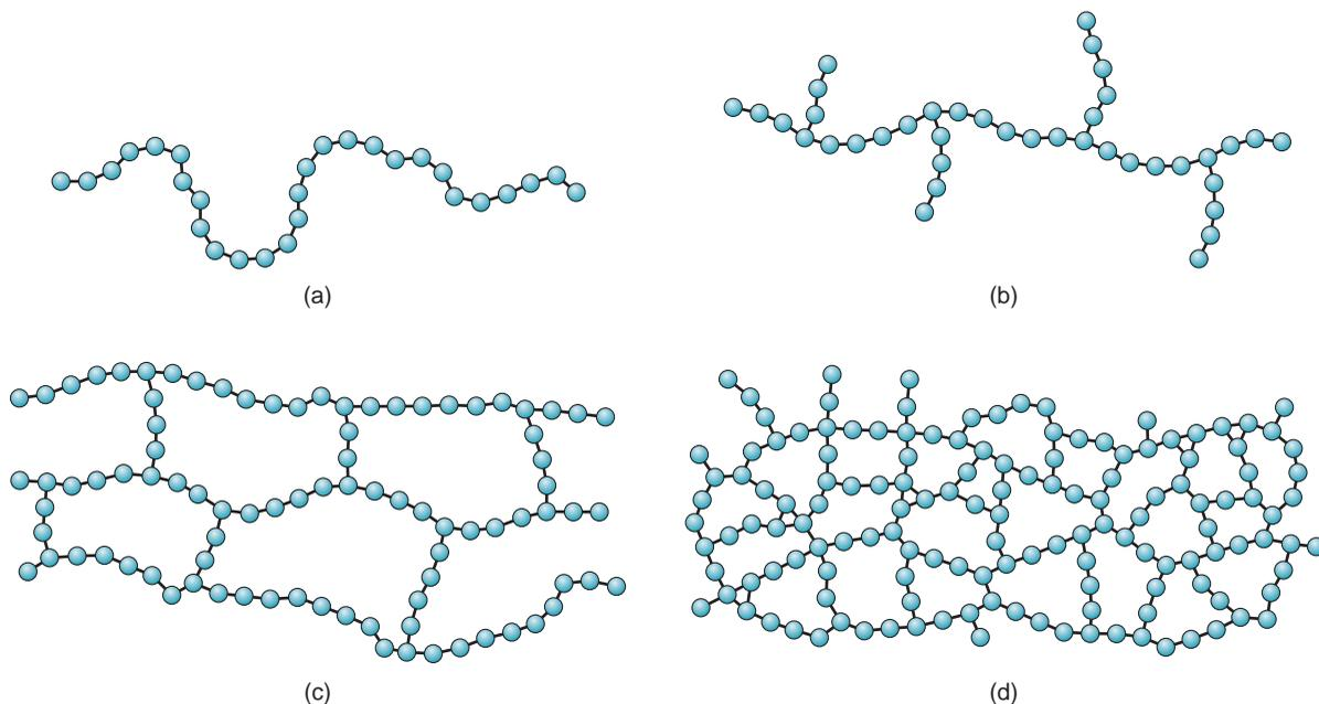
**FIGURE 8.7** Various structures of polymer molecules: (a) linear, characteristic of thermoplastics; (b) branched; (c) loosely cross-linked as in an elastomer; and (d) tightly cross-linked or networked structure as in a thermoset.
