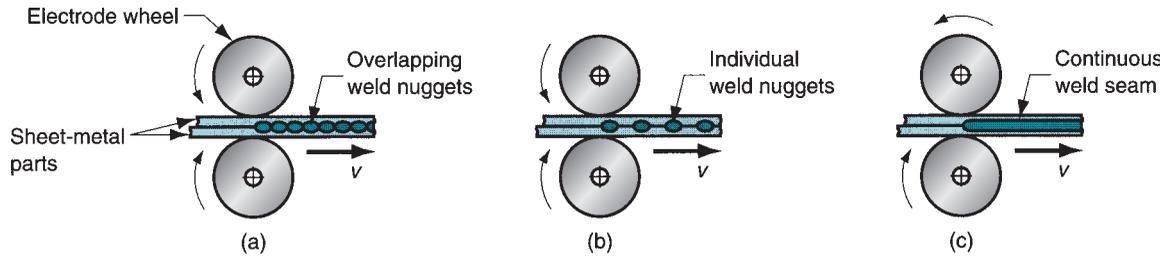
**FIGURE 30.16** Different types of seams produced by electrode wheels: (a) conventional resistance seam welding, in which overlapping spots are produced; (b) roll spot welding; and (c) continuous resistance seam.
