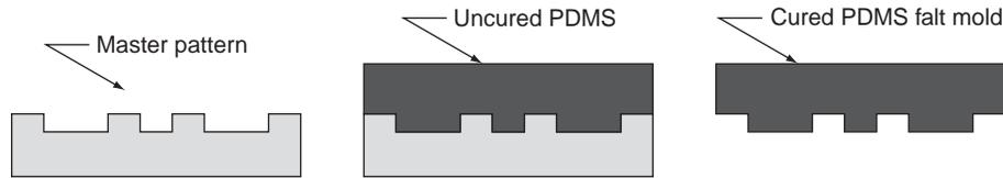
**FIGURE 36.13** Steps in mold-making for soft lithography: (1) master pattern fabricated by traditional lithography, (2) polydimethylsiloxane flat mold is cast from the master pattern, and (3) cured flat mold is peeled off pattern for use.
