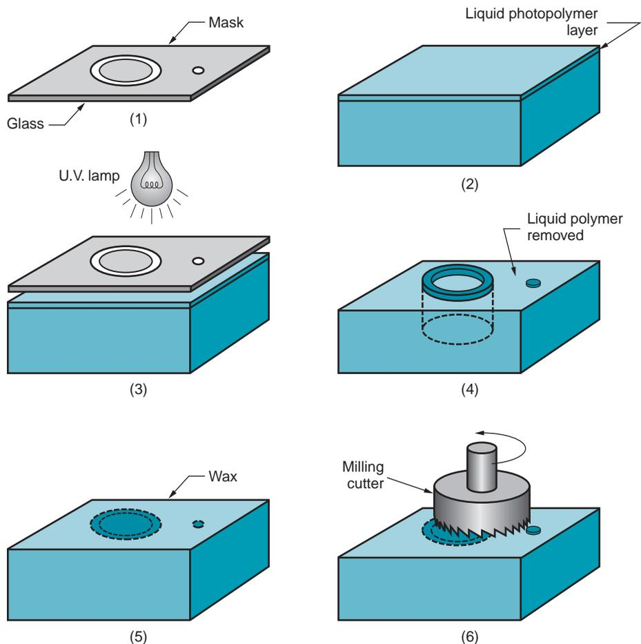
**FIGURE 33.4** Solid ground curing process for each layer: (1) mask preparation, (2) applying liquid photopolymer layer, (3) mask positioning and exposure of layer, (4) uncured polymer removed from surface, (5) wax filling, (6) milling for flatness and thickness.
