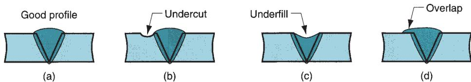
**FIGURE 30.34** (a) Desired weld profile for single V-groove weld joint. Same joint but with several weld defects: (b) **undercut**, in which a portion of the base metal part is melted away; (c) **underfill**, a depression in the weld below the level of the adjacent base metal surface; and (d) **overlap**, in which the weld metal spills beyond the joint onto the surface of the base part but no fusion occurs.
