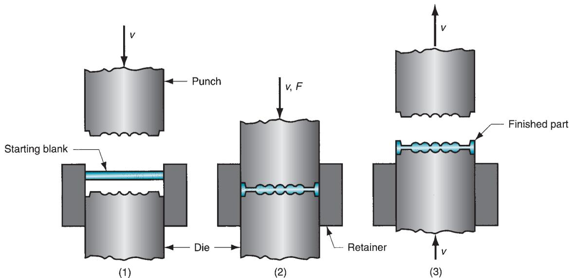
**FIGURE 19.18** Coining operation: (1) start of cycle, (2) compression stroke, and (3) ejection of finished part.
