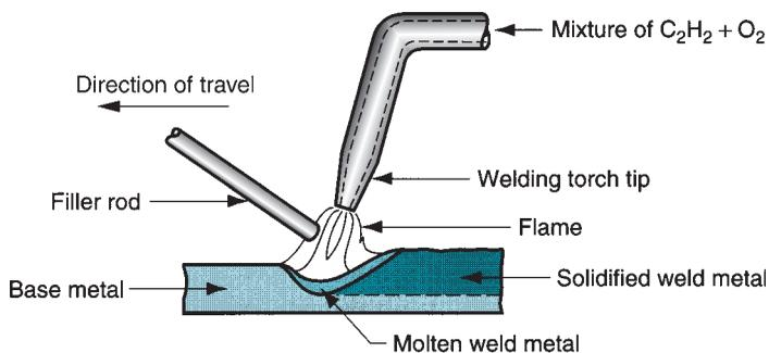
**FIGURE 30.21** A typical oxyacetylene welding operation (OAW).
