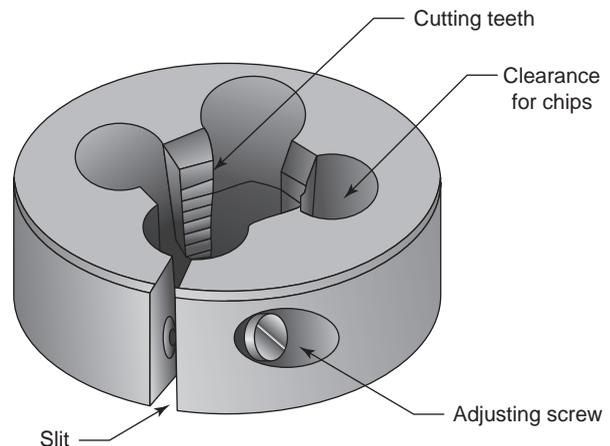
FIGURE 22.36 Threading die.
