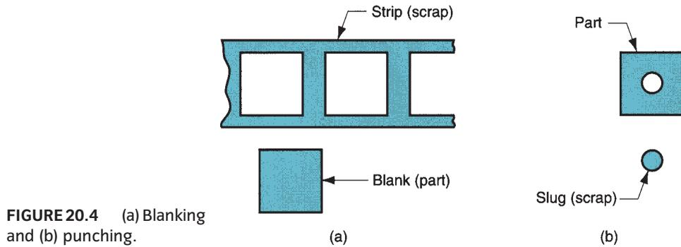
**FIGURE 20.4** (a) Blanking and (b) punching.
