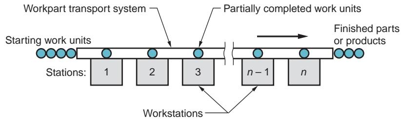
**FIGURE 39.2** General configuration of a production line.
