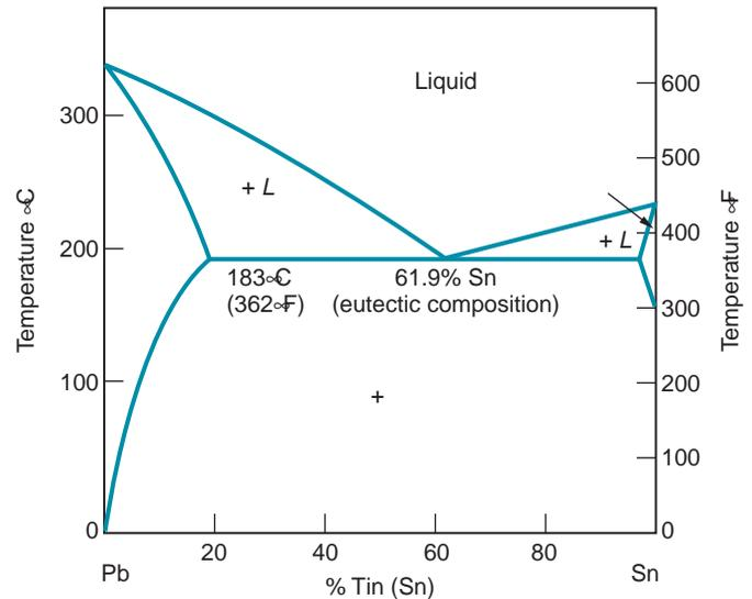
**FIGURE 6.3** Phase diagram for the tin-lead alloy system.
