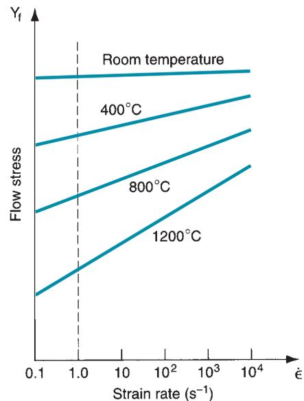
**FIGURE 18.6** Effect of temperature on flow stress for a typical metal. The constant  $C$  in Eq. (18.4), indicated by the intersection of each plot with the vertical dashed line at strain rate = 1.0, decreases, and  $m$  (slope of each plot) increases with increasing temperature.
