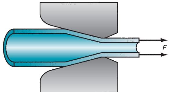
**FIGURE 19.44** Tube drawing with no mandrel (tube sinking).
