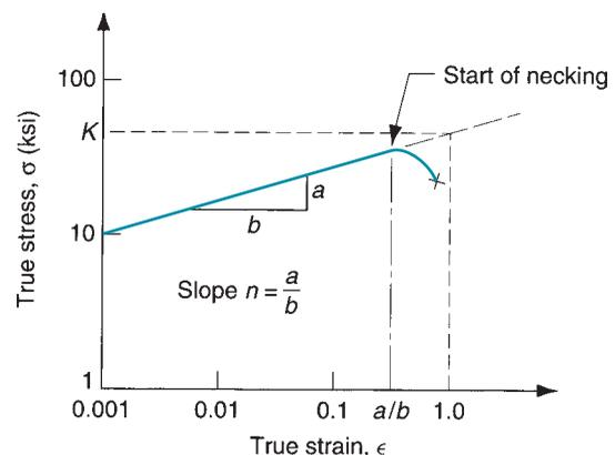
**FIGURE 3.5** True stress–strain curve plotted on log–log scale.
