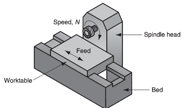
**FIGURE 22.25** Simplex bed-type milling machine horizontal spindle.
