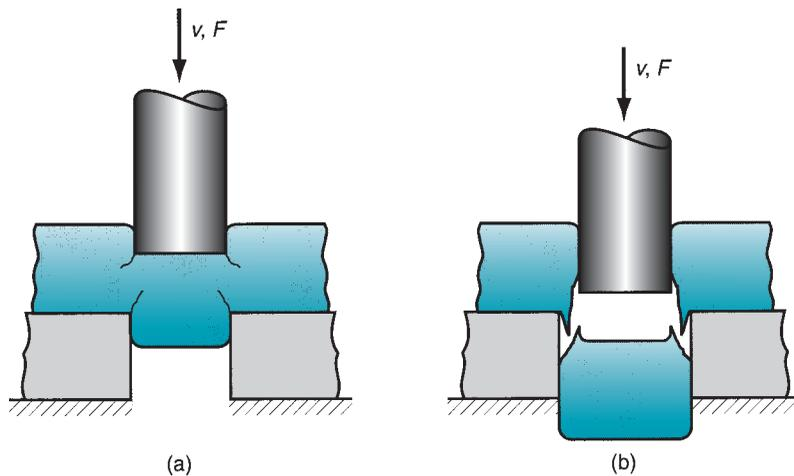
**FIGURE 20.5** Effect of clearance: (a) clearance too small causes less-than-optimal fracture and excessive forces; and (b) clearance too large causes oversized burr. Symbols  $v$  and  $F$  indicate motion and applied force, respectively.
