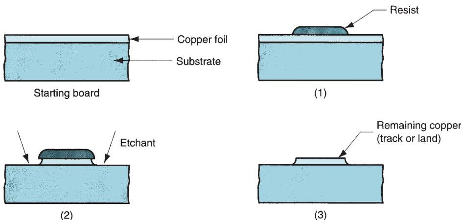
**FIGURE 35.5** The subtractive method of circuitization in PCB fabrication: (1) apply resist to areas not to be etched, using photolithography to expose the areas that are to be etched, (2) etch, and (3) strip resist.
