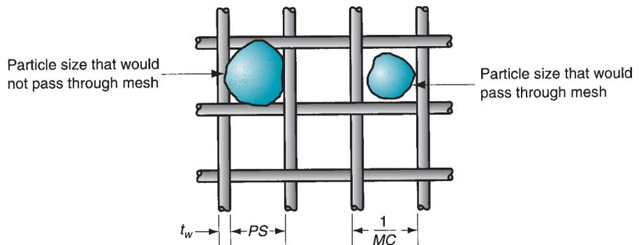
**FIGURE 16.2** Screen mesh for sorting particle sizes.
