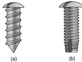
**FIGURE 32.4** Self-tapping screws: (a) thread-forming and (b) thread-cutting.
