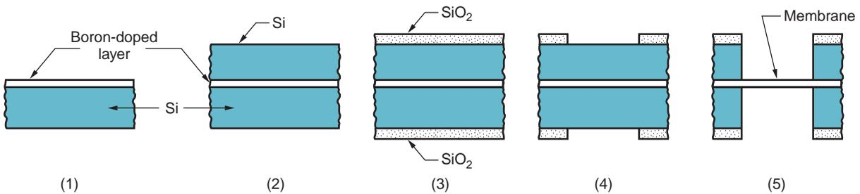
**FIGURE 36.9** Formation of a thin membrane in a silicon substrate: (1) silicon substrate is doped with boron, (2) a thick layer of silicon is applied on top of the doped layer by epitaxial deposition, (3) both sides are thermally oxidized to form a SiO<sub>2</sub> resist on the surfaces, (4) the resist is patterned by lithography, and (5) anisotropic etching is used to remove the silicon except in the boron-doped layer.
