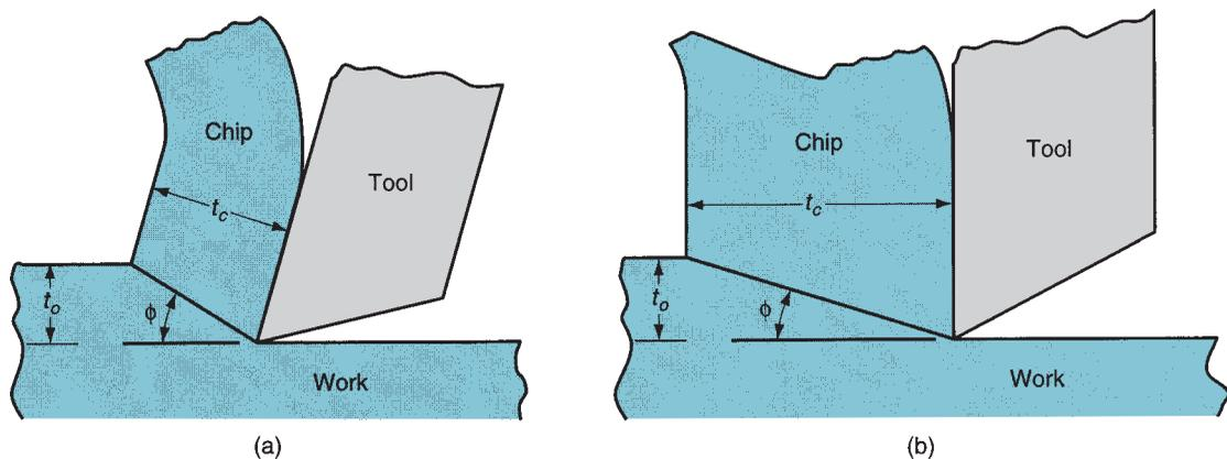
**FIGURE 21.12** Effect of shear plane angle  $\phi$ : (a) higher  $\phi$  with a resulting lower shear plane area; (b) smaller  $\phi$  with a corresponding larger shear plane area. Note that the rake angle is larger in (a), which tends to increase shear angle according to the Merchant equation.
