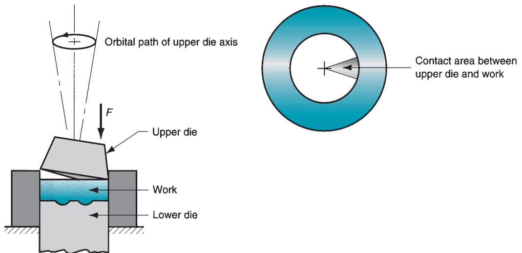
**FIGURE 19.27** Orbital forging. At end of deformation cycle, lower die lifts to eject part.
