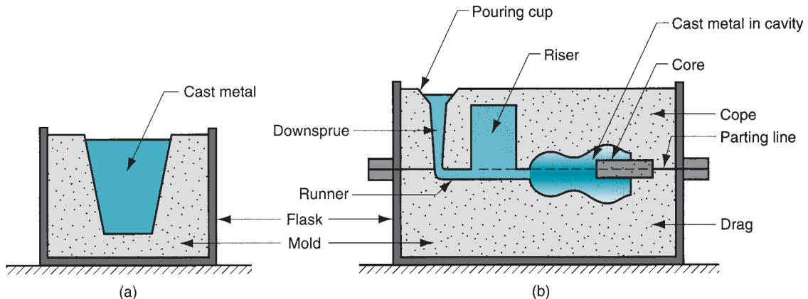
**FIGURE 10.2** Two forms of mold: (a) open mold, simply a container in the shape of the desired part; and (b) closed mold, in which the mold geometry is more complex and requires a gating system (passageway) leading into the cavity.
