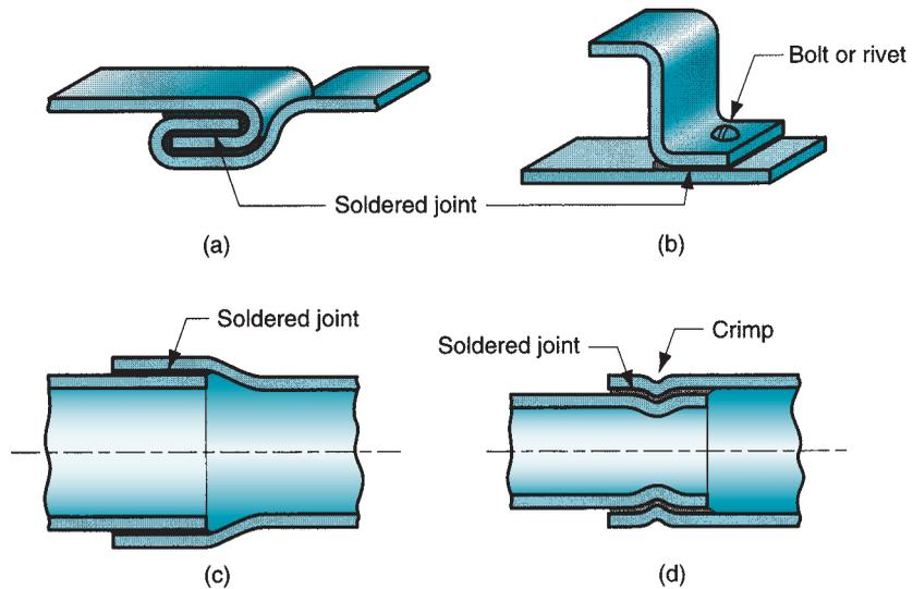
**FIGURE 31.7** Mechanical interlocking in soldered joints for increased strength: (a) flat lock seam; (b) bolted or riveted joint; (c) copper pipe fittings—lap cylindrical joint; and (d) crimping (forming) of cylindrical lap joint.
