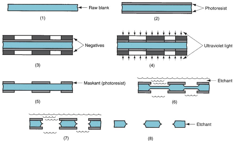
**FIGURE 26.19** Sequence of processing steps in photochemical machining: (1) clean raw part; (2) apply resist (maskant) by dipping, spraying, or painting; (3) place negative on resist; (4) expose to ultraviolet light; (5) develop to remove resist from areas to be etched; (6) etch (shown partially etched); (7) etch (completed); (8) remove resist and clean to yield finished part.
