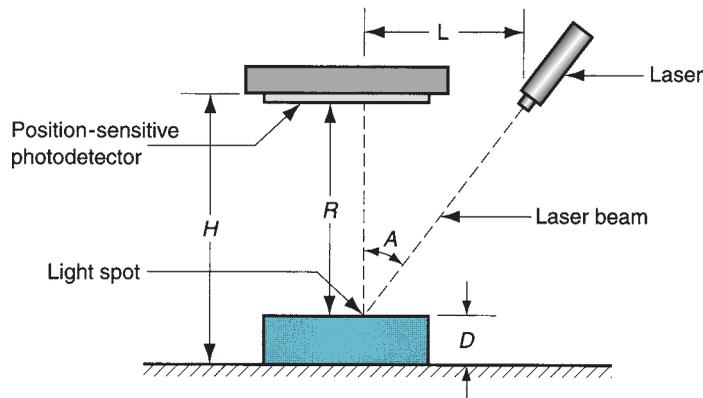
**FIGURE 42.7** Laser triangulation to measure part dimension  $D$ .
