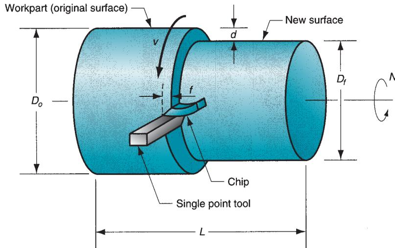
**FIGURE 22.5** Turning operation.
