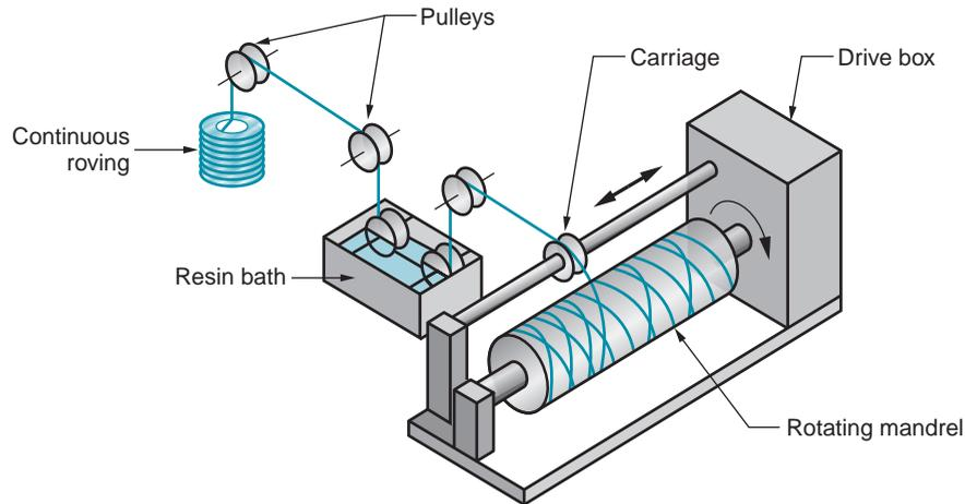
**FIGURE 15.8** Filament winding.
