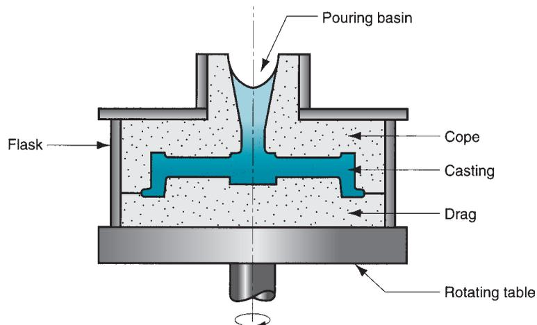
**FIGURE 11.16** Semicentrifugal casting.
