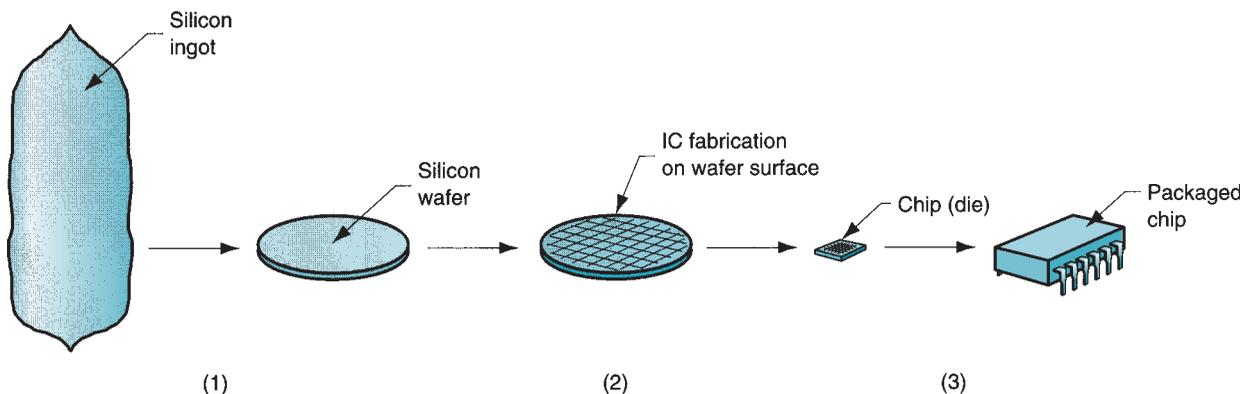
**FIGURE 34.3** Sequence of processing steps in the production of integrated circuits: (1) pure silicon is formed from the molten state into an ingot and then sliced into wafers; (2) fabrication of integrated circuits on the wafer surface; and (3) wafer is cut into chips and packaged.
