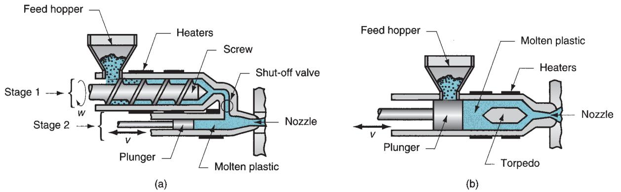
**FIGURE 13.25** Two alternative injection systems to the reciprocating screw shown in Figure 13.21: (a) screw preplasticizer, and (b) plunger type.
