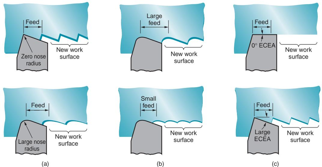
**FIGURE 24.1** Effect of geometric factors in determining the theoretical finish on a work surface for single-point tools: (a) effect of nose radius, (b) effect of feed, and (c) effect of end cutting-edge angle.
