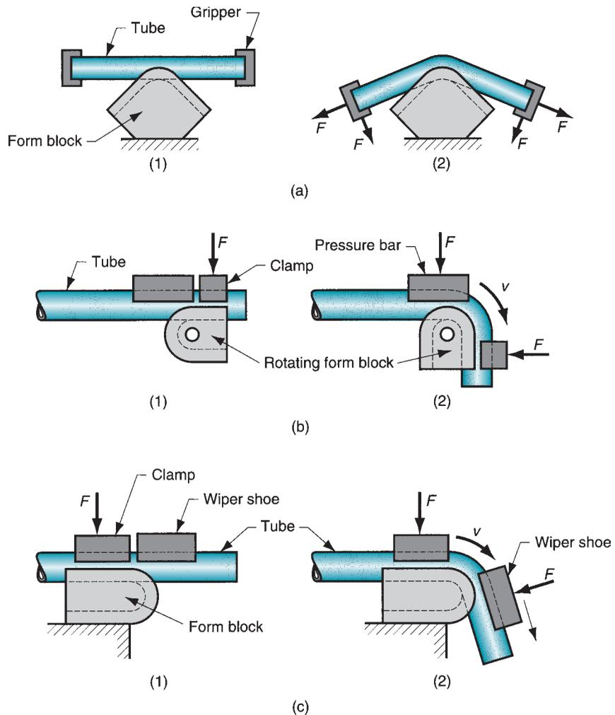
**FIGURE 20.49** Tube bending methods: (a) stretch bending, (b) draw bending, and (c) compression bending. For each method: (1) start of process, and (2) during bending. Symbols  $v$  and  $F$  indicate motion and applied force, respectively.
