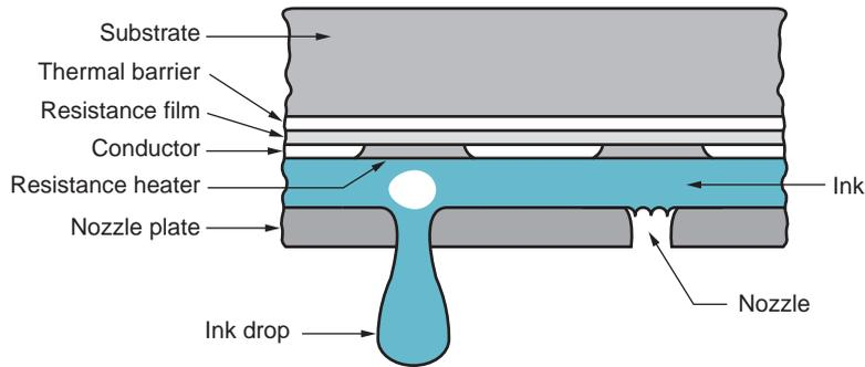
**FIGURE 36.4** Diagram of an ink-jet printing head.
