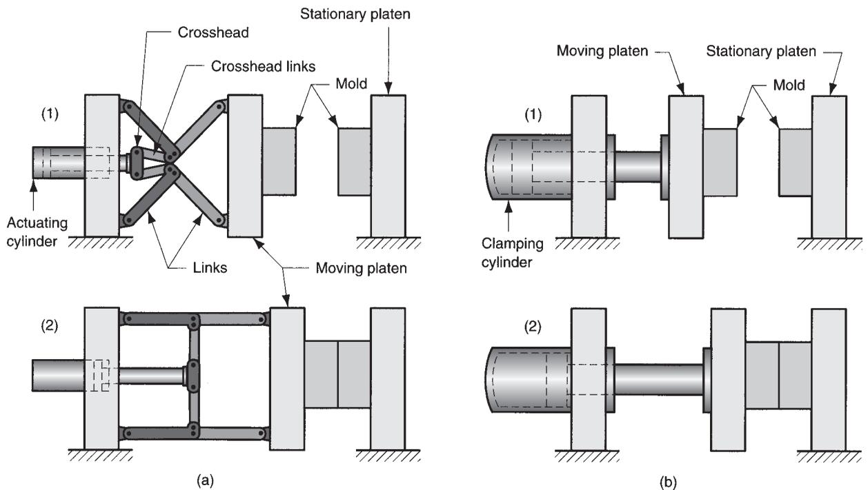
**FIGURE 13.26** Two clamping designs: (a) one possible toggle clamp design: (1) open and (2) closed; and (b) hydraulic clamping: (1) open, and (2) closed. Tie rods used to guide moving platens not shown.
