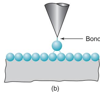
**FIGURE 37.5** Dip-pen nanolithography, in which the tip of an atomic force microscope is used to deposit molecules through the water meniscus that forms naturally between the tip and the substrate.
