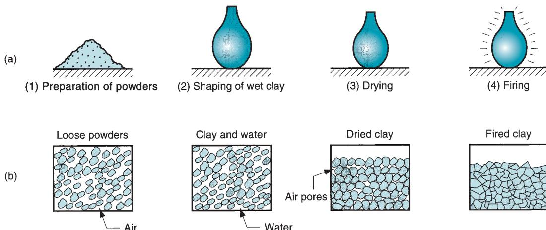
**FIGURE 17.1** Usual steps in traditional ceramics processing: (1) preparation of raw materials, (2) shaping, (3) drying, and (4) firing. Part (a) shows the workpart during the sequence, whereas (b) shows the condition of the powders.
