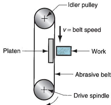
FIGURE 25.15 Abrasive belt grinding.
