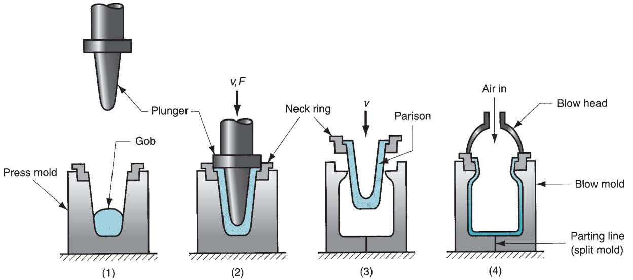
**FIGURE 12.4** Press-and-blow forming sequence: (1) molten gob is fed into mold cavity; (2) pressing to form a *parison*; (3) the partially formed parison, held in a neck ring, is transferred to the blow mold; and (4) blown into final shape. Symbols  $v$  and  $F$  indicate motion ( $v$  = velocity) and applied force, respectively.
