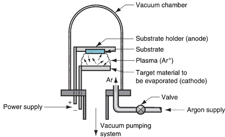
**FIGURE 28.7** One possible setup for sputtering, a form of physical vapor deposition.
