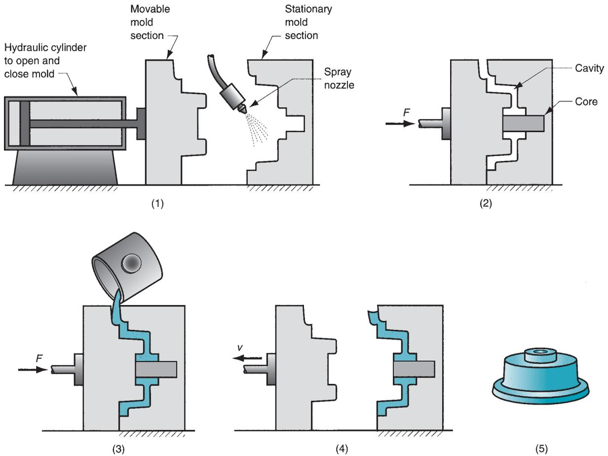
**FIGURE 11.10** Steps in permanent-mold casting: (1) mold is preheated and coated; (2) cores (if used), and mold is closed; (3) molten metal is poured into the mold; and (4) mold is opened. Finished part is shown in (5).
