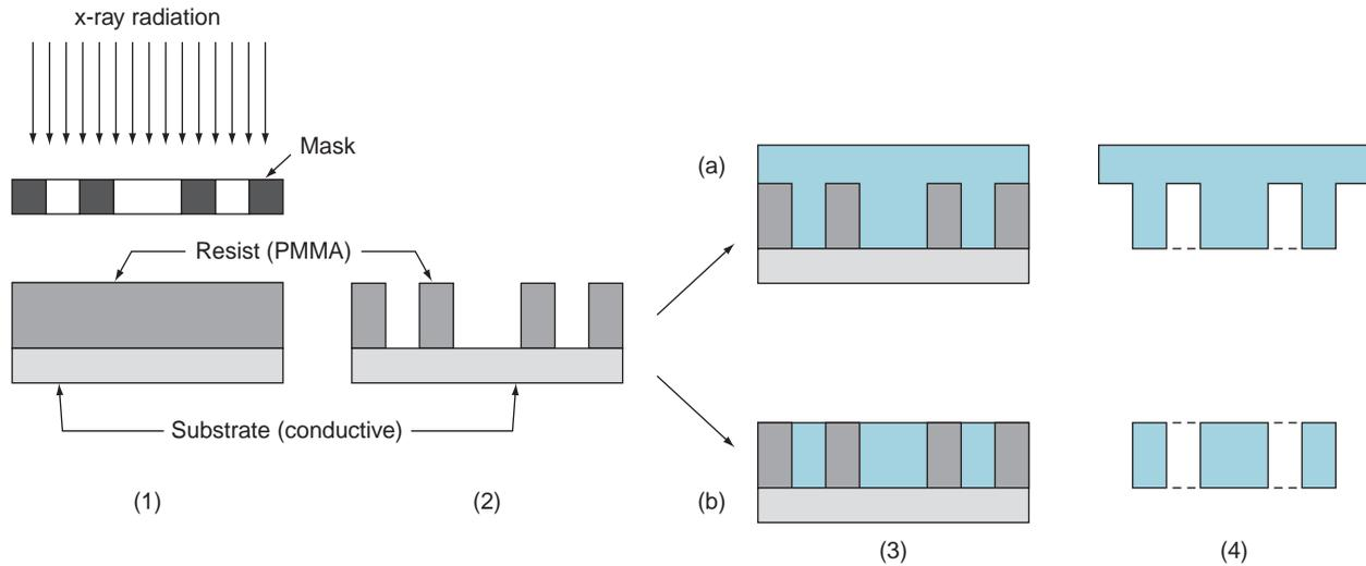
**FIGURE 36.12** LIGA processing steps: (1) thick layer of resist applied and x-ray exposure through mask, (2) exposed portions of resist removed, (3) electrodeposition to fill openings in resist, (4) resist stripped to provide (a) a mold or (b) a metal part.
