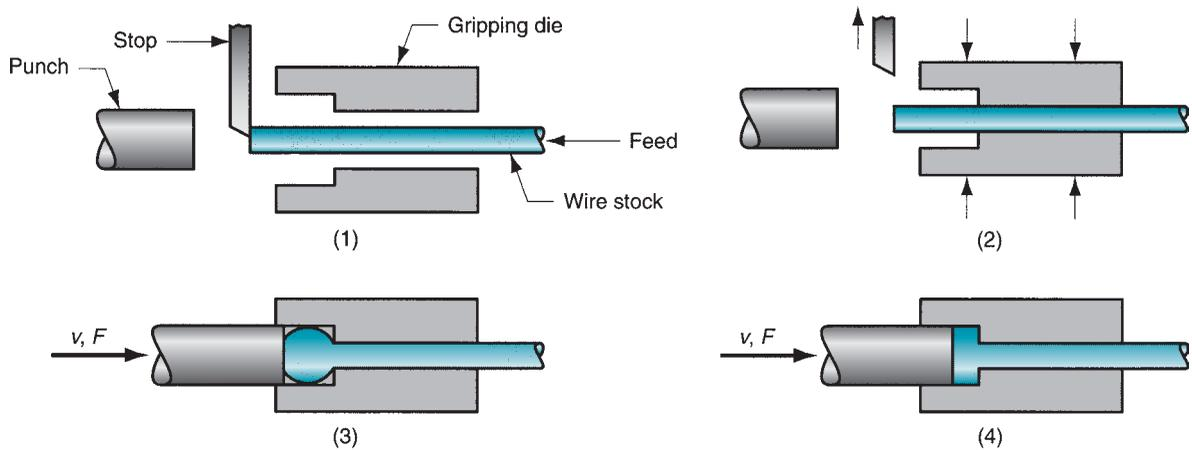
**FIGURE 19.22** An upset forging operation to form a head on a bolt or similar hardware item. The cycle is as follows: (1) wire stock is fed to the stop; (2) gripping dies close on the stock and the stop is retracted; (3) punch moves forward; and (4) bottoms to form the head.
