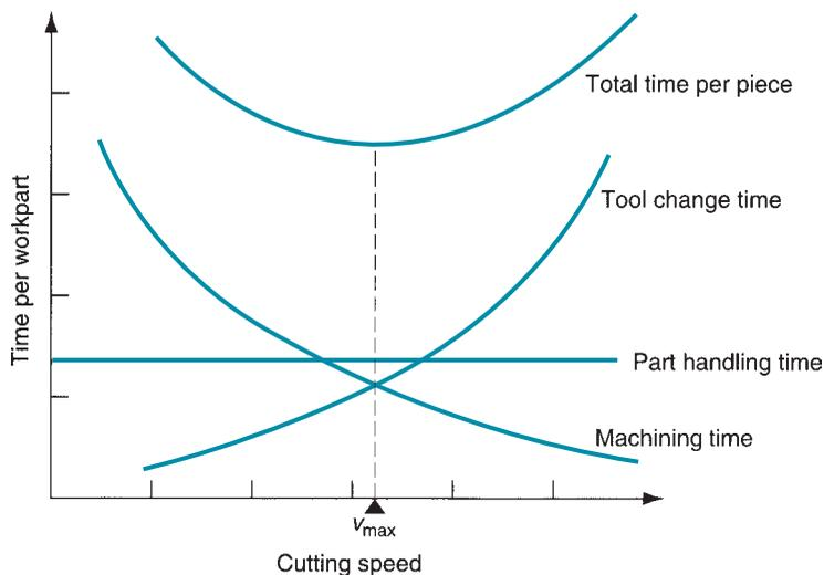
**FIGURE 24.3** Time elements in a machining cycle plotted as a function of cutting speed. Total cycle time per piece is minimized at a certain value of cutting speed. This is the speed for maximum production rate.
