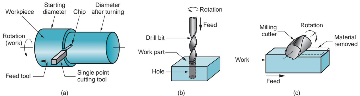
**FIGURE 1.8** Common machining operations: (a) **turning**, in which a single-point cutting tool removes metal from a rotating workpiece to reduce its diameter; (b) **drilling**, in which a rotating drill bit is fed into the work to create a round hole; and (c) **milling**, in which a workpart is fed past a rotating cutter with multiple edges.
