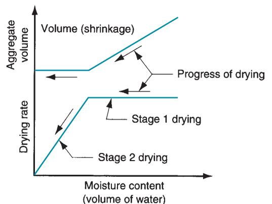
**FIGURE 17.9** Typical drying rate curve and associated volume reduction (drying shrinkage) for a ceramic body in drying. Drying rate in the second stage of drying is depicted here as a straight line (constant rate decrease as a function of water content); the function is variously shown as concave or convex in the literature [3], [8].
