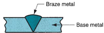
conventional weld joint, such as the V-joint shown. A greater quantity of filler metal is deposited than in brazing, and no capillary action occurs. In braze welding, the joint consists entirely of filler metal; the base metal does not melt and is therefore not fused into the joint as in a conventional fusion welding process. The principal application of braze welding is repair work.
