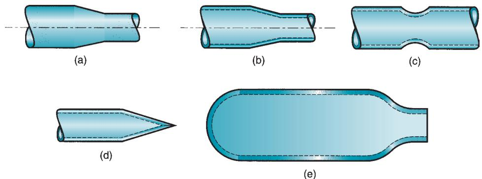
**FIGURE 19.25** Examples of parts made by swaging: (a) reduction of solid stock, (b) tapering a tube, (c) swaging to form a groove on a tube, (d) pointing a tube, and (e) swaging of neck on a gas cylinder.
