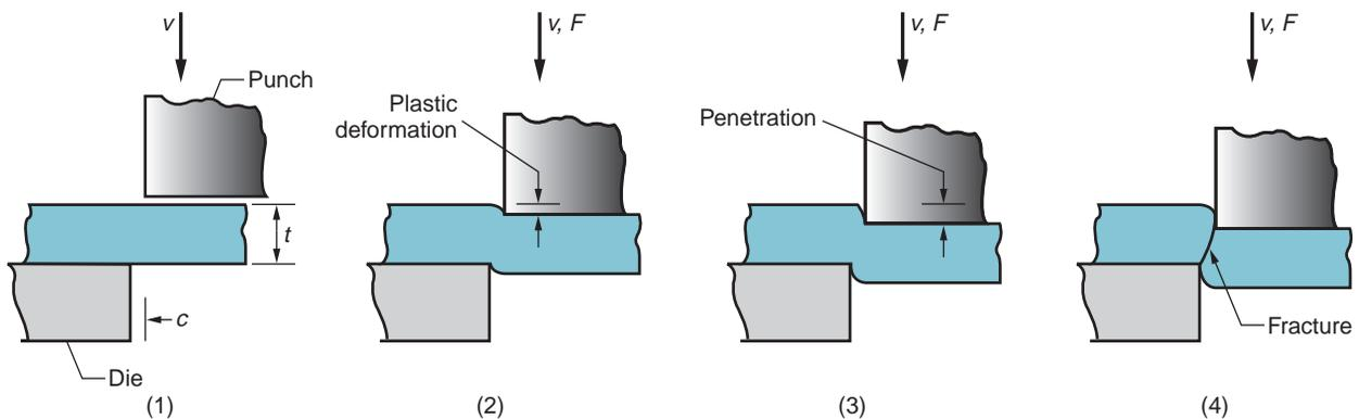
**FIGURE 20.1** Shearing of sheet metal between two cutting edges: (1) just before the punch contacts work; (2) punch begins to push into work, causing plastic deformation; (3) punch compresses and penetrates into work causing a smooth cut surface; and (4) fracture is initiated at the opposing cutting edges that separate the sheet. Symbols  $v$  and  $F$  indicate motion and applied force, respectively,  $t$  = stock thickness,  $c$  = clearance.
