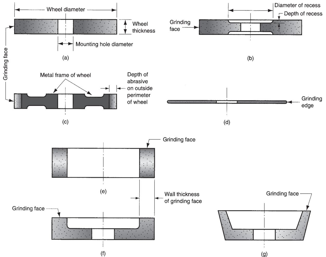
**FIGURE 25.2** Some of the standard grinding wheel shapes: (a) straight, (b) recessed two sides, (c) metal wheel frame with abrasive bonded to outside circumference, (d) abrasive cutoff wheel, (e) cylinder wheel, (f) straight cup wheel, and (g) flaring cup wheel.
