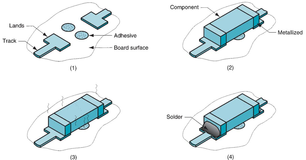
**FIGURE 35.11** Adhesive bonding and wave soldering, shown here for a discrete capacitor or resistor component: (1) adhesive is applied to areas on the board where components are to be placed; (2) components are placed onto adhesive-coated areas; (3) adhesive is cured; and (4) solder joints are made by wave soldering.
