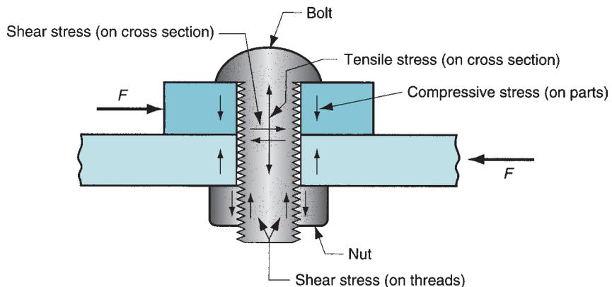
**FIGURE 32.9** Typical stresses acting on a bolted joint.
