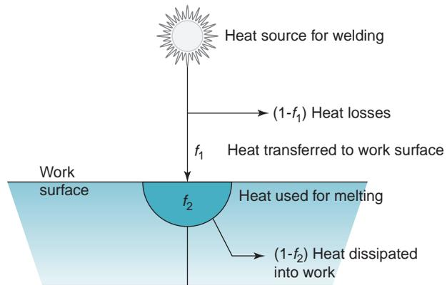
**FIGURE 29.8** Heat transfer mechanisms in fusion welding.
