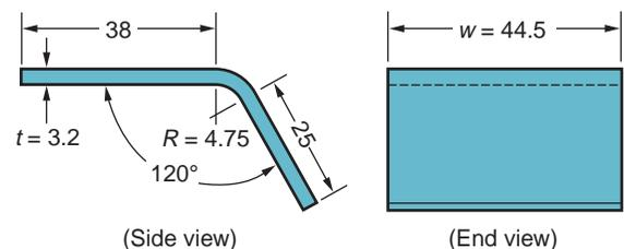
**FIGURE 20.15** Sheet-metal part of Example 20.2.2 (dimensions in mm).
