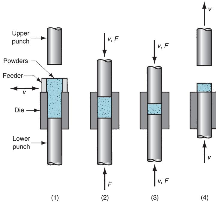
**FIGURE 16.9** Pressing, the conventional method of compacting metal powders in PM: (1) filling the die cavity with powder, done by automatic feed in production, (2) initial, and (3) final positions of upper and lower punches during compaction, and (4) ejection of part.
