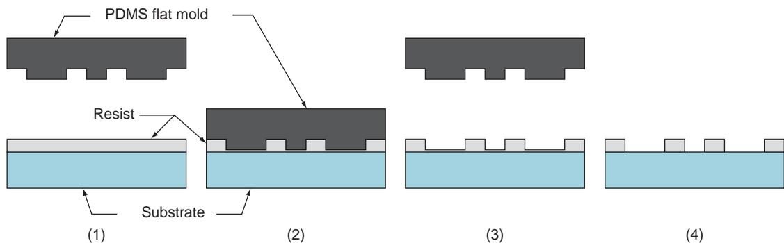
**FIGURE 36.14** Steps in micro-imprint lithography: (1) mold positioned above and (2) pressed into resist, (3) mold is lifted, and (4) remaining resist is removed from substrate surface in defined regions.
