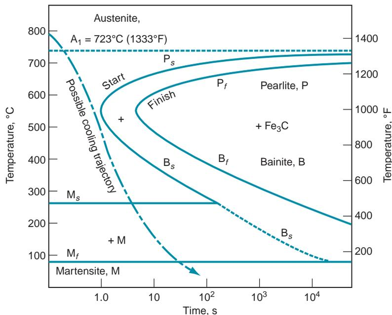
**FIGURE 27.1** The TTT curve, showing the transformation of austenite into other phases as a function of time and temperature for a composition of about 0.80% C steel. The cooling trajectory shown here yields martensite.
