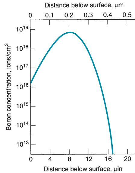
**FIGURE 28.4** Profile of surface chemistry as treated by ion implantation. (Source: [17].) Shown here is a typical plot for boron implanted in silicon. Note the difference in profile shape and depth of altered layer compared to diffusion in Figure 28.3.
