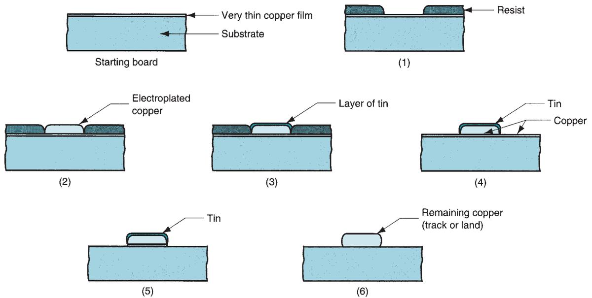
**FIGURE 35.7** The semiadditive method of circuitization in PCB fabrication: (1) Apply resist to areas that will not be plated; (2) electroplate copper, using the thin copper film for conduction; (3) apply tin on top of plated copper; (4) strip resist; (5) etch remaining thin film of copper on the surface, while the tin serves as a resist for the electroplated copper; and (6) strip tin from copper.
