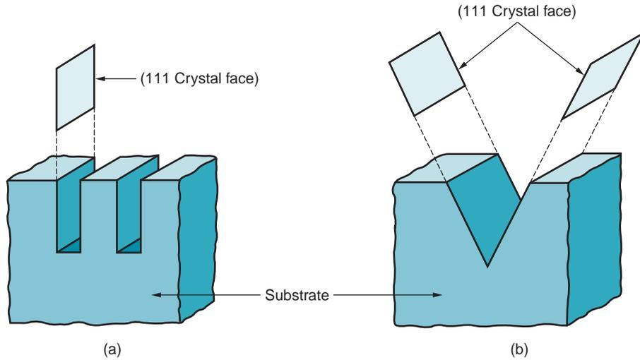
**FIGURE 36.8** Several structures that can be formed in single-crystal silicon substrate by bulk micromachining: (a) (110) silicon and (b) (100) silicon.
