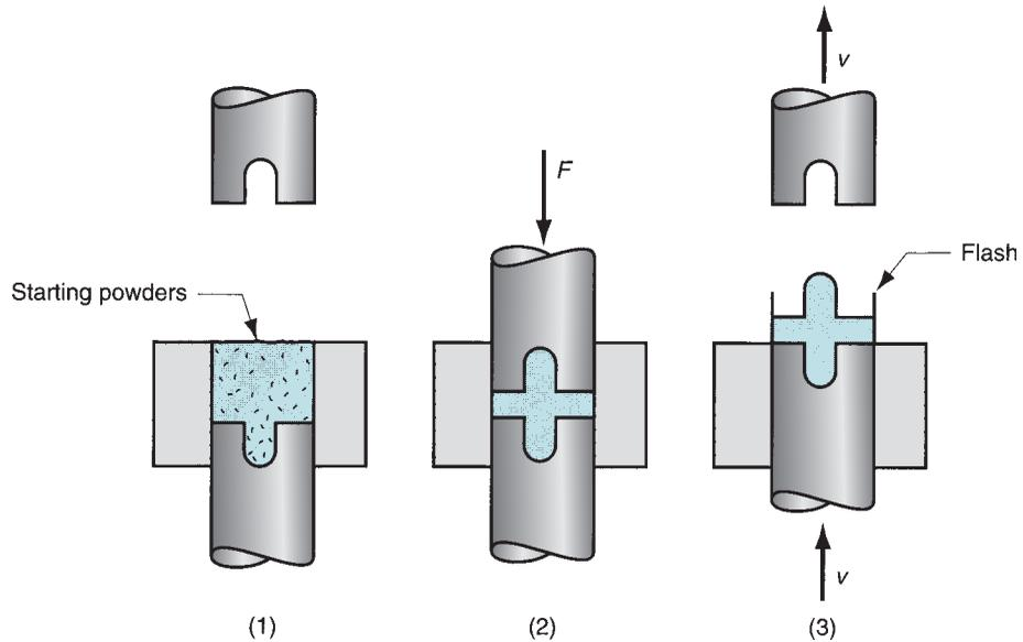
**FIGURE 17.7** Semi-dry pressing: (1) depositing moist powder into die cavity, (2) pressing, and (3) opening the die sections and ejection. Symbols  $v$  and  $F$  indicate motion ( $v$  = velocity) and applied force, respectively.
