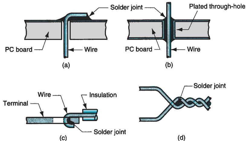
**FIGURE 31.8** Techniques for securing the joint by mechanical means prior to soldering in electrical connections: (a) crimped lead wire on printed circuit board (PCB); (b) plated through hole on PCB to maximize solder contact surface; (c) hooked wire on flat terminal; and (d) twisted wires.
