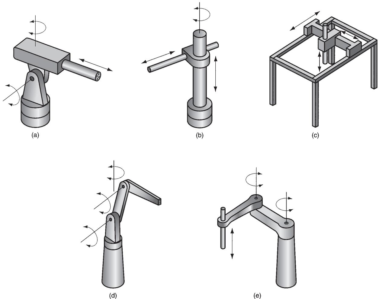
**FIGURE 38.14** Five common anatomies of commercial industrial robots: (a) polar, (b) cylindrical, (c) Cartesian coordinate, (d) jointed-arm, and (e) SCARA, or selectively compliant assembly robot arm.
