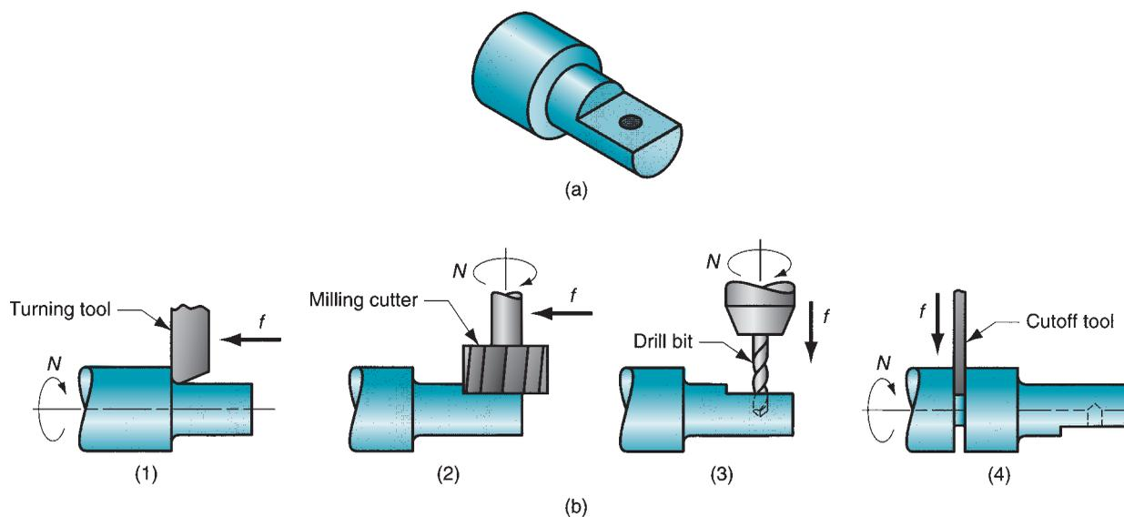
**FIGURE 22.28** Operation of a mill-turn center: (a) example part with turned, milled, and drilled surfaces; and (b) sequence of operations on a mill-turn center: (1) turn second diameter, (2) mill flat with part in programmed angular position, (3) drill hole with part in same programmed position, and (4) cutoff.
