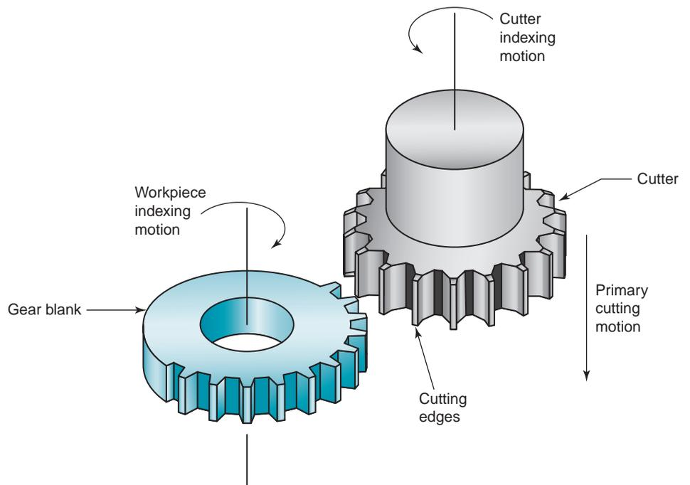
**FIGURE 22.41** Gear shaping.
