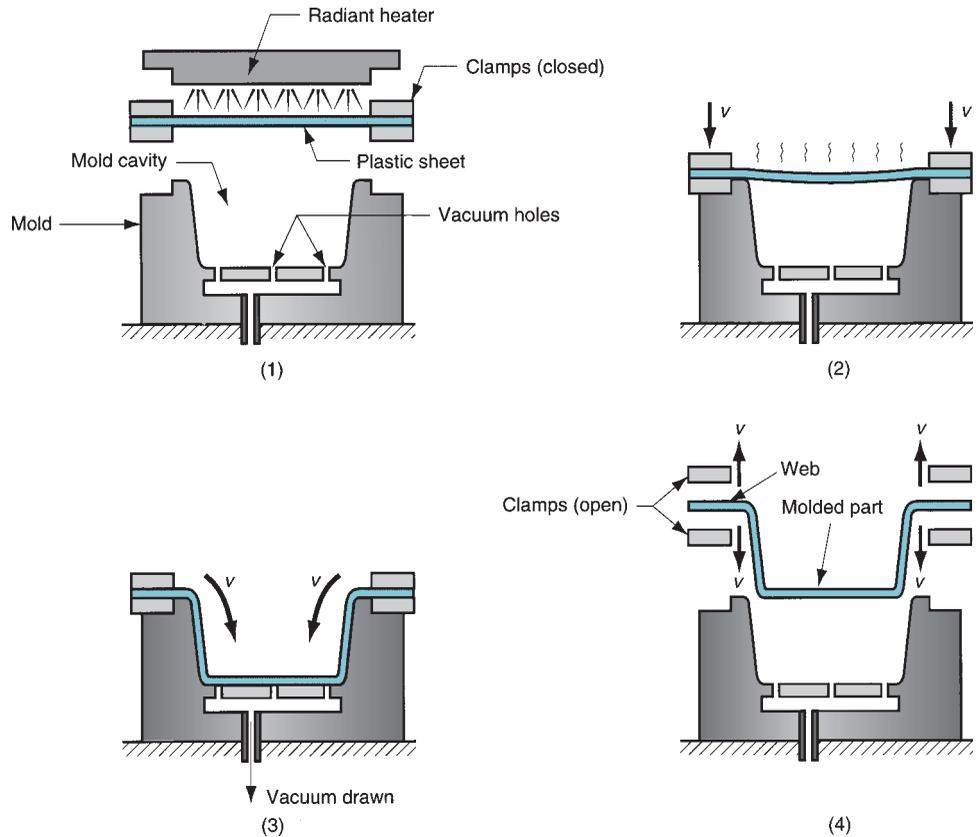
**FIGURE 13.35** Vacuum thermoforming: (1) a flat plastic sheet is softened by heating; (2) the softened sheet is placed over a concave mold cavity; (3) a vacuum draws the sheet into the cavity; and (4) the plastic hardens on contact with the cold mold surface, and the part is removed and subsequently trimmed from the web.
