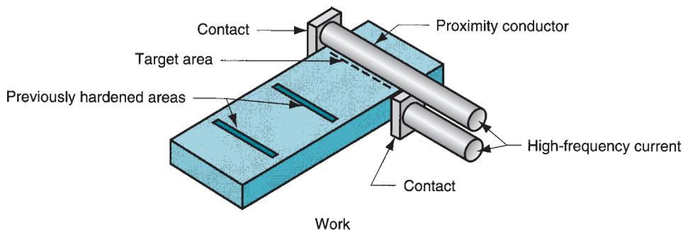
**FIGURE 27.8** Typical setup for high-frequency resistance heating.
