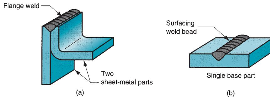
**FIGURE 29.7** (a) Flange weld; and (b) surfacing weld.
